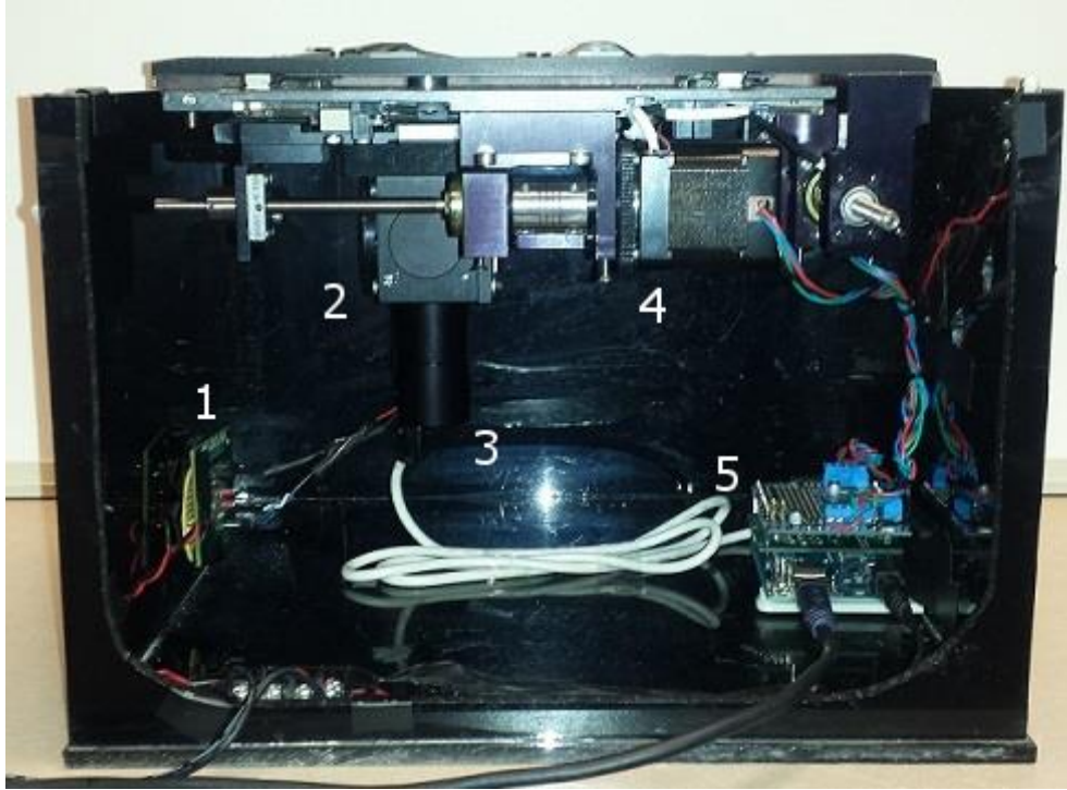
Figure 4.2A: Close-up view of the portable system. 1. LED current driver board. 2. Optical mounting containing dichroic mirror, LED, objective lens, and optical filter. 3. Photodiode and preamplifier board. 4. Positioning motors, seen here from the side. 5. Arduino microcontroller with stacked motor driver shield and amplifier and analog to digital converter shield connected to preamplifier via white USB cable. The system itself measures 12" wide x 11" deep x 8" tall and weighs approximately 10 lbs.
