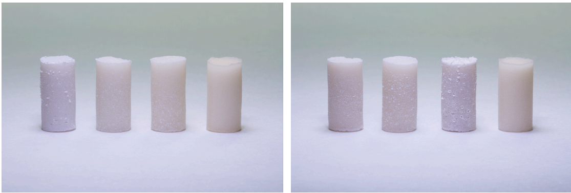
Figure 3-1: Left: From left to right, a 30% 5 \mu\text{m} pellet, a 30% 33 \mu\text{m} pellet, a 30% 100 \mu\text{m} pellet, and a control pellet. The samples were soaked for 7 days and were dried in an oven at 90°C for one day. Right: From left to right, a 20% 33 \mu\text{m} pellet, a 30% 33 \mu\text{m} pellet, a 40% 33 \mu\text{m} pellet, and a control pellet. The samples were soaked for 21 days and dried in an oven at 90°C for one day.
