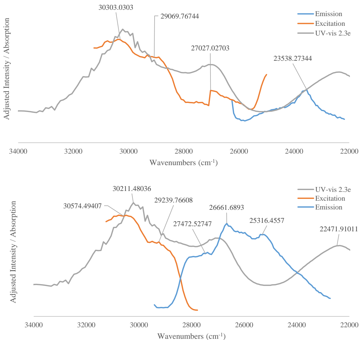
Figure 4.2d: superimposed UV-vis and fluorescence spectra of 2.3e.
