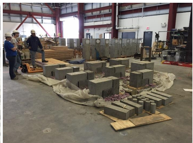
(f) Push-off Specimens after Demolding
