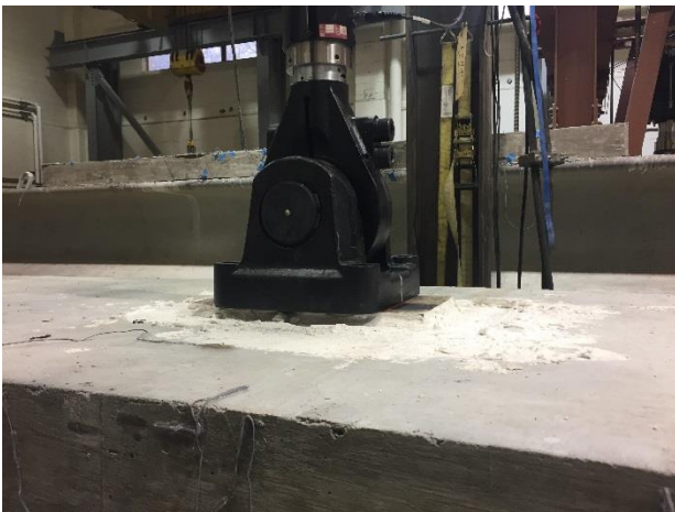
(c) Bearing of Actuator on Bridge Deck
