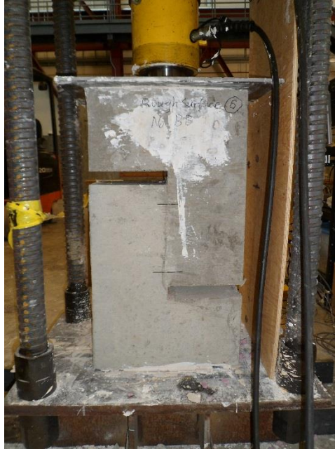
Figure 2.1: Typical Push-off Specimen
