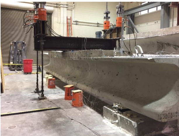
(c) Large Deformation at End of Test
