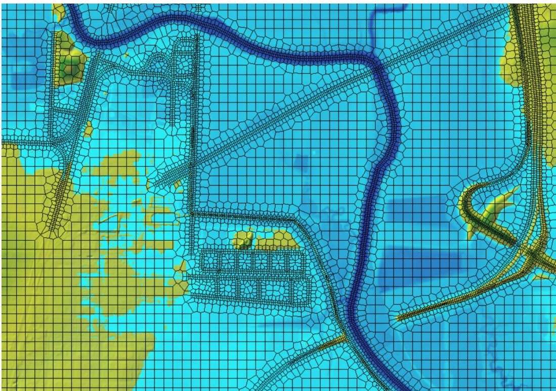
Figure 3-9: 4.8K cms flood at the Coffeyville Refinery along the Verdigris River.
