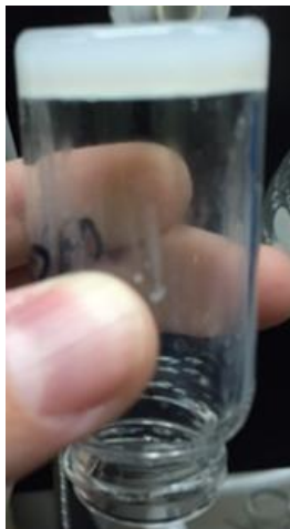
Figure 7. Inverted vial containing gel formed from 3.2 in DMSO.
