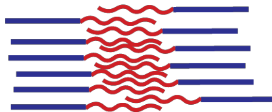
Figure 4. Lamellar alignment of rod-coil BCP leading to microphase segregation.
