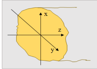
Figure 3.2: Regions showing the boundary condition in rough surface TSV conductor
