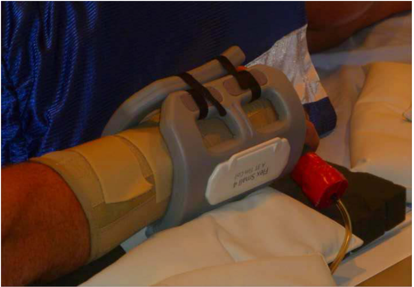
Figure 2. Example wrist of a subject with the grip device in the active grasp position. The wrist was also braced for consistent loaded positions.
