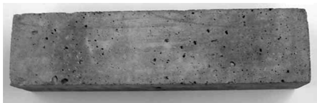
Fig. 5—Specimen subjected to 95 weeks of exposure to 1.06 molal ion concentration solution of CaCl 2 .
