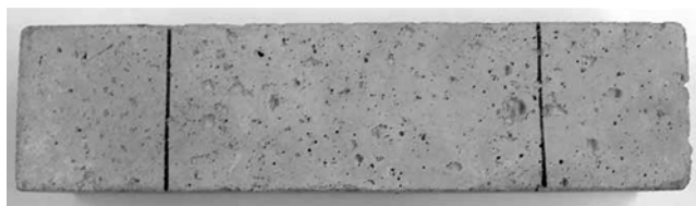
Fig. 3—Specimen subjected to 95 weeks of exposure to distilled water.
