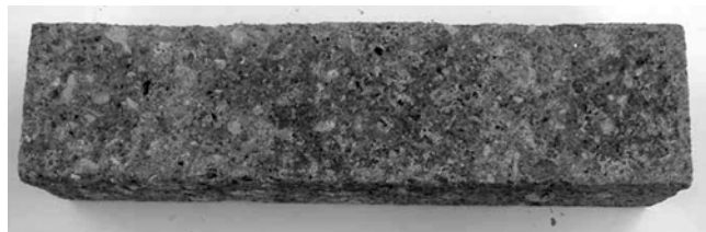
Fig. 8—Specimen subjected to 95 weeks of exposure to 6.04 molal ion concentration solution of NaCl.
