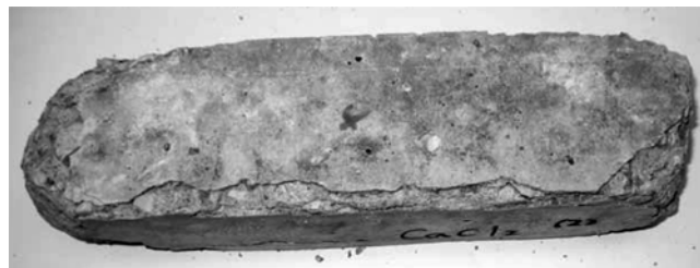
Fig. 9—Specimen subjected to 10 weeks of exposure to 6.04 molal ion concentration solution of CaCl 2 .
