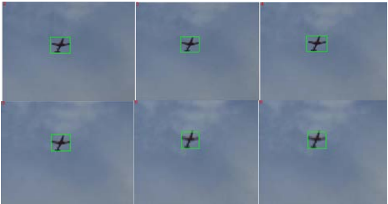
Fig 1.1: Object detection & tracking application of locating a flying object from airplane_001 dataset [42]
