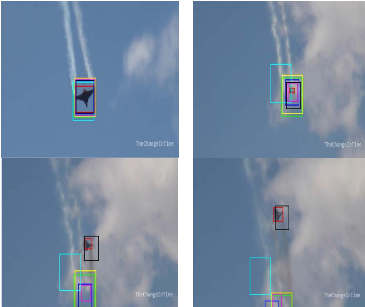
Fig 6.7: Tracking result with bounding box around the objects in airplane_005 dataset for all the 7 trackers exhibiting partial occlusion. Color code same as Precision and Success Plots
