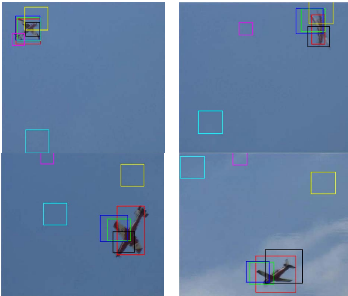
Fig 6.10: Tracking result with bounding boxes around the objects in Aircraft dataset for all the 7 trackers exhibiting in-plane rotation. Color code same as Precision and Success Plots
