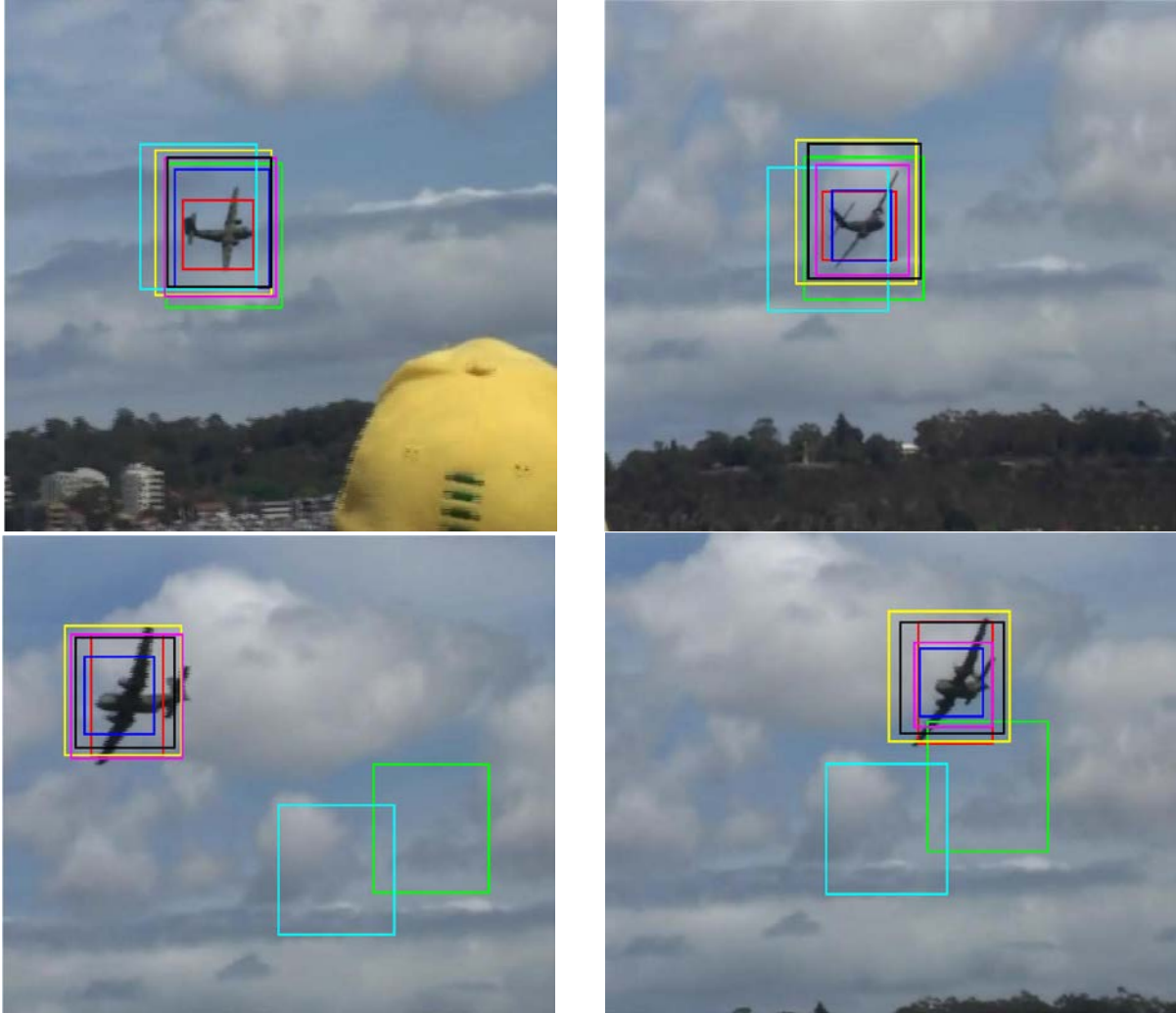
Fig 6.11: Tracking result with bounding boxes around the objects in big_2 dataset for all the 7 trackers exhibiting out-of-plane rotation. Color code same as Precision and Success Plots
