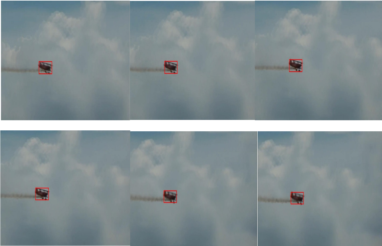
Fig A.9: Snapshots from airplane_013 dataset showing tracking with the proposed tracker
