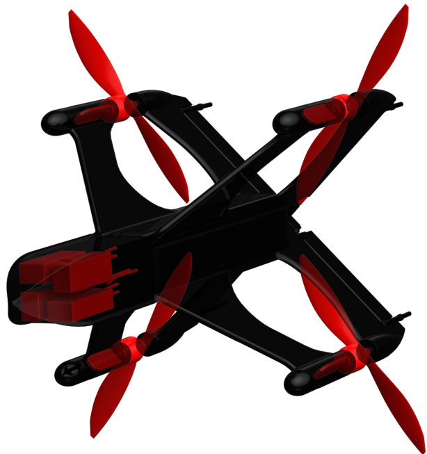
Fig. 3.5: XQ-139B propulsion system.
