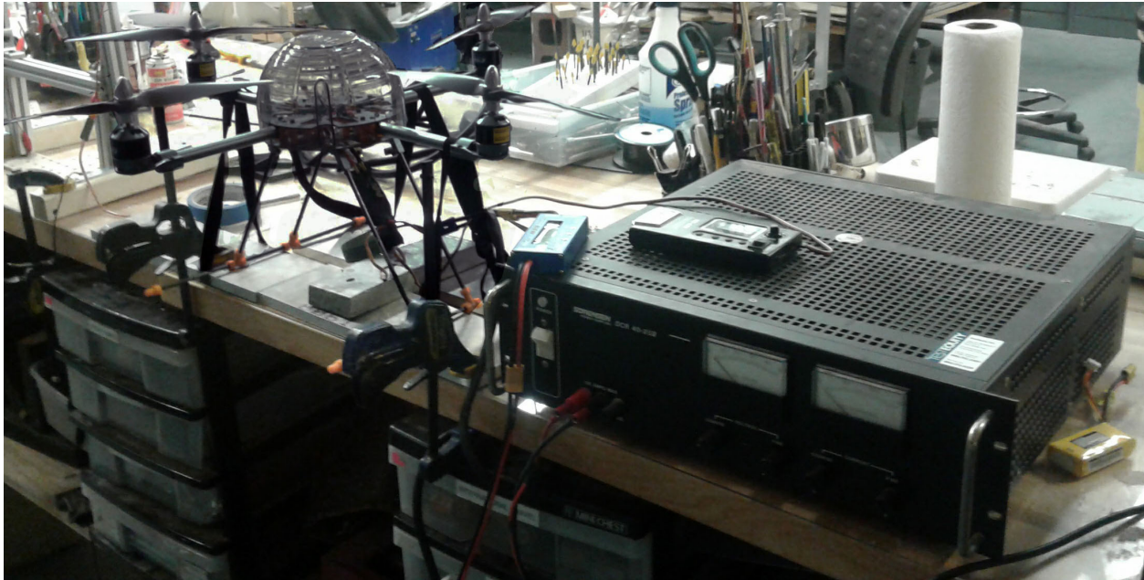
Fig. 4.2: H.A.L. frame constrained for efficiency testing.
