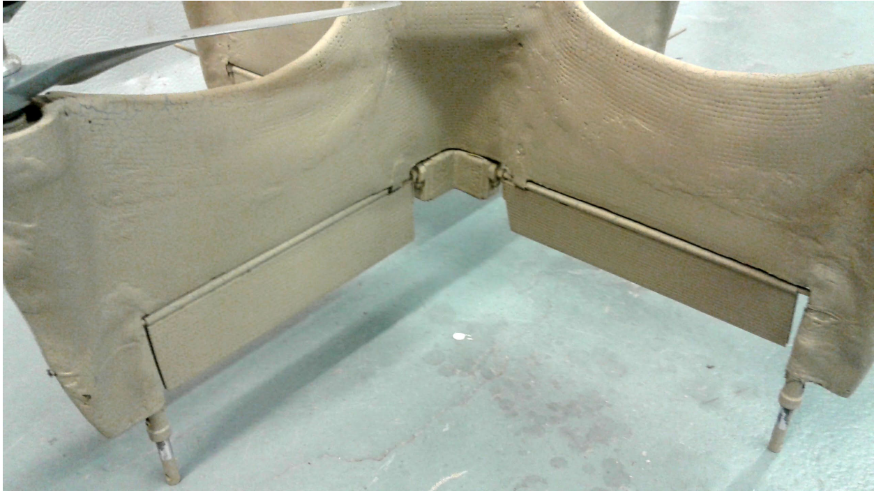
Fig. 3.11: Servos installed for control surface actuation.
