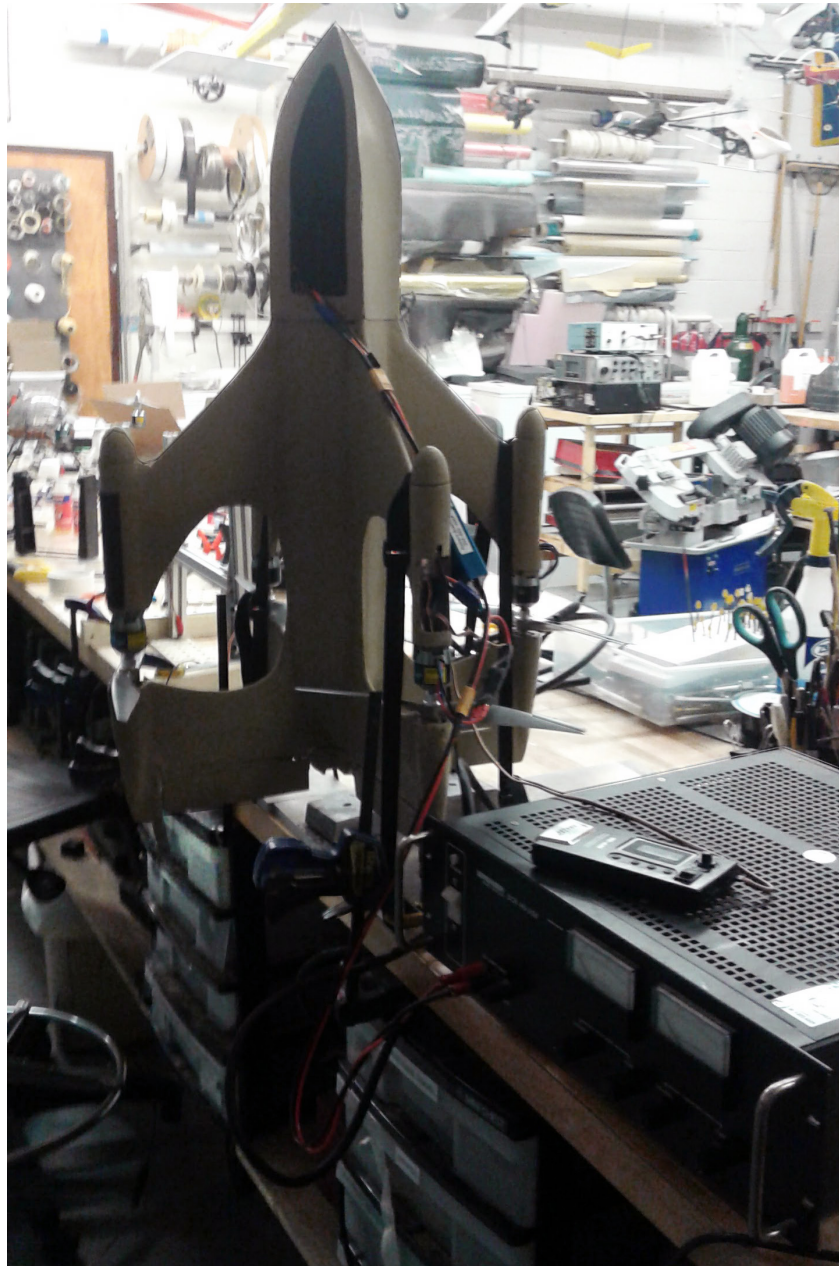
Fig. 4.5: XQ-139B constrained for efficiency testing.
