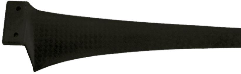
Fig. 1.41: Multi-rotor blade manufactured with near-ideal taper and twist. (63)
