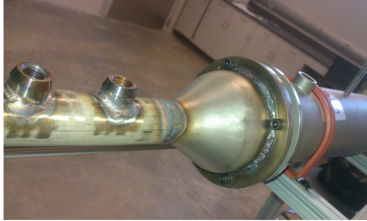
Figure 54: Connection between HX and engine exhaust showing sensor ports, concentric reducer, and flange
