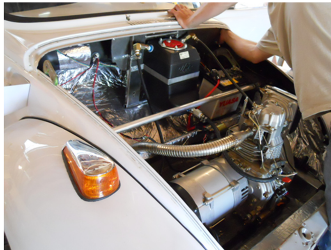
Figure 61: View of EcoHawks beetle trunk showing space near firewall away from the engine-generator
