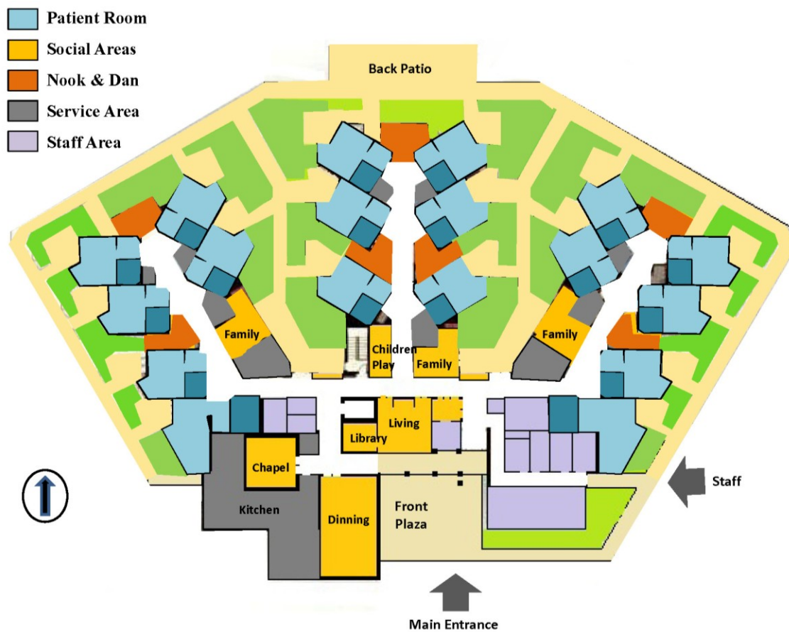
Figure 6-16. The building layout of Case-3. It shows the south side main entrance, three pods or wings. Each pod has six patients room, two nooks, one den. This figure is produced by Sharmin Kader from the building layout with permission.
