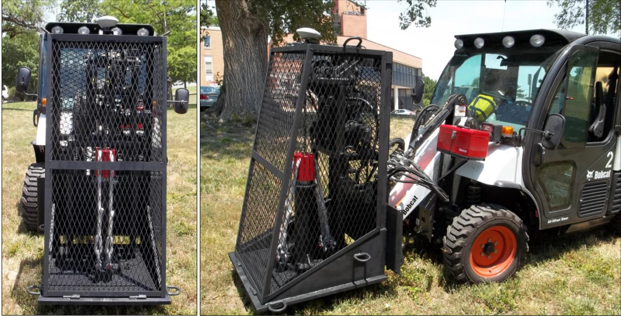
Figure 27: bungee assisted accelerated weight drop (Photos from the Kansas Geological Survey)
