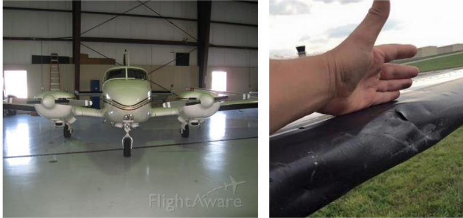
Figure 2: Damaged wing of a Piper Apache GA aircraft after colliding with a UAS at 2,500-ft AGL at Lewis University, Illinois in Aug, 2015 [ref 1].
