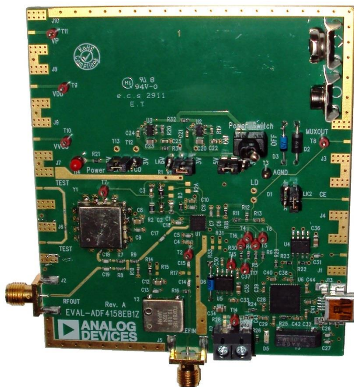
Figure 19: Analog Device ADF4158 FMCW waveform synthesizer evaluation board. Modifications were made to the VCO and snubber filter to produce a 15-MHz chirp centered at 1.445 GHz.
