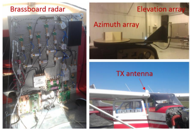
Figure 38: Brassboard radar system installation onboard the Cessna 172. (left) Brassboard radar system mounted vertically in the back of the Cessna 172 just behind the rear seat. (top right) RX azimuth and elevation antennas mounted inside the aircraft. (bottom right) TX antenna mounted to the roof.
