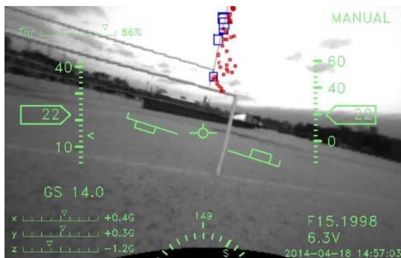
Figure 4: MIT's Drone collision avoidance camera technology uses two cameras and two separate GPU processors to constant detect targets located specifically at 10m in front of the aircraft to provide real time collision avoidance capability [ref 3].
