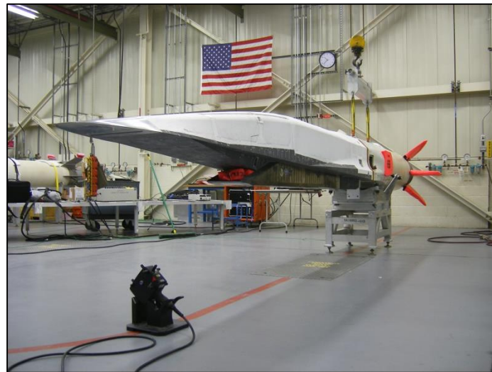
Figure 3: X-51A Hypersonic vehicle being prepared for first flight. Image courtesy of Air Force Flight Test Center Public Affairs[6]
