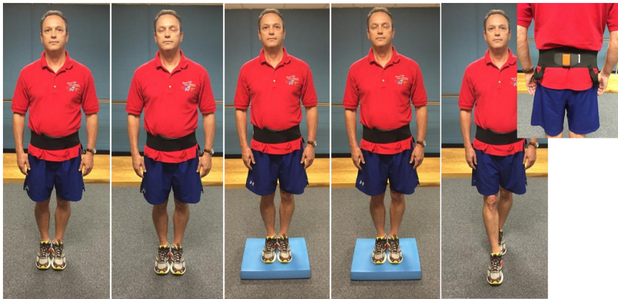
Figure 1: The five experimental conditions used to examine postural sway. The inertial sensor was positioned at L3 spine level, displayed in the inset picture.
