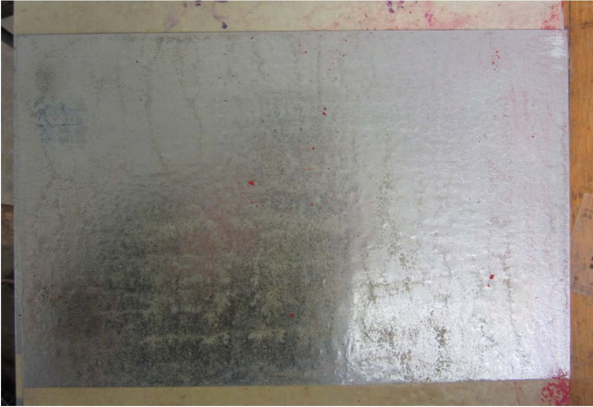
Figure 6: Chemical Resistance Test - MC-500 on steel exposed to paint thinner and gasoline. No alterations.
