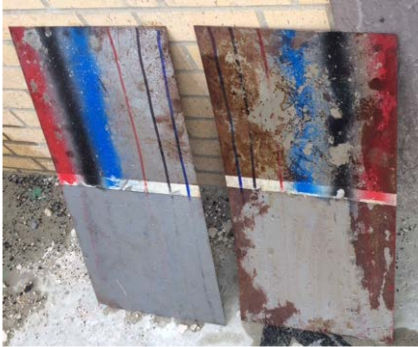
Figure 31a: Pressure Washer Test - 2nd Cycle. Uncoated steel (top) and steel coated with MC-300 (bottom).
