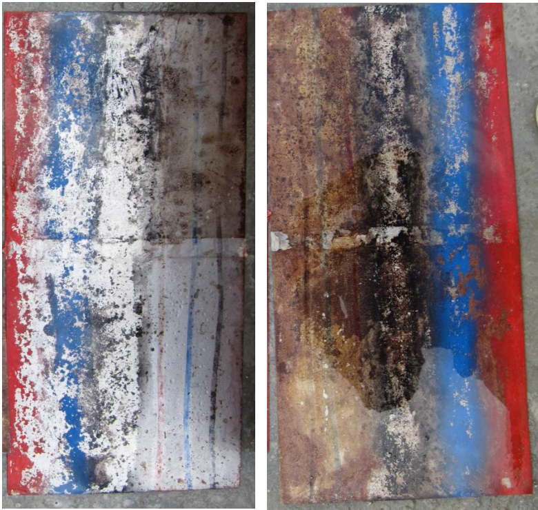
Figure 35b32: Pressure Washer Test - 10th Cycle. Uncoated steel (top) and steel coated with MC-300 (bottom).
