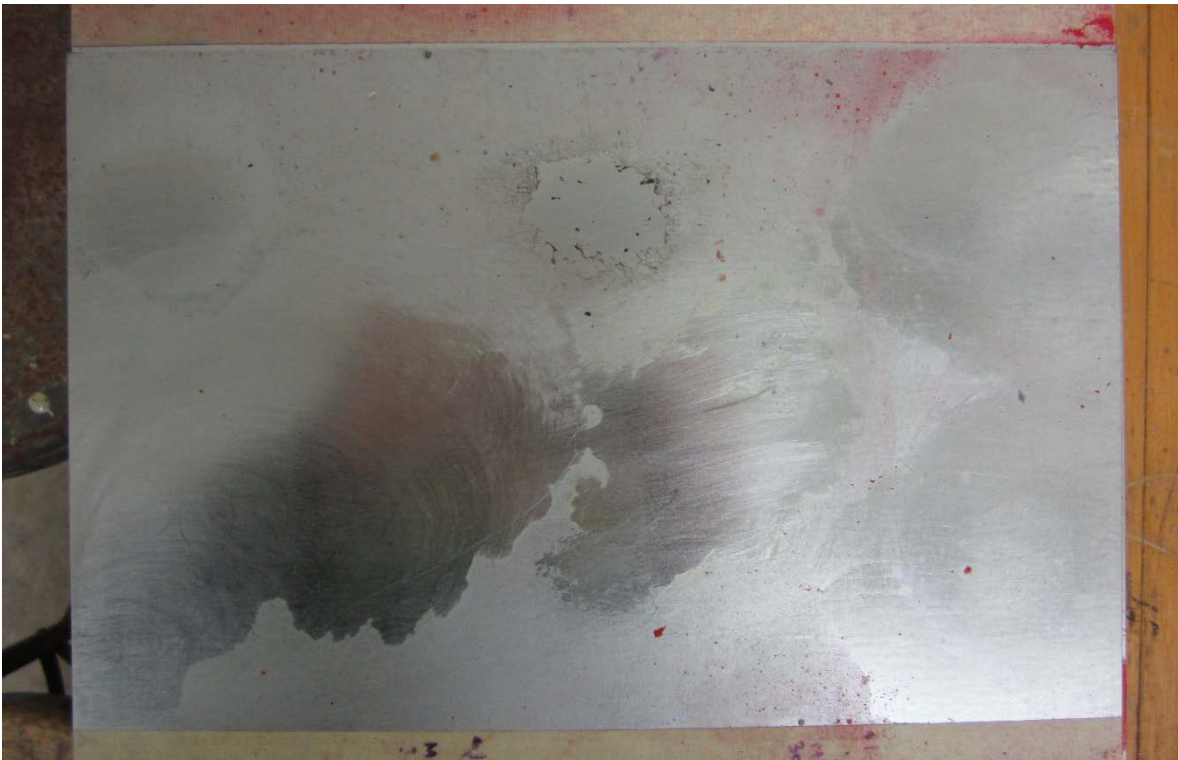
Figure 4: Chemical Resistance Test - MC-300 on steel exposed to paint thinner and gasoline. Complete adhesion loss.
