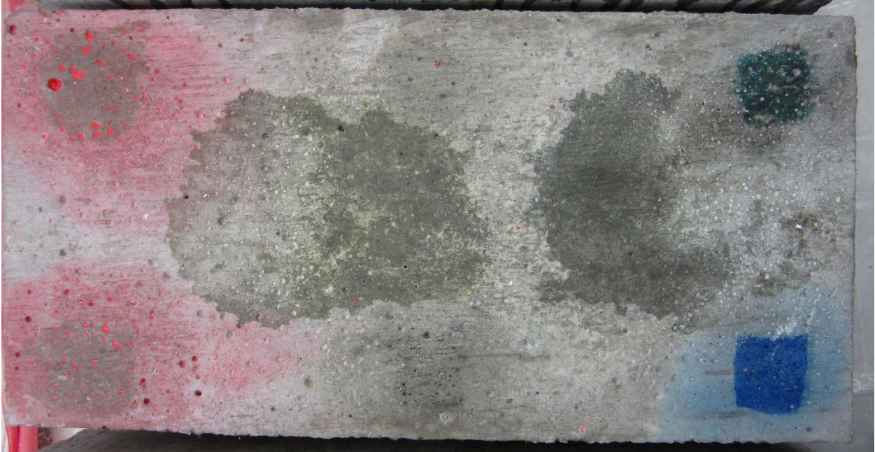
Figure 3: Chemical Resistance Test - MC-300 on concrete exposed to paint thinner and gasoline. Some adhesion loss.
