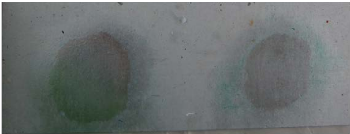
Figure 20: Wear on MC-300 coating after 10 cycles
