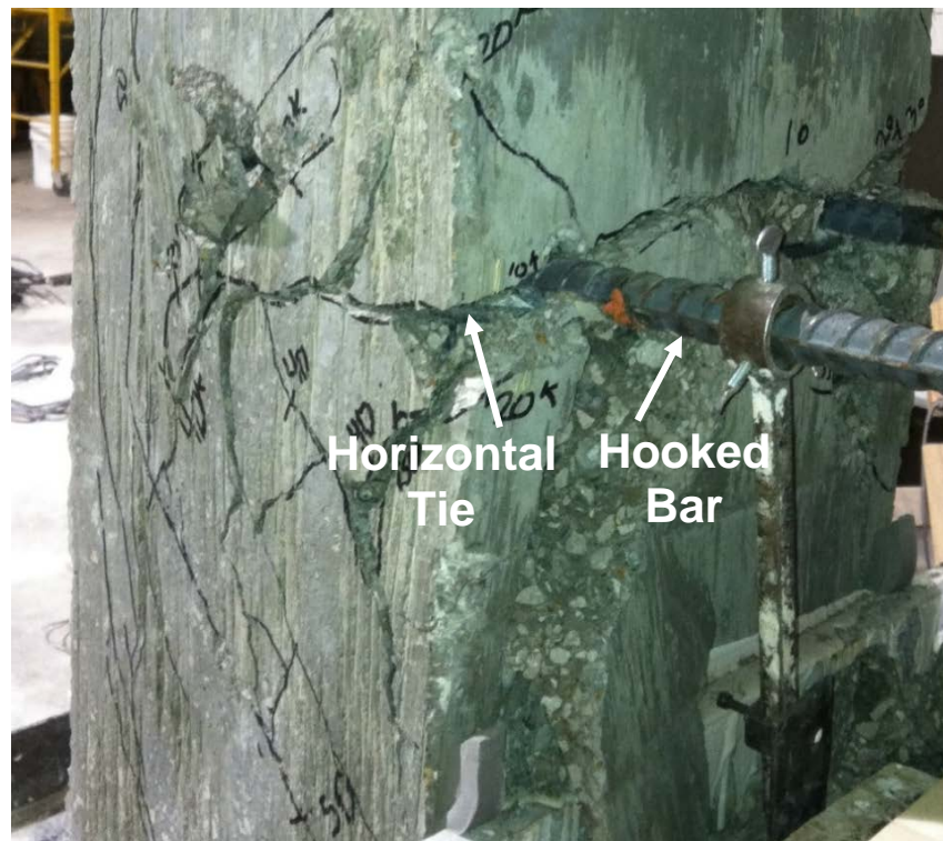
Figure 4.15 Horizontal ties pinning back concrete cone (Specimens 8-12-90-5#3-i-2.5-2-10 after failure)
