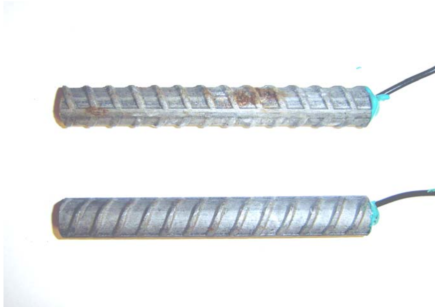
Figure 3.103 – 2101(2)p anode bars in 6.04 m ion NaCl and simulated concrete pore solution showing small amounts of corrosion products on one of the bars, at week 15.
