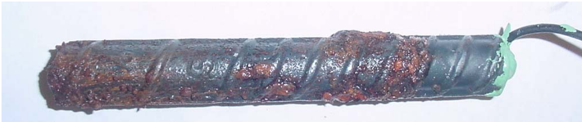
Figure 3.63 – Bare conventional steel (N3) anode bar showing corrosion products that formed above and below the surface of the solution at week 15.
