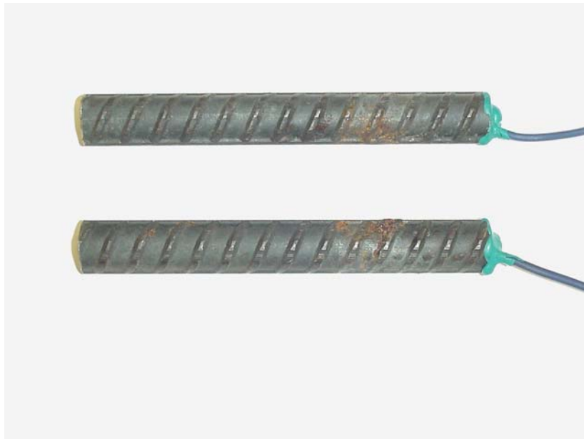
Figure 3.104 – 2205 anode bars in 6.04 m ion NaCl and simulated concrete pore solution showing some corrosion products at week 15.
