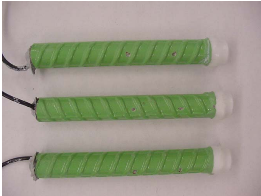
Figure 3.85 – Epoxy-coated anode bars with no corrosion products after removal of mortar cover at week 15.
