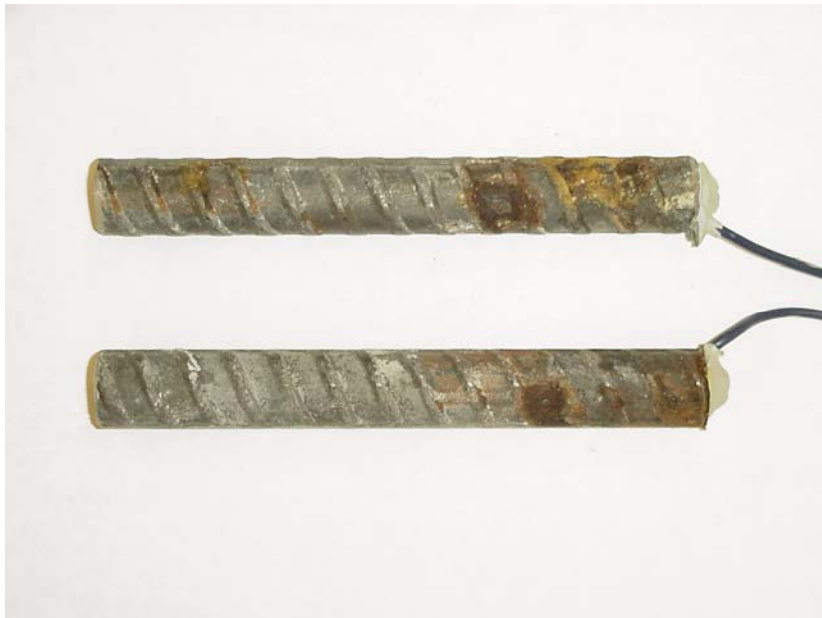
Figure 3.109 – Corrosion products on 2101(1) anode bars after removal of mortar cover at week 15.
