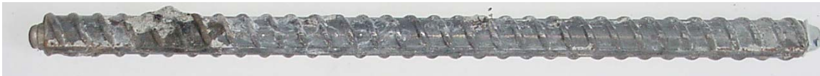
Figure 3.130 – Corrosion products on 2205 steel bar from top mat of cracked beam specimen, at week 96
