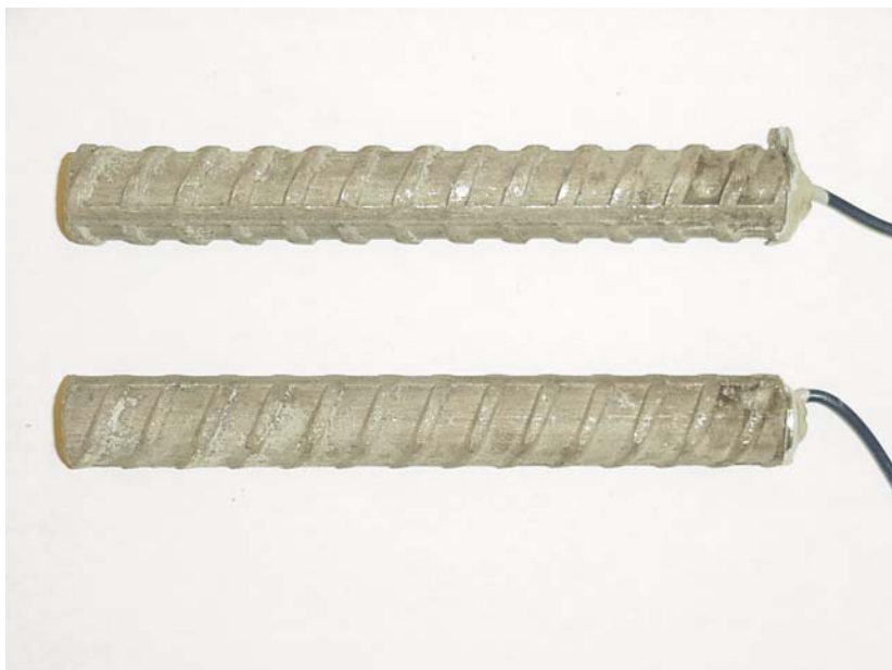
Figure 3.110 – 2101(1)p anode bars after removal of mortar cover at week 15 showing no corrosion products.
