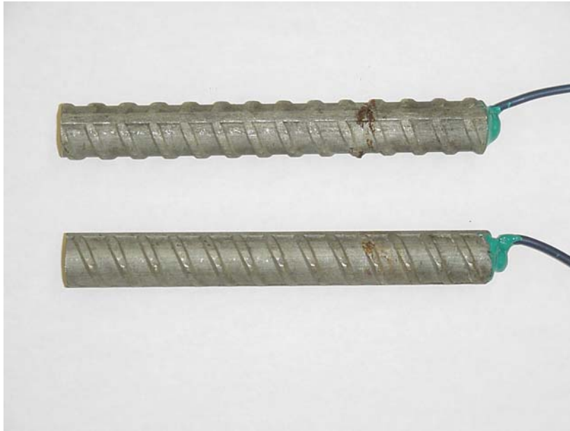
Figure 3.101 – 2101(1)p anode bars in 6.04 m ion NaCl and simulated concrete pore solution showing small amounts of corrosion products at week 15.
