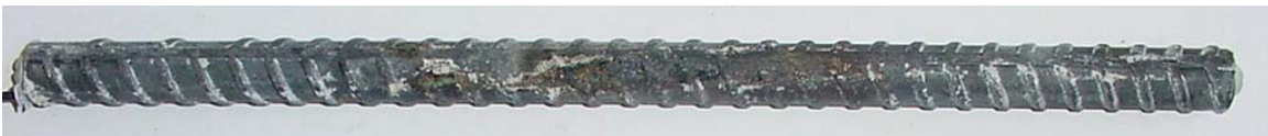
Figure 3.129 – Corrosion products on 2101(2) steel bar from top mat of cracked beam specimen, at week 96.
