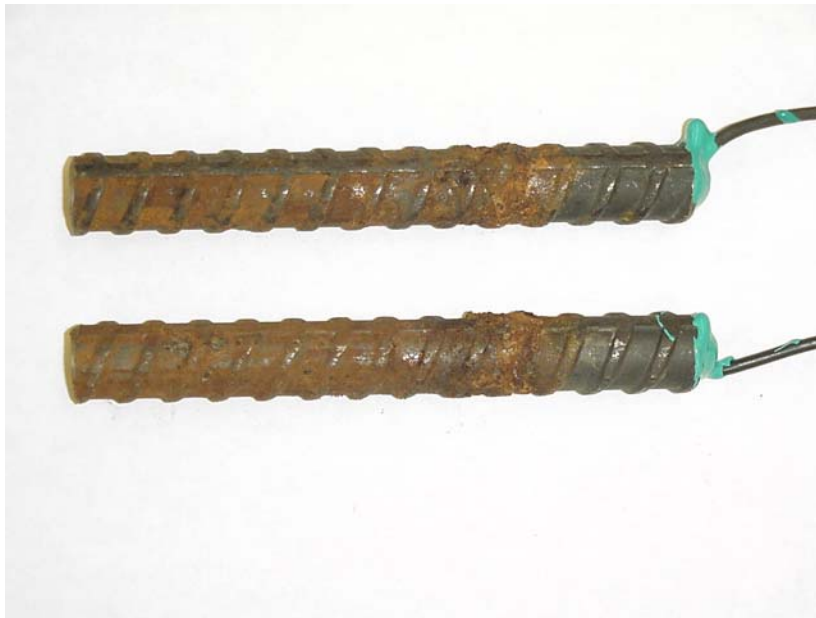
Figure 3.100 – Corrosion products on 2101(1) anode bars in 6.04 m ion NaCl and simulated concrete pore solution at week 15.
