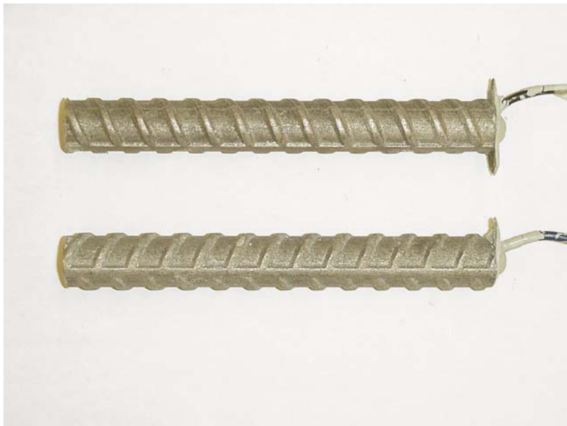
Figure 3.114 – 2205p anode bars after removal of mortar cover at week 15 showing no corrosion products.
