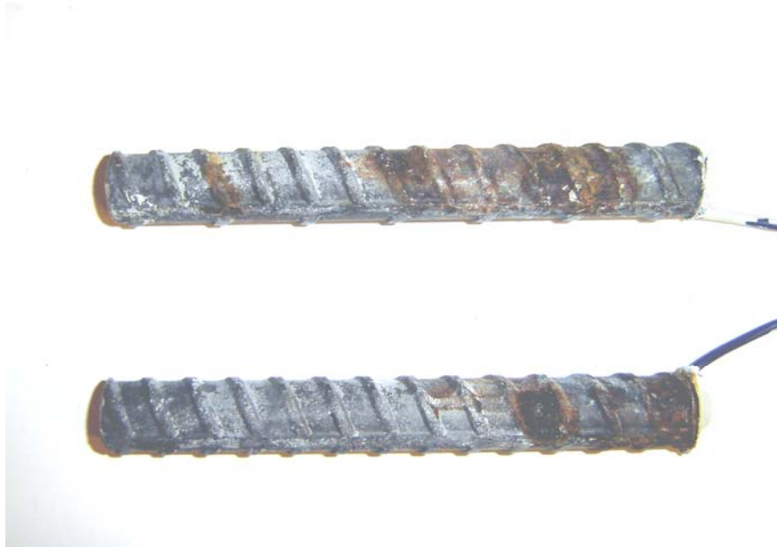
Figure 3.111 – Corrosion products on 2101(2) anode bars after removal of mortar cover at week 15.
