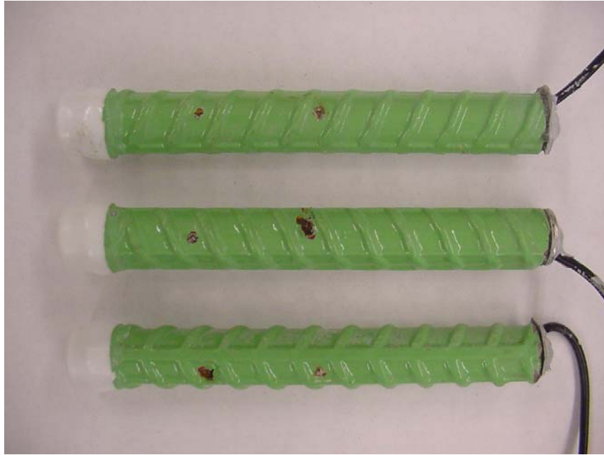
Figure 3.84 – Corrosion products on exposed steel on epoxy-coated anode bars after removal of mortar cover at week 15.
