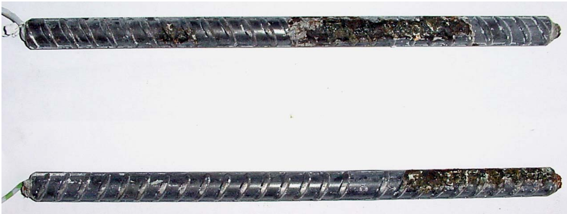
Figure 3.76 - Corrosion products on MMFX microcomposite steel bars from top mat of a Southern Exposure specimen, at week 96.
