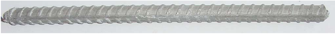
Figure 3.132 – 2101(2)p bar used on top mat of cracked beam specimen, showing no corrosion products, at week 96.
