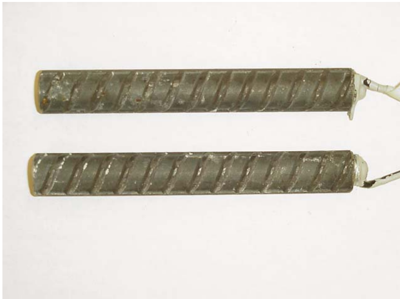
Figure 3.113 – 2205 anode bars after removal of mortar cover at week 15 showing no corrosion products.
