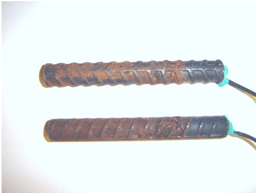
Figure 3.102 – Corrosion products on 2101(2) anode bars in 6.04 m ion NaCl and simulated concrete pore solution at week 15.
