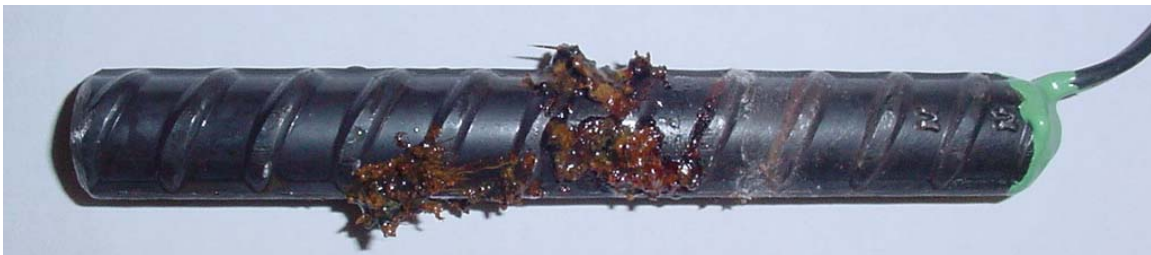
Figure 3.62 – Bare MMFX steel anode bar from group MMFX(2), showing corrosion products that formed below the surface of the solution at week 15.
