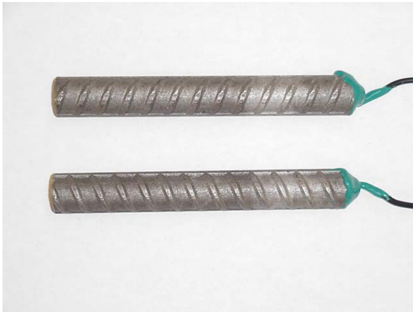
Figure 3.105 – 2205p anode bars in 6.04 m ion NaCl and simulated concrete pore solution showing no corrosion products at week 15.
