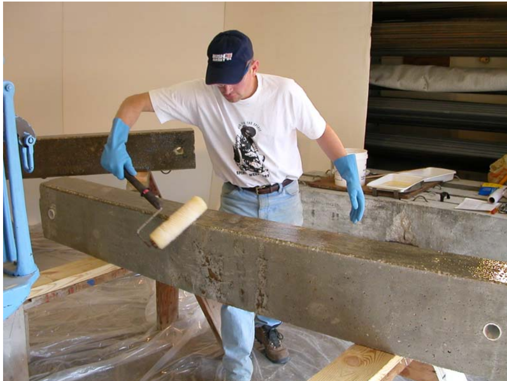
Figure A.38 – One coat of MBrace Primer was applied to each beam using a short nap roller
