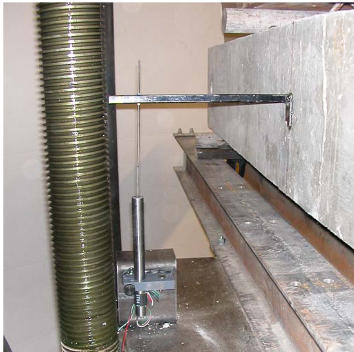
Figure A.54 – Displacement transducer measured the deflection of the centerline of the beam. The horizontal bar was epoxyed to the side of the beam and the transducer rod was firmly attached to the bar with two nuts. The transducer had a 2 in. (50 mm) displacement capacity.
