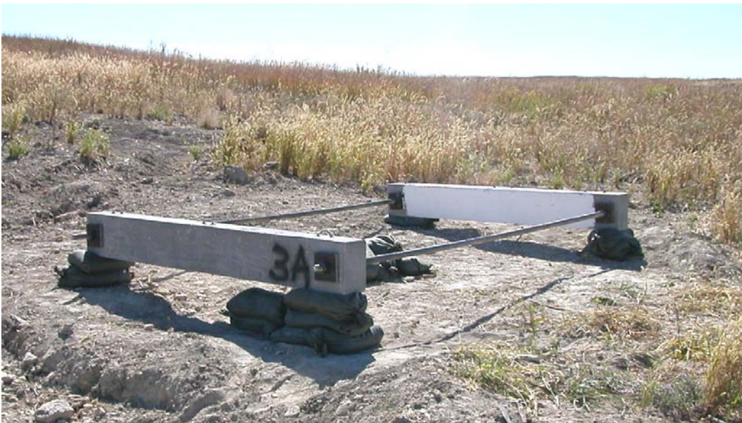
Figure A.8 – Beam blast configuration for Set 3
