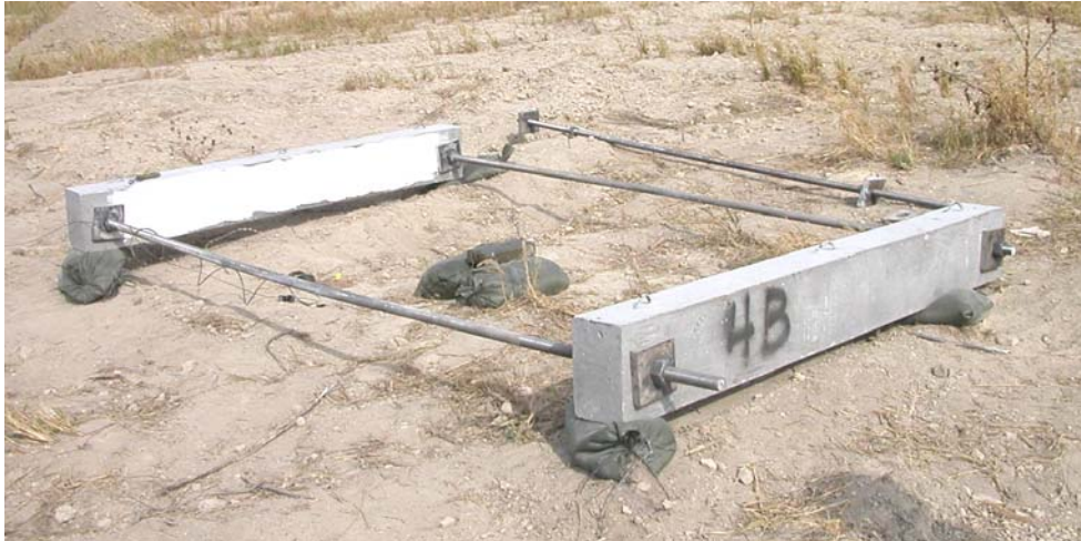
Figure A.9 – Beam blast configuration for Set 4
