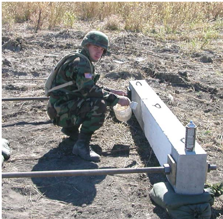
Figure A.10 – Interior face of beams were painted using lime and water to more easily identify cracks. This, however, did not work since the blast blew the lime off.
