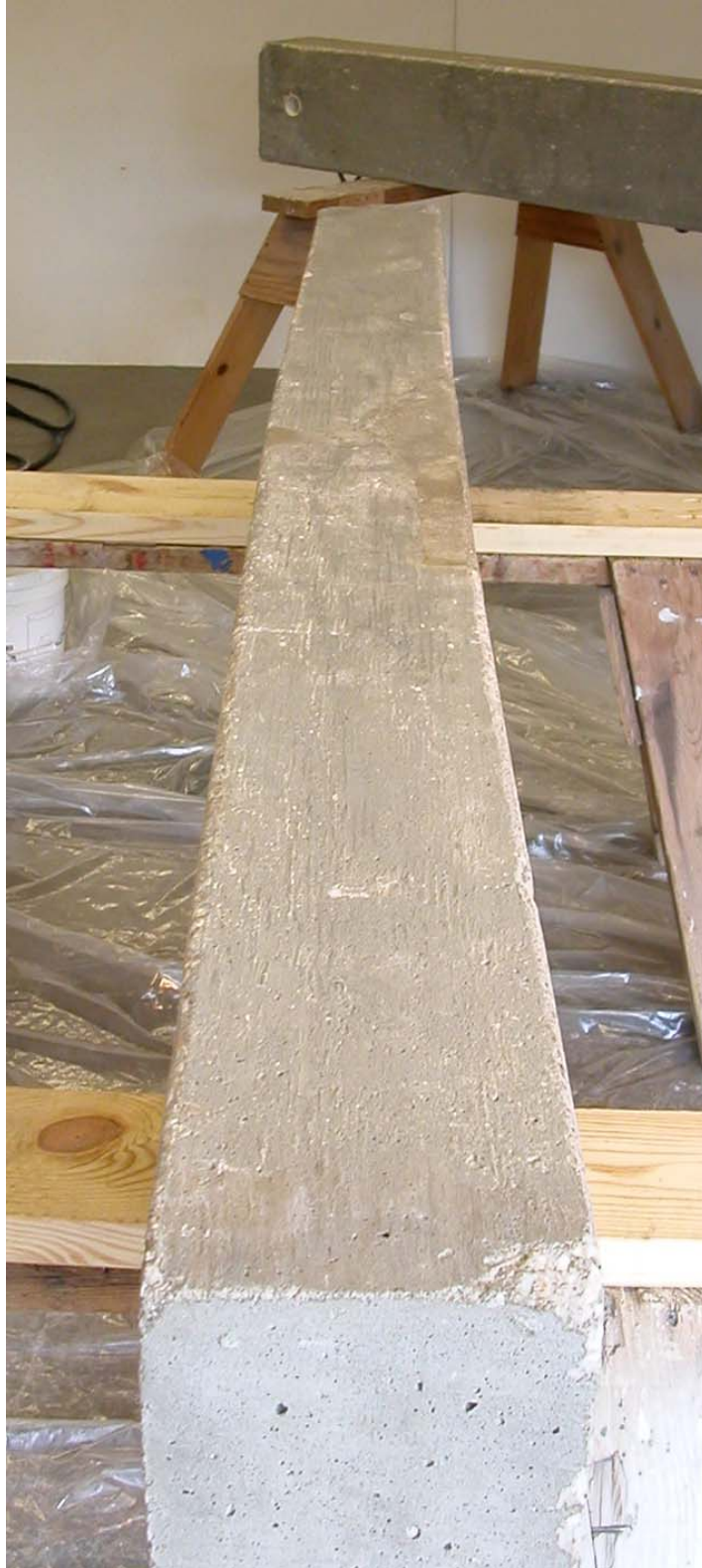
Figure A.36 – Beam 2B still had a slight bow in it after the straightening process had been completed. Beam 4A can be seen in the back ground.
