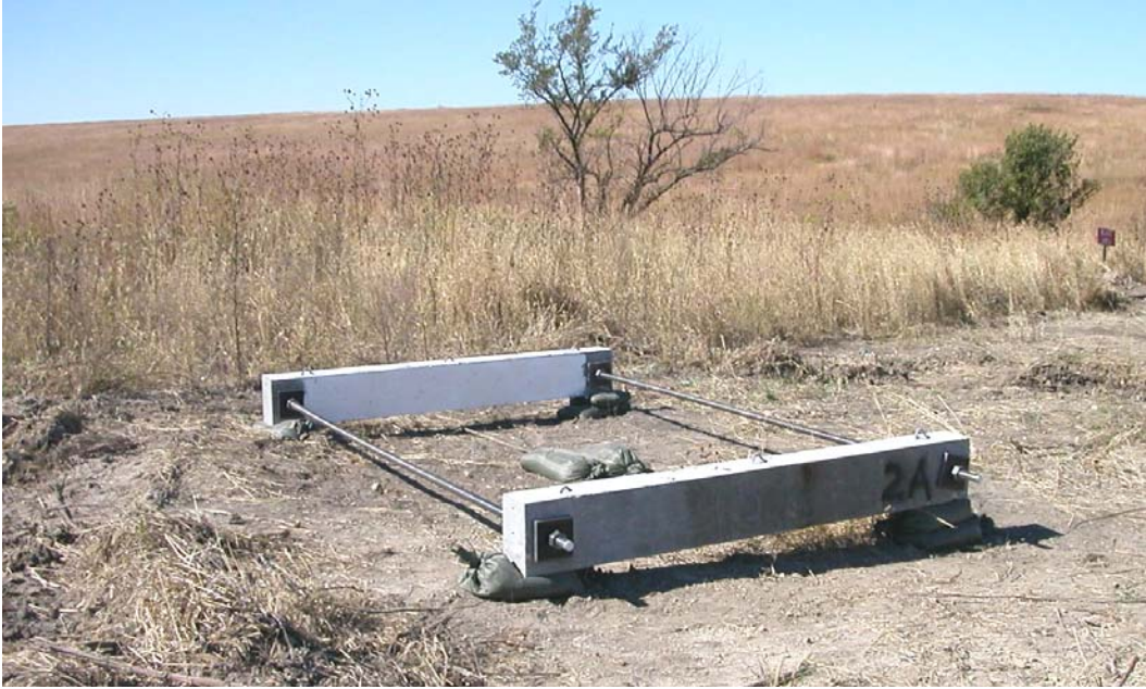
Figure A.7 – Beam blast configuration for Set 2
