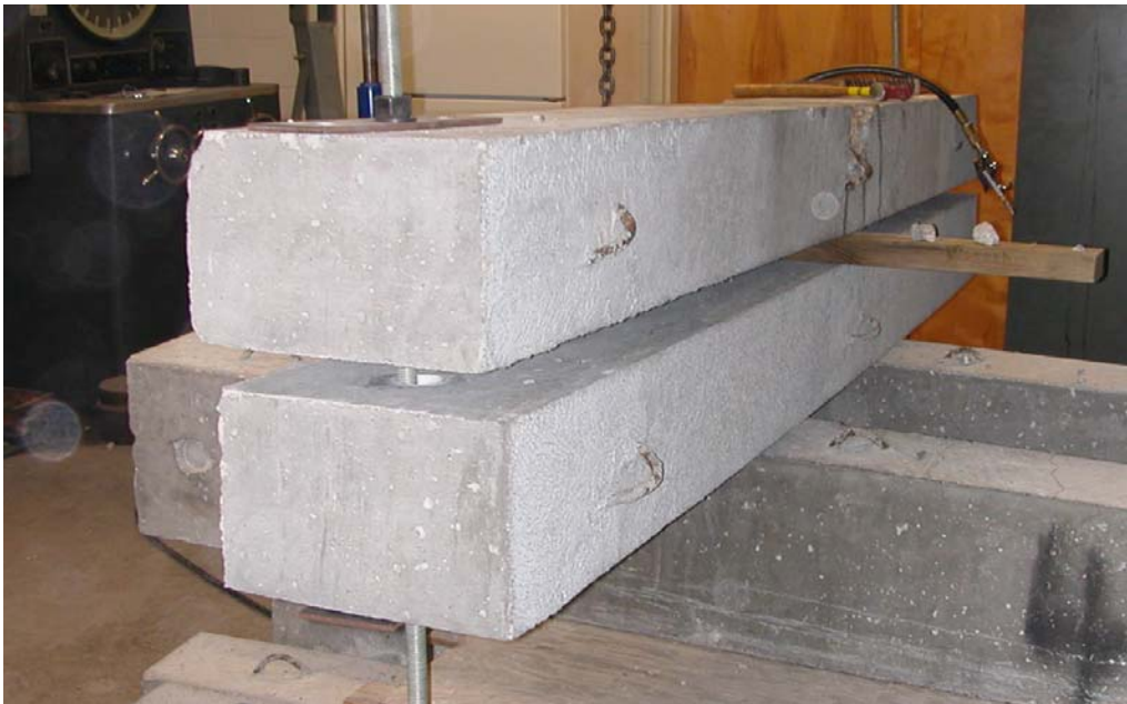
Figure A.26 – Beam 2A was straightened by jacking it against an undamaged beam using threaded rods that were run through the same holes used to hold the beams together during the blast. The large cracks on the outside face of the beam were filled with epoxy adhesive prior to jacking the beam straight.
