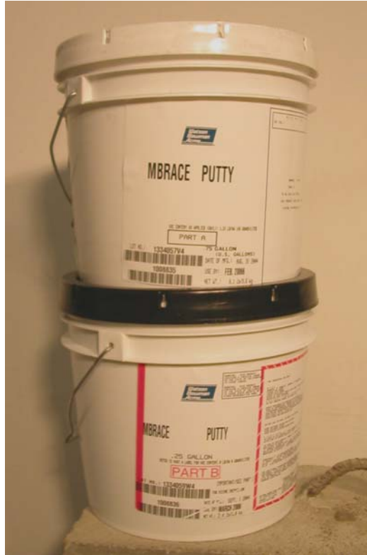
Figure A.41 – The MBRace Putty comes in two parts that are mixed just prior to use. Once mixed, there is about 40 minutes working time prior to setting.
