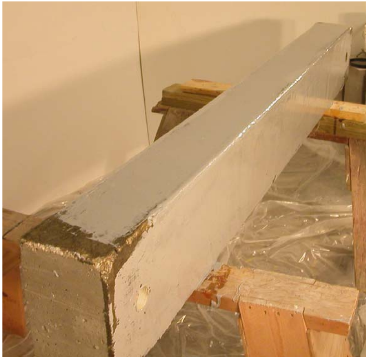
Figure A.44 – The MBrace Putty cured for approximately six hours before the saturant was applied.
