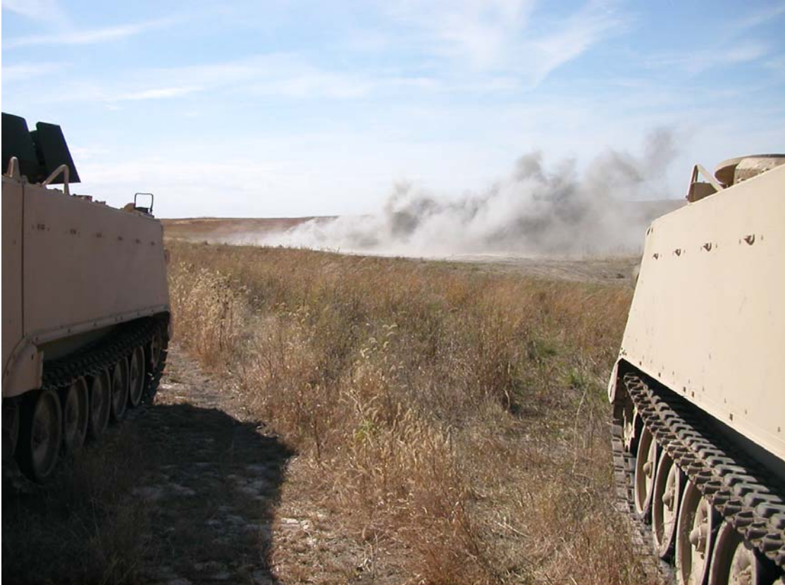
Figure A.13 – The C-4 charges were detonated from behind the safety M113 Armored Personnel Carriers which were located approximately 450 ft (135 m) from the blasts
