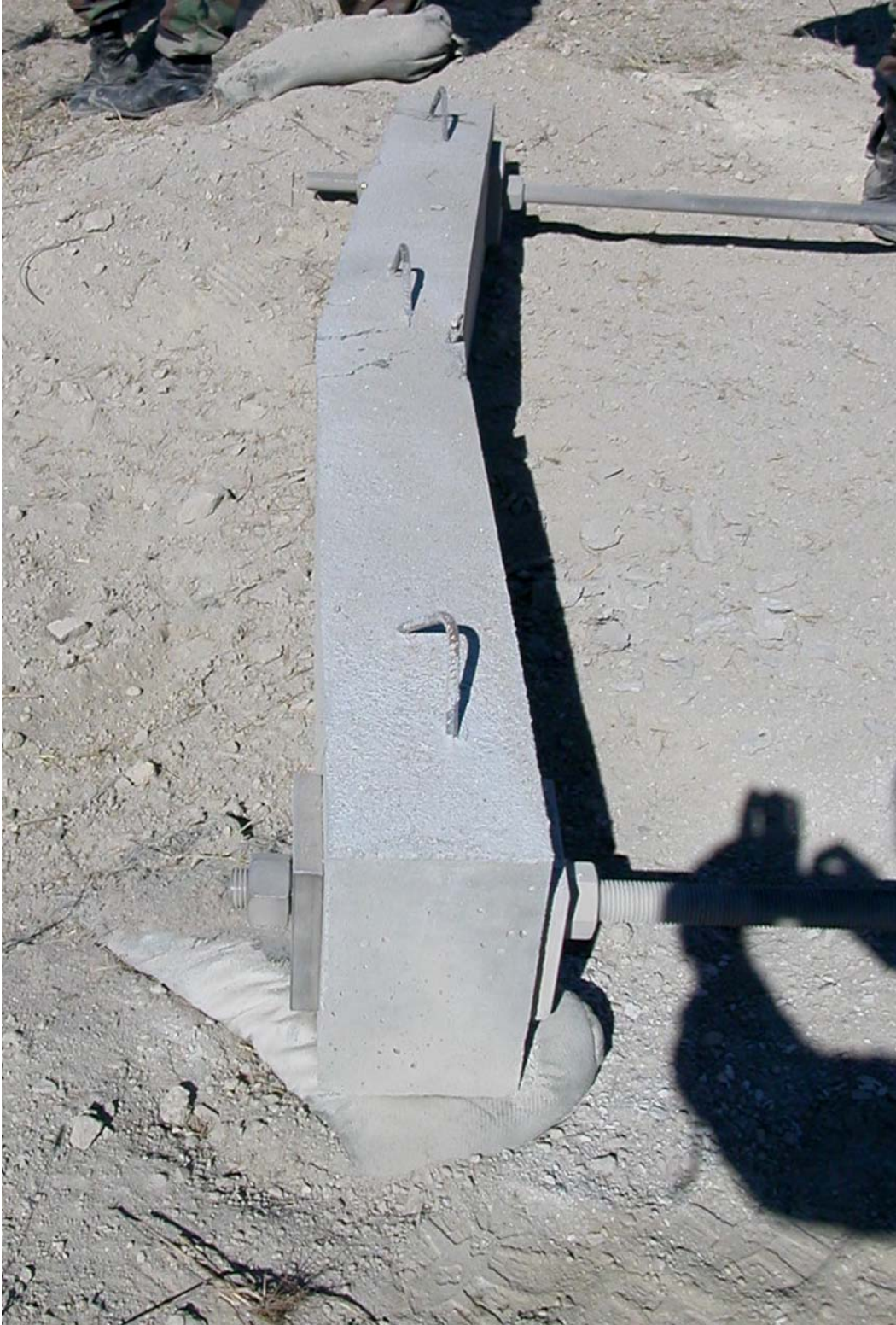
Figure A.16 – Beam 3B following detonation of 15 lbs (6.80 kg) of C-4. Note the outward bend due to the yielding of the concrete beams.
