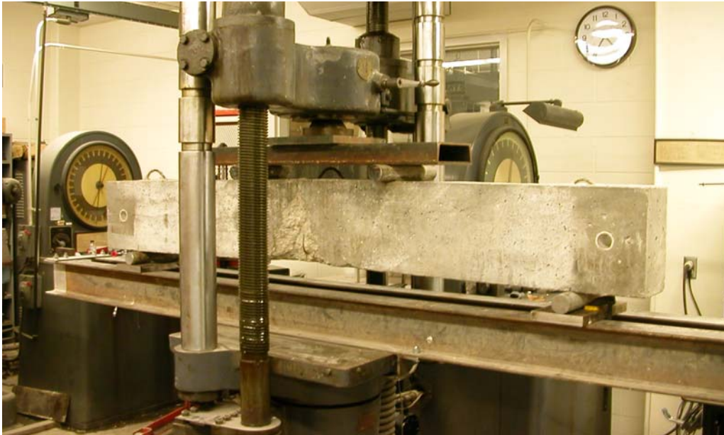
Figure A.53 – Beam 2A mounted in the third-point reaction from on the 120 kip (534 kN) Baldwin Universal Testing Machine.
