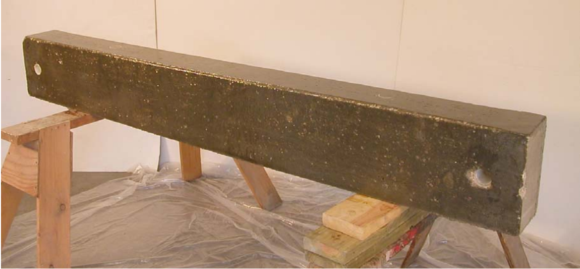
Figure A.39 – The primer cured for approximately 18 hours resulting in a clear, shiny, slightly tacky surface.
