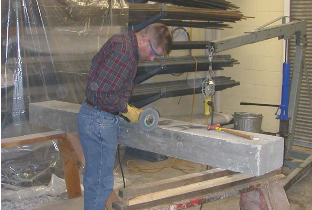
Figure A.25 – The bottom edges of beams 4A and 2A were rounded to a \frac{1}{2} in. (13 mm) diameter radius to reduce the force concentration on the FRP which wraps perpendicular across the edge.
