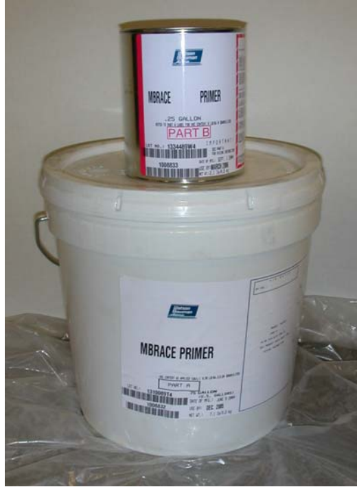
Figure A.37 – The MBrace Primer comes in two parts that are mixed just prior to use. Once mixed, there is about 20 minutes working time prior to setting.
