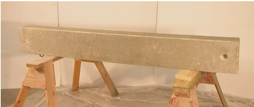
Figure A.35 – Beam 4A after surface preparation but before the application of the primer.
