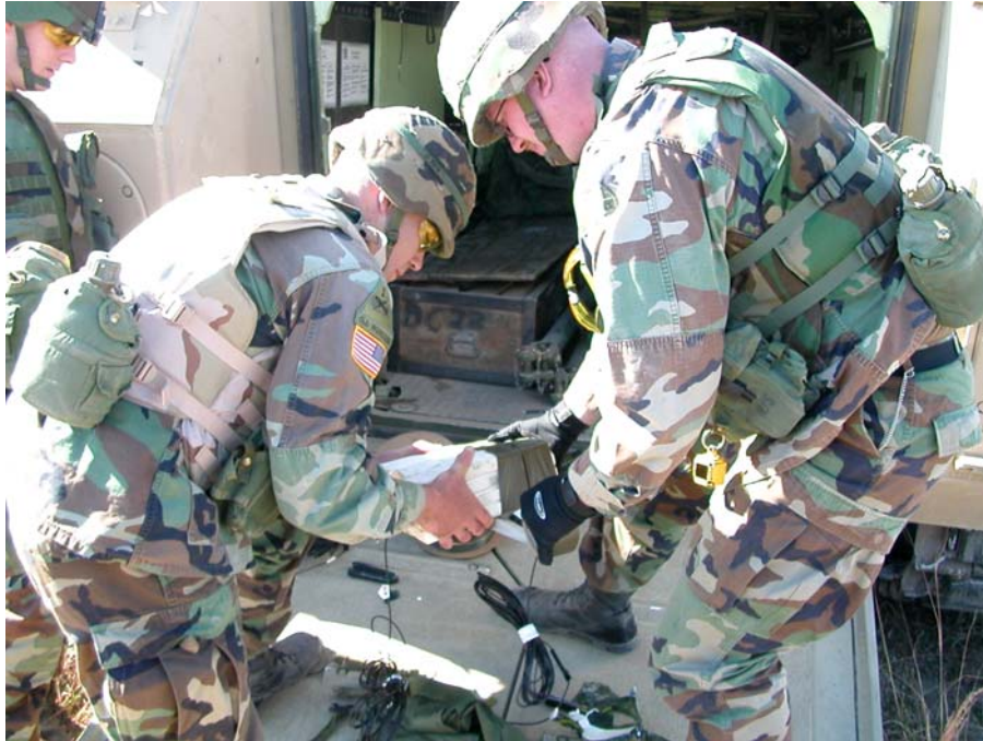
Figure A.11 – The C-4 charge was dual primed and tightly packed into a single large charge for each blast. The charge was tightly wrapped with military issue green duct tape to minimize air voids within the charge.
