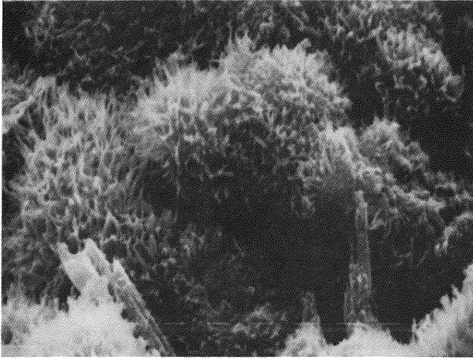
Fig. 2.28. Type I Calcium Silicate Hydrate (CSH); Oven Dried Specimen; magnification = 5000x, \mu marker = 0.9 \mu m
