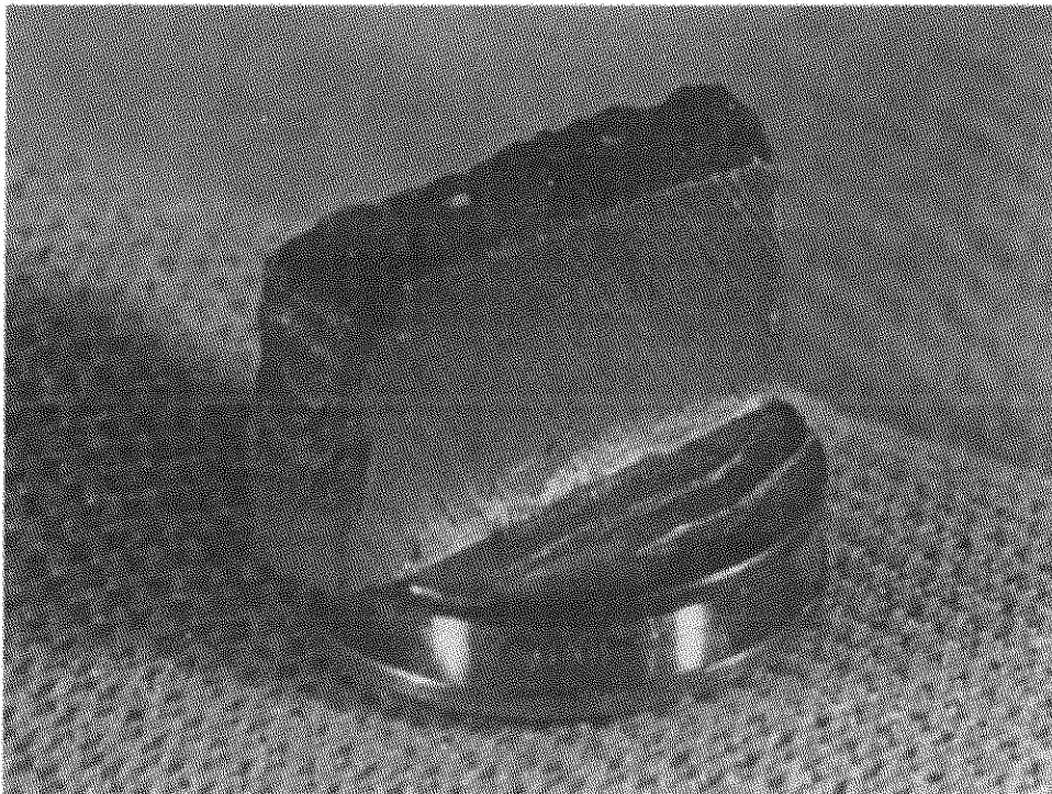
Fig. 2.26. Specimen as Mounted on Stud
