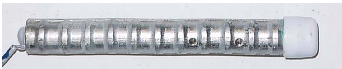
Figure 3.43 – SMI-d anode bar after removal of mortar, at 15 weeks, showing corrosion products that formed at penetrations through the cladding.
