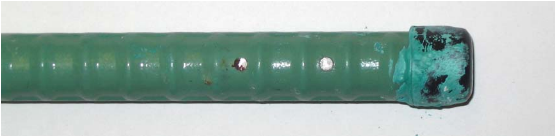
Figure 3.68 – Bare ECR(DuPont) anode bar, at 15 weeks, showing corrosion products that formed at drilled holes.
