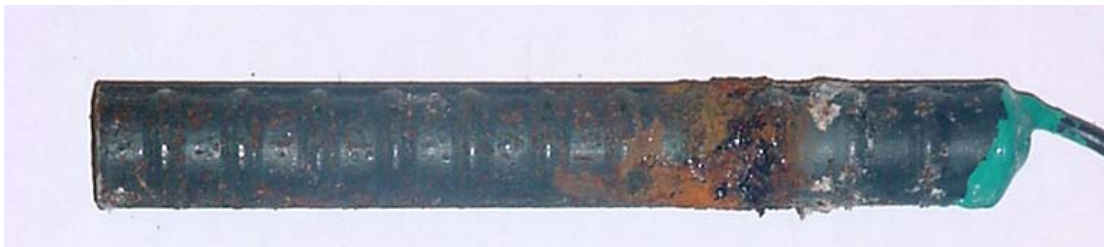
Figure 3.10 – Bare conventional anode bar, at 15 weeks, showing corrosion products that formed at contact points between the bar and plastic lid.
