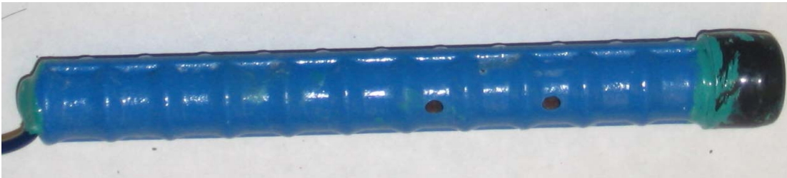
Figure 3.132 – Bare MC anode bar with only epoxy penetrated, at 15 weeks, showing corrosion products that formed at drilled holes
