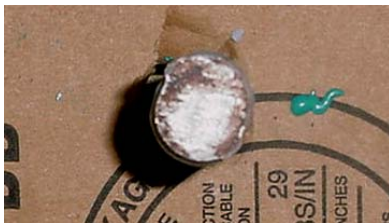
Figure 3.40 – Bare SMI-nc anode bar from 1.6 m ion salt solution, at 15 weeks, showing corrosion products that formed at the unprotected end.
