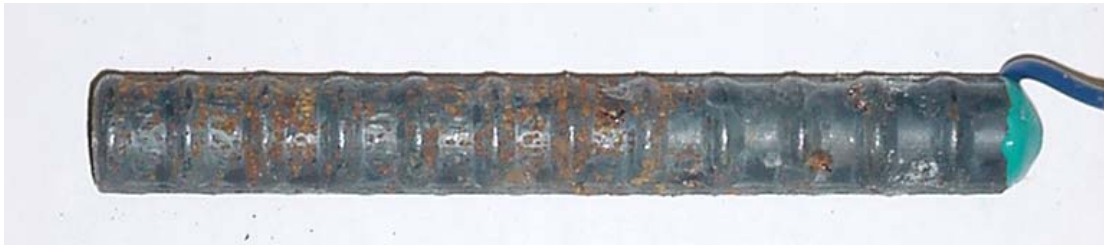
Figure 3.9 – Bare conventional anode bar, at 15 weeks, showing corrosion products that formed below the surface of the solution.
