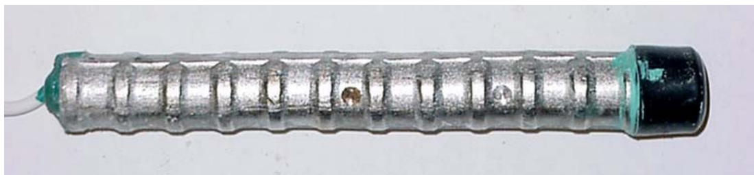
Figure 3.41 – Bare SMI-d anode bar from 1.6 m ion salt solution, at 15 weeks, showing corrosion products that formed at penetrations through the cladding.
