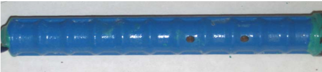
Figure 3.133 – Bare MC anode bar with both layers penetrated, at 15 weeks, showing corrosion products that formed at drilled holes
