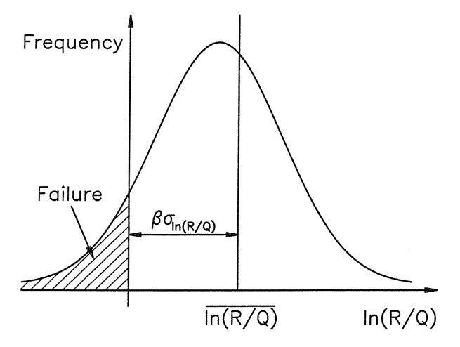
Fig. 1 Illustration of reliability index (after Ellingwood et al. 1980).  $\beta$  = number of standard deviations,  $\sigma_{\ln(R/Q)}$ , between  $\ln(R/Q) = \overline{\ln(R/Q)}$  and  $\ln(R/Q) = 0$ .
