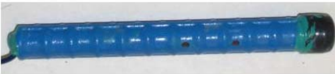
Figure 3.105 – Bare bar specimen. Multiple coated anode bar with only epoxy penetrated showing corrosion products that formed at holes at week 15.
