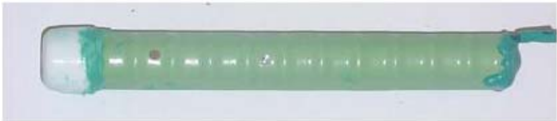
Figure 3.8 – Bare bar specimen. ECR anode bar showing corrosion products that formed at drilled holes at week 15.
