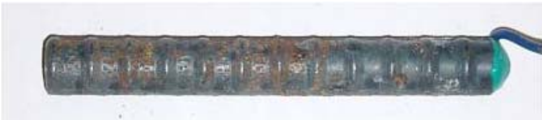
Figure 3.6 – Bare bar specimen. Conventional steel anode bar showing corrosion products that formed below the surface of the solution at week 15.
