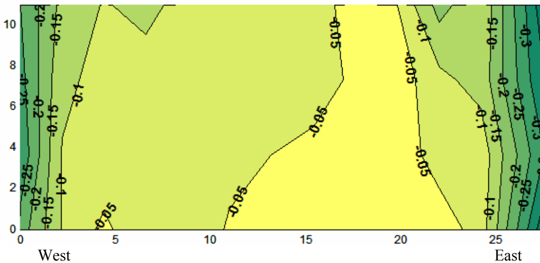
Figure 3.199 – Corrosion potential map for the Mission Creek Bridge (April 1, 2005)
