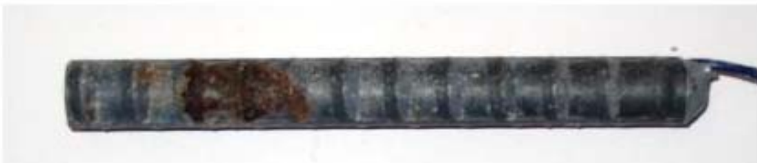
Figure 3.14 – Mortar-wrapped specimen. Conventional steel anode bar showing corrosion products after removal of mortar cover at week 15.
