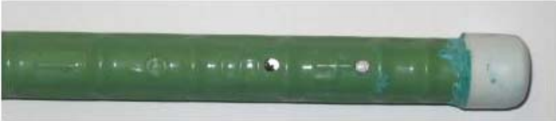
Figure 3.150 – Bare bar specimen. ECR(Valspar) anode bar showing corrosion products that formed at drilled holes at week 15.
