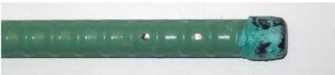
Figure 3.149 – Bare bar specimen. ECR(DuPont) anode bar showing corrosion products that formed at drilled holes at week 15.
