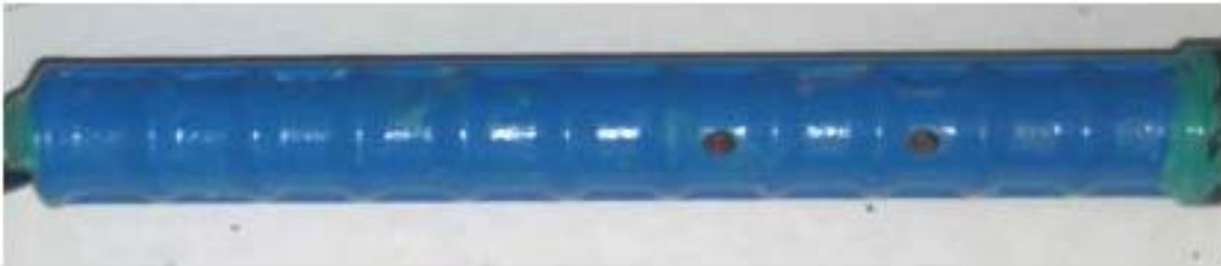
Figure 3.106 – Bare bar specimen. Multiple coated anode bar with both layers penetrated showing corrosion products that formed at holes at week 15.
