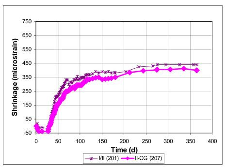
Figure 3.65 - Free Shrinkage, Program IV. Average free shrinkage vs. time for 28-day cure specimens. Comparing cement type through 365 days.
