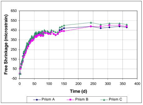
Figure A3.18 - Free Shrinkage, Batch 79. 60% Aggregate, 0.50 w/c. Type II coarse ground (CG) cement. Drying begins on day 3.
