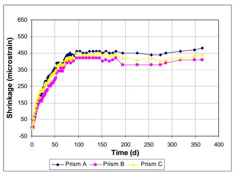
Figure A3.73 - Free Shrinkage, Batch 183. 75% Aggregate, 0.45 w/c. Type I/II cement. Drying begins at 3 days. Control, no chemical admixtures.
