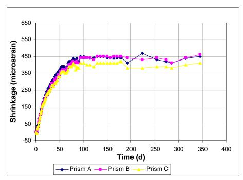
Figure A3.75 - Free Shrinkage, Batch 185. 75% Aggregate, 0.45 w/c. Type I/II cement. Drying begins at 3 days. Medium dosage of Adva 100.
