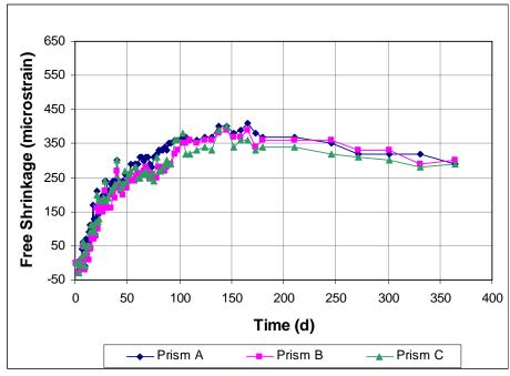
Figure A3.60 - Free Shrinkage, Batch 170. 75% Aggregate, 0.45 w/c. Type I/II cement. Drying begins at 3 days. High dosage of Glenium 3000NS.
