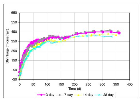
Figure 3.57 - Free Shrinkage, Program IV. Average free shrinkage vs. time for different curing times. Type II coarse ground (CG) cement. Batch 207 through 365 days. Drying only.
