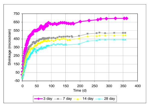
Figure 3.51 - Free Shrinkage, Program IV. Average free shrinkage vs. time for different curing times. Type I/II cement. Batch 201 through 365 days. Drying only.
