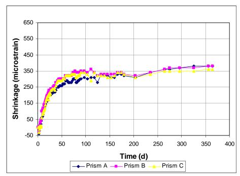
Figure A3.78 - Free Shrinkage, Batch 191. 75% Aggregate, 0.45 w/c. Type I/II cement. Drying begins at 3 days. Medium dosage of Adva 100.
