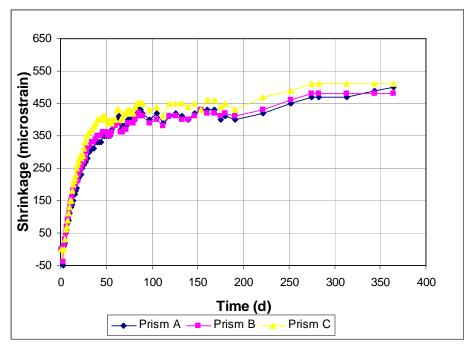
Figure A3.35 - Free Shrinkage, Batch 195. 70% Aggregate, 0.45 w/c. Type I/II cement. Drying begins at 3 days. 30% Replacement by Slag.
