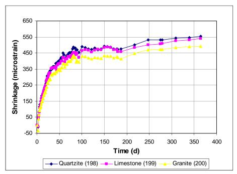
Figure 3.21 Free Shrinkage Test, Program II. Comparison of different aggregate types through 365 days.
