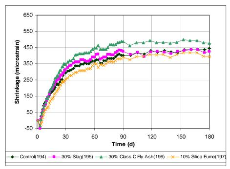
Figure 3.29 Free Shrinkage Test, Program III. Comparing mineral admixtures through 180 days.
