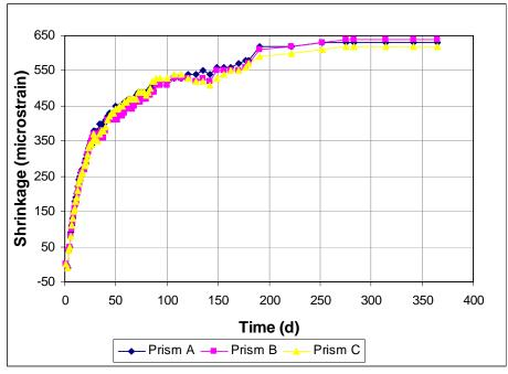
Figure A3.84 - Free Shrinkage, Batch 211. 70% Aggregate, 0.45 w/c. Type I/II cement. Drying begins at 3 days, Rheobuild 1000.
