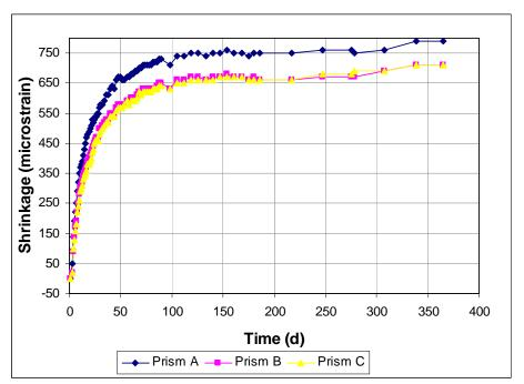
Figure A3.86- Free Shrinkage, Batch 249. 67.8% Aggregate, 0.45 w/c. Type I/II cement. Air-entrained concrete. Drying begins at 3 days. Glenium 3000 NS.
