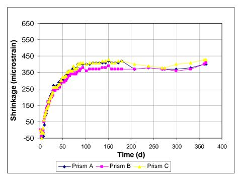
Figure A3.67 - Free Shrinkage, Batch 177. 75% Aggregate, 0.45 w/c. Type I/II cement. Drying begins at 3 days. Medium dosage of Glenium 3000NS.
