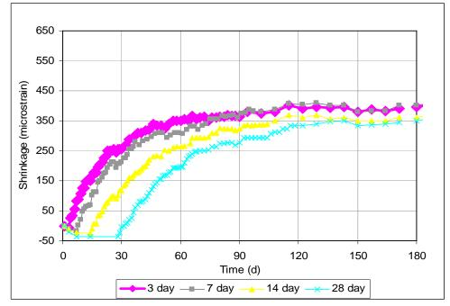
Figure 3.54 - Free Shrinkage, Program IV. Average free shrinkage vs. time for different curing times. Type II coarse ground (CG) cement through 180 days. Batch 207.
