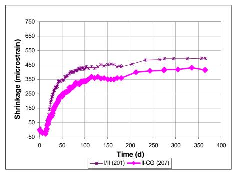
Figure 3.64 - Free Shrinkage, Program IV. Average free shrinkage vs. time for 14-day cure specimens. Comparing cement type through 365 days.
