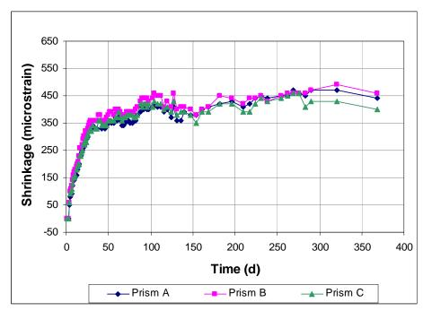
Figure A3.31 - Free Shrinkage, Batch 86. 70% Aggregate, 0.45 w/c. Type I/II cement. Drying begins at 3 days. 30% slag replacement.
