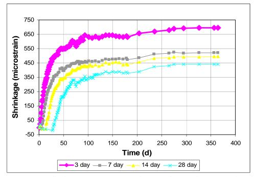
Figure 3.50 - Free Shrinkage, Program IV. Average free shrinkage vs. time for different curing times. Type I/II cement. Batch 201 through 365 days.
