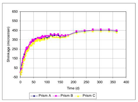
Figure A3.53 Free Shrinkage, Batch 207(3-days-cured), 70% Aggregate, 0.45 w/c ratio, Type II coarse ground (CG) cement. Drying begins at 3 days.
