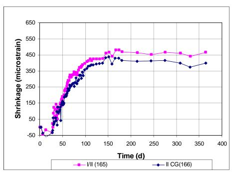
Figure 3.61 - Free Shrinkage, Program IV. Average free shrinkage vs. time for 28-day cure specimens. Comparing cement type through 365 days.
