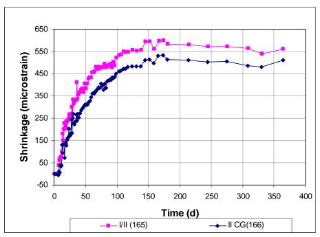
Figure 3.59 - Free Shrinkage, Program IV. Average free shrinkage vs. time for 7-day cure specimens. Comparing cement type through 365 days.
