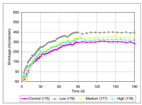
Figure 3.73 Free Shrinkage Test, Program V. Average free shrinkage vs. time. Comparing different dosages of Glenium 3000 NS through 180 days.
