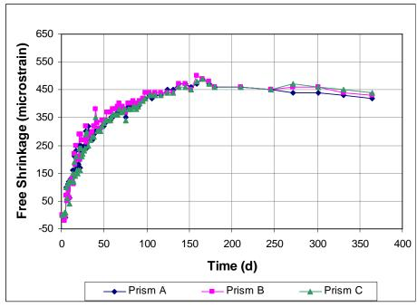
Figure A3.58 - Free Shrinkage, Batch 168. 75% Aggregate, 0.45 w/c. Type I/II cement. Drying begins at 3 days. Low dosage of Glenium 3000NS.
