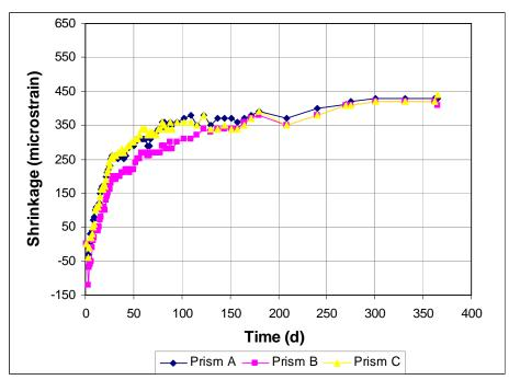
Figure A3.22 - Free Shrinkage, Batch 188. 70% Aggregate, 0.45 w/c. Type I/II cement. Drying begins at 3 days. Limestone.
