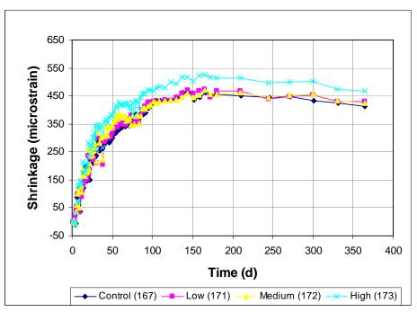
Figure 3.71 Free Shrinkage Test, Program V. Average free shrinkage vs. time. Comparing different dosages of Rheobuild 1000 through 365 days.
