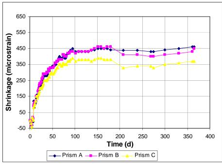
Figure A3.70 - Free Shrinkage, Batch 180. 75% Aggregate, 0.45 w/c. Type I/II cement. Drying begins at 3 days. Medium dosage of Rheobuild 1000.
