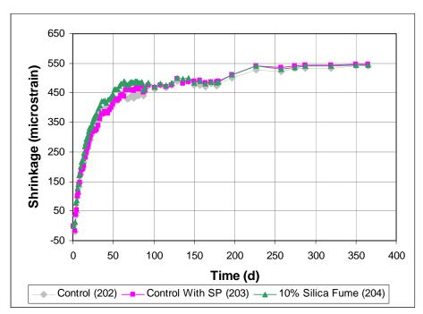
Figure 3.33 Free Shrinkage Test, Program III. Comparing Silica Fume and controls through 365 days.
