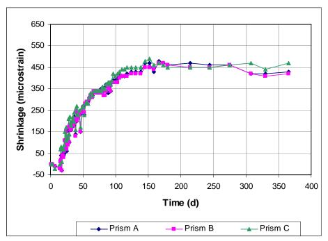
Figure A3.47 - Free Shrinkage, Batch 166, 14-day cure. 70% Aggregate, 0.45 w/c. Type II coarse ground (CG) cement. Drying begins at 14 days.
