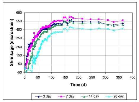
Figure 3.38 - Free Shrinkage, Program IV. Average free shrinkage vs. time for different curing times. Batch 165. Type I/II cement through 365 days.
