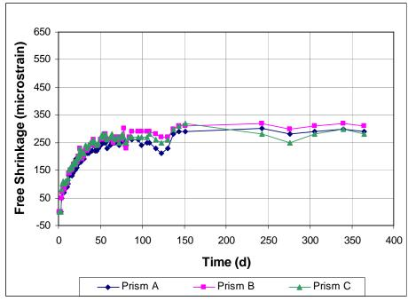
Figure A3.12 - Free Shrinkage, Batch 73. 80% Aggregate, 0.50 w/c. Type II coarse ground (CG) cement. Drying begins on day 3.
