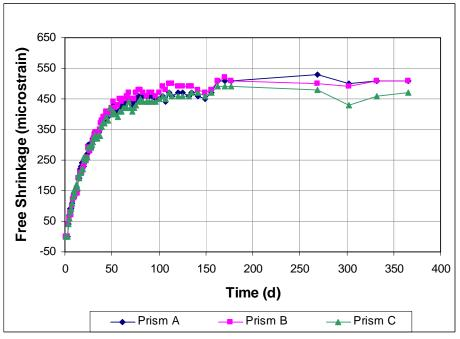
Figure A3.4 - Free Shrinkage, Batch 65. 70% Aggregate, 0.50 w/c. Type I/II cement. Drying begins on day 3.
