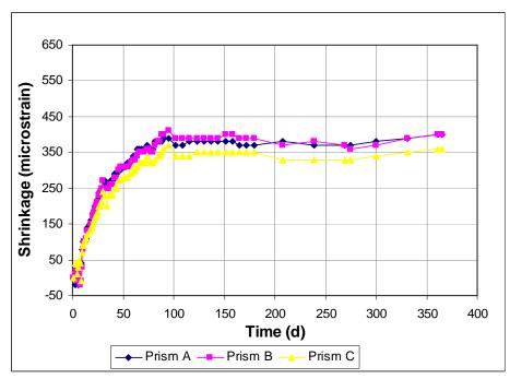
Figure A3.68 - Free Shrinkage, Batch 178. 75% Aggregate, 0.45 w/c. Type I/II cement. Drying begins at 3 days. High dosage of Glenium 3000NS.
