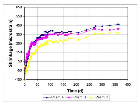
Figure A3.21 - Free Shrinkage, Batch 187. 70% Aggregate, 0.45 w/c. Type I/II cement. Drying begins at 3 days. Quartzite.
