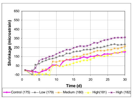
Figure 3.75 Free Shrinkage Test, Program V. Average free shrinkage vs. time. Comparing different dosages of Rheobuild 1000 through 30 days.
