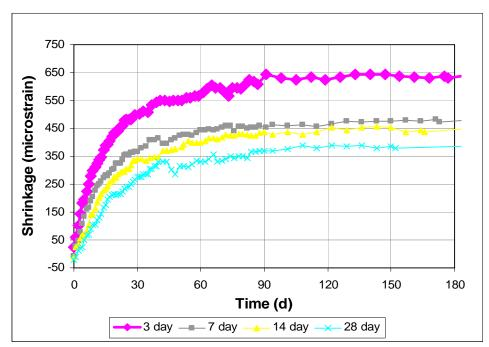
Figure 3.49 - Free Shrinkage, Program IV. Average free shrinkage vs. time for different curing times. Type I/II cement. Batch 201 through 180 days. Drying only.
