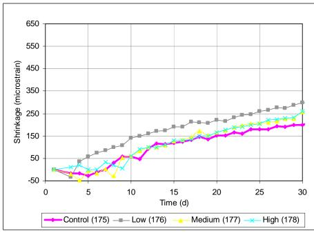
Figure 3.72 Free Shrinkage Test, Program V. Average free shrinkage vs. time. Comparing different dosages of Glenium 3000 NS through 30 days.
