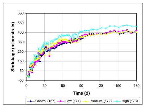
Figure 3.70 Free Shrinkage Test, Program V. Average free shrinkage vs. time. Comparing different dosages of Rheobuild 1000 through 180 days.
