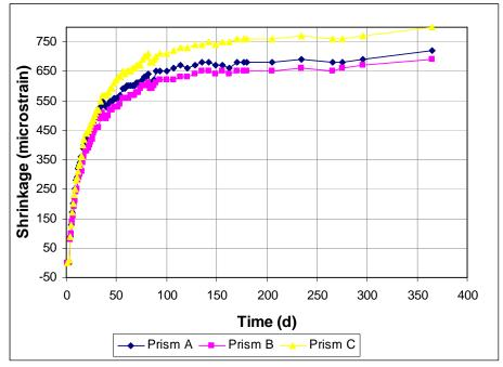
Figure A3.88 - Free Shrinkage, Batch 259 67.8% Aggregate, 0.45 w/c. Type I/II cement. Air-entrained concrete. Drying begins at 3 days. Adva 100.
