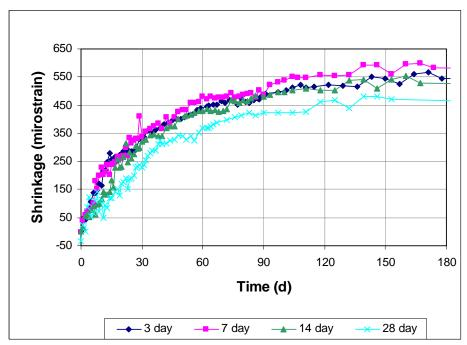
Figure 3.37 - Free Shrinkage, Program IV. Average free shrinkage vs. time for different curing times. Batch 165. Type I/II cement through 180 days. Drying only.
