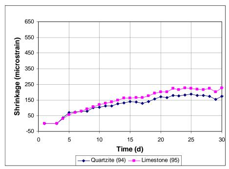
Figure 3.13 Free Shrinkage Test, Program II. Comparison of different aggregate types through 30 days.
