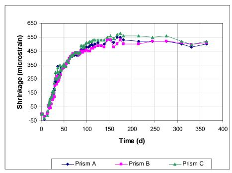
Figure A3.43 - Free Shrinkage, Batch 165, 14-day cure. 70% Aggregate, 0.45 w/c. Type I/II cement. Drying begins at 14 days.
