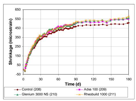
Figure 3.85 Free Shrinkage Test, Program V. Average free shrinkage vs. time. Comparing different Superplasticizers (Dosages for same slump) through 180 days.
