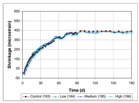
Figure 3.79 Free Shrinkage Test, Program V. Average free shrinkage vs. time. Comparing different dosages of Adva 100 through 180 days.
