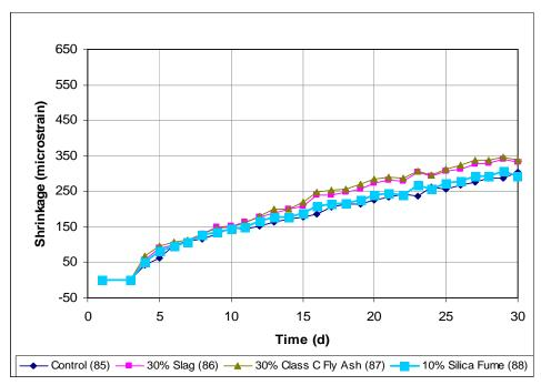
Figure 3.25 Free Shrinkage Test, Program III. Comparing mineral admixtures through 30 days.
