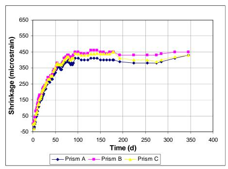
Figure A3.76 - Free Shrinkage, Batch 186. 75% Aggregate, 0.45 w/c. Type I/II cement. Drying begins at 3 days. High dosage of Adva 100.
