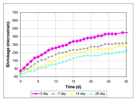
Figure 3.47 - Free Shrinkage, Program IV. Average free shrinkage vs. time for different curing times. Type I/II cement. Batch 201 through 30 days. Drying only.
