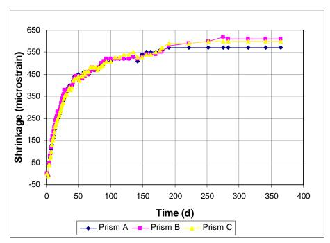
Figure A3.83 - Free Shrinkage, Batch 210. 70% Aggregate, 0.45 w/c. Type I/II cement. Drying begins at 3 days, Glenium 3000 NS.
