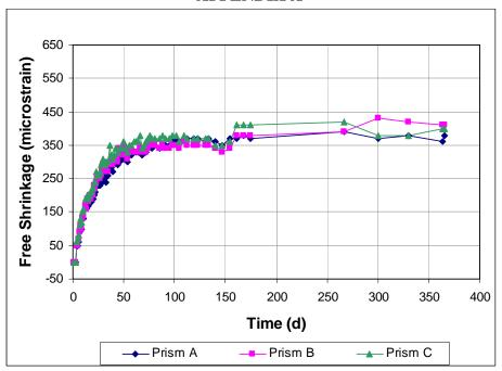
Figure A3.1 - Free Shrinkage, Batch 62. 80% Aggregate, 0.40 w/c. Type I/II cement. Drying begins at 3 days.
