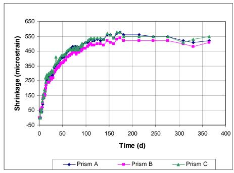
Figure A3.41 - Free Shrinkage, Batch 165, 3-day cure. 70% Aggregate, 0.45 w/c. Type I/II cement. Drying begins at 3 days.
