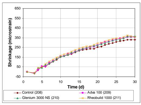
Figure 3.84 Free Shrinkage Test, Program V. Average free shrinkage vs. time. Comparing different Superplasticizers (Dosages for same slump) through 30 days.
