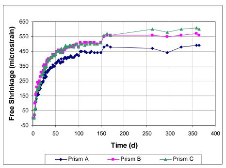
Figure A3.5 - Free Shrinkage, Batch 66. 70% Aggregate, 0.40 w/c. Type I/II cement. Drying begins on day 3.
