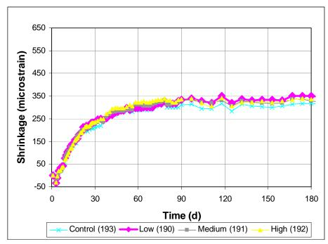
Figure 3.82 Free Shrinkage Test, Program V. Average free shrinkage vs. time. Comparing different dosages of Adva 100 through 180 days.
