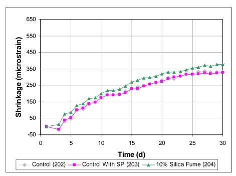
Figure 3.31 Free Shrinkage Test, Program III. Comparing Silica Fume and controls through 30 days.
