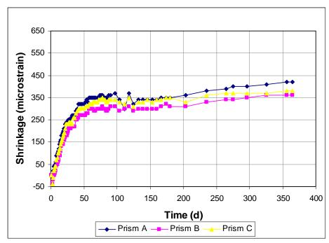
Figure A3.79 - Free Shrinkage, Batch 192. 75% Aggregate, 0.45 w/c. Type I/II cement. Drying begins at 3 days. High dosage of Adva 100.
