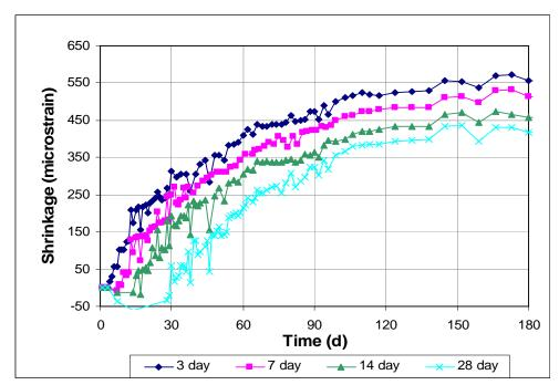
Figure 3.42 - Free Shrinkage, Program IV. Average free shrinkage vs. time for different curing times. Batch 166 through 180 days. Type II coarse ground (CG) cement.
