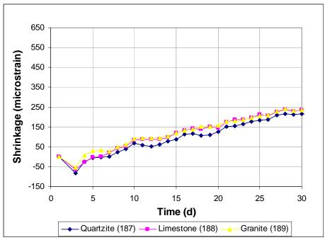
Figure 3.16 Free Shrinkage Test, Program II. Comparison of different aggregate types through 30 days.
