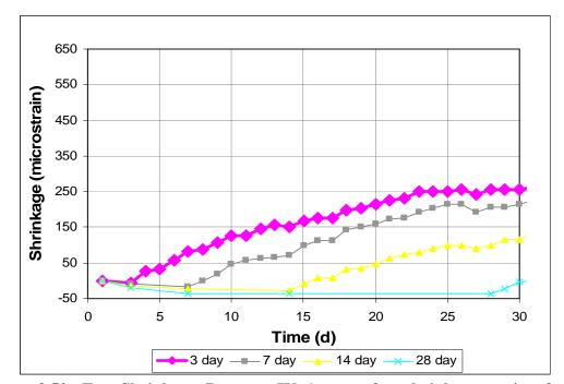
Figure 3.52 - Free Shrinkage, Program IV. Average free shrinkage vs. time for different curing times. Type II coarse ground (CG) cement. Batch 207 through 30 days.
