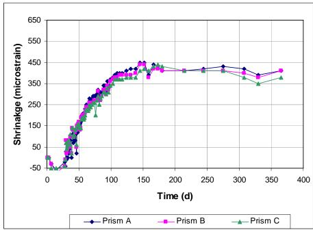
Figure A3.48 - Free Shrinkage, Batch 166, 28-day cure. 70% Aggregate, 0.45 w/c. Type II coarse ground (CG) cement. Drying begins at 28 days.
