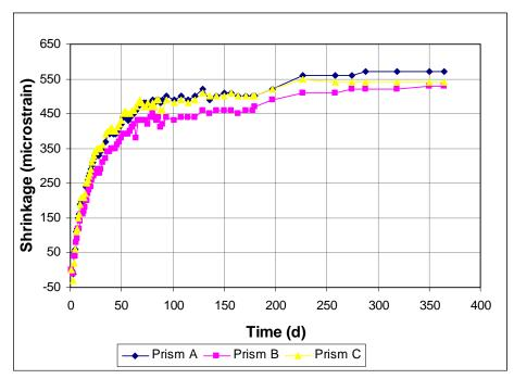
Figure A3.39 - Free Shrinkage, Batch 203. 70% Aggregate, 0.45 w/c. Type I/II cement. Drying begins at 3 days. Control, no mineral admixtures. Adva superplasticizer.
