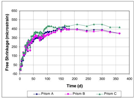
Figure A3.62 - Free Shrinkage, Batch 172. 75% Aggregate, 0.45 w/c. Type I/II cement. Drying begins at 3 days. Medium dosage of Rheobuild 1000.
