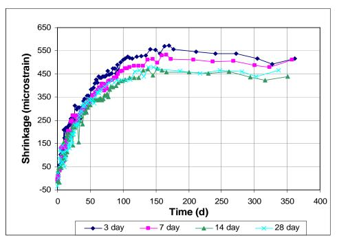
Figure 3.45 - Free Shrinkage, Program IV. Average free shrinkage vs. time for different curing times. Batch 166. Type II coarse ground (CG) cement through 365 days. Drying only.
