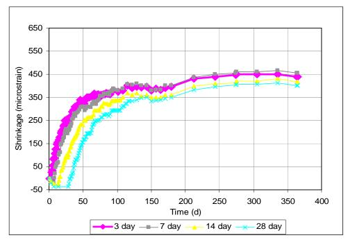
Figure 3.56 - Free Shrinkage, Program IV. Average free shrinkage vs. time for different curing times. Type II coarse ground (CG) cement. Batch 207 through 365 days.
