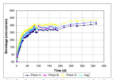
Figure A3.26 - Free Shrinkage, Batch 200. 70% Aggregate, 0.45 w/c. Type I/II cement. Drying begins at 3 days. Granite.
