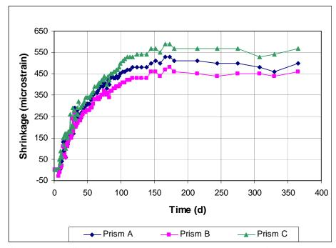
Figure A3.46 - Free Shrinkage, Batch 166, 7-day cure. 70% Aggregate, 0.45 w/c. Type II coarse ground (CG) cement. Drying begins at 7 days.
