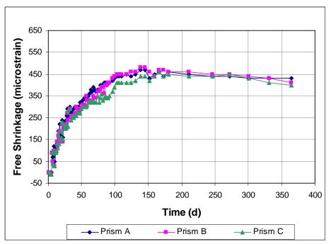
Figure A3.57 - Free Shrinkage, Batch 167. 75% Aggregate, 0.45 w/c. Type I/II cement. Drying begins at 3 days. Control, no chemical admixtures.
