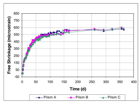
Figure A3.8 - Free Shrinkage, Batch 69. 60% Aggregate, 0.45 w/c., Type I/II cement. Drying begins on day 3.
