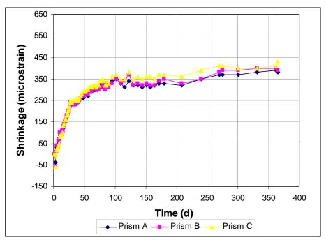
Figure A3.23 - Free Shrinkage, Batch 189. 70% Aggregate, 0.45 w/c. Type I/II cement. Drying begins at 3 days. Granite.
