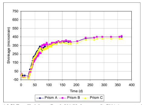
Figure A3.52 Free Shrinkage, Batch 201(28-days-cured), 70% Aggregate, 0.45 w/c ratio, Type I/II Cement. Drying begins at 28 days.
