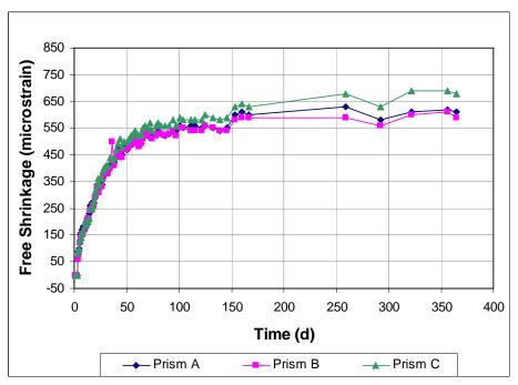
Figure A3.9- Free Shrinkage, Batch 70. 60% Aggregate, 0.50 w/c. Type I/II cement. Drying begins on day 3.
