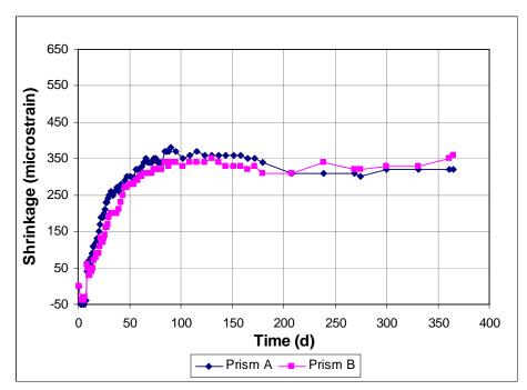
Figure A3.71 - Free Shrinkage, Batch 181. 75% Aggregate, 0.45 w/c. Type I/II cement. Drying begins at 3 days. High dosage of Rheobuild 1000.
