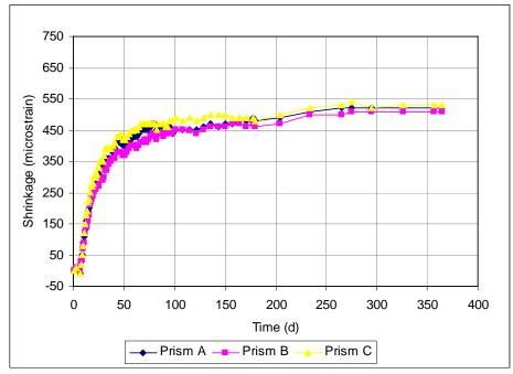
Figure A3.50 Free Shrinkage, Batch 201(7-days-cured), 70% Aggregate, 0.45 w/c ratio, Type I/II Cement. Drying begins at 7 days.
