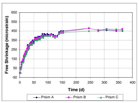
Figure A3.17 - Free Shrinkage, Batch 78. 60% Aggregate, 0.45 w/c. Type II coarse ground (CG) cement. Drying begins on day 3.
