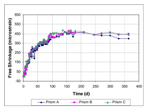
Figure A3.61 - Free Shrinkage, Batch 171. 75% Aggregate, 0.45 w/c. Type I/II cement. Drying begins at 3 days. Low dosage of Rheobuild 1000.
