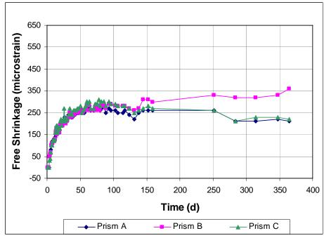
Figure A3.10 - Free Shrinkage, Batch 71. 80% Aggregate, 0.40 w/c. Type II coarse ground (CG) cement. Drying begins on day 3.
