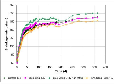
Figure 3.30 Free Shrinkage Test, Program III. Comparing mineral admixtures through 365 days.
