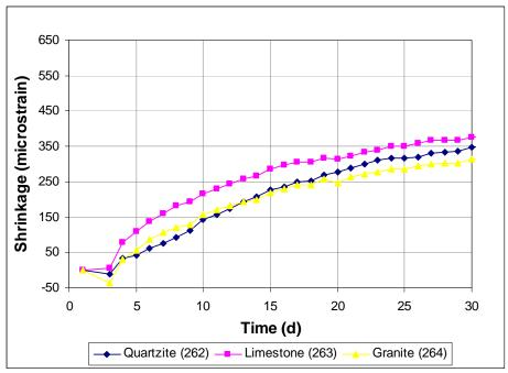
Figure 3.22 Free Shrinkage Test, Program II. Comparison of different aggregate types through 30 days.
