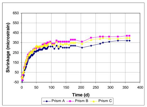
Figure A3.77 - Free Shrinkage, Batch 190. 75% Aggregate, 0.45 w/c. Type I/II cement. Drying begins at 3 days. Low dosage of Adva 100.
