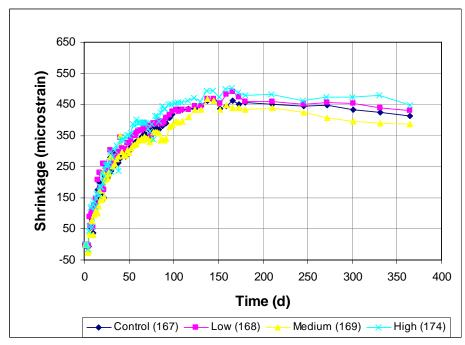
Figure 3.68 Free Shrinkage Test, Program V. Average free shrinkage vs. time. Comparing different dosages of Glenium 3000 NS through 365 days.
