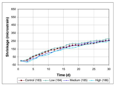
Figure 3.78 Free Shrinkage Test, Program V. Average free shrinkage vs. time. Comparing different dosages of Adva 100 through 30 days.
