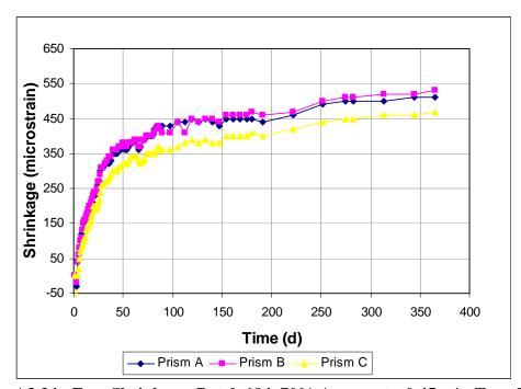
Figure A3.34 - Free Shrinkage, Batch 194. 70% Aggregate, 0.45 w/c. Type I/II cement. Drying begins at 3 days. Control, no mineral admixtures.
