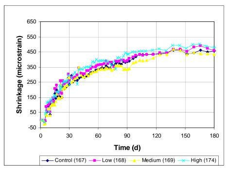
Figure 3.67 Free Shrinkage Test, Program V. Average free shrinkage vs. time. Comparing different dosages of Glenium 3000 NS through 180 days.
