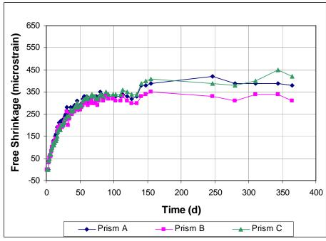
Figure A3.14 - Free Shrinkage, Batch 75. 70% Aggregate, 0.45 w/c. Type II coarse ground (CG) cement. Drying begins on day 3.
