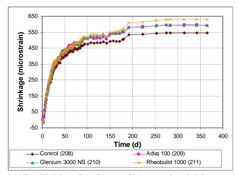
Figure 3.86 Free Shrinkage Test, Program V. Average free shrinkage vs. time. Comparing different Superplasticizers (Dosages for same slump) through 365 days.
