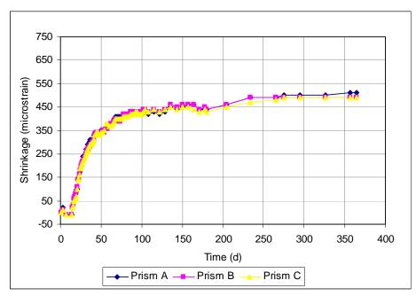
Figure A3.51 Free Shrinkage, Batch 201(14-days-cured), 70% Aggregate, 0.45 w/c ratio, Type I/II Cement. Drying begins at 14 days.
