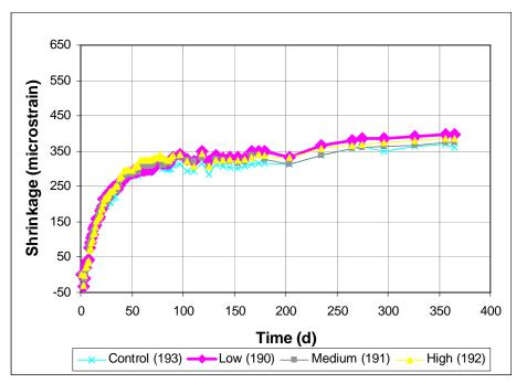
Figure 3.83 Free Shrinkage Test, Program V. Average free shrinkage vs. time. Comparing different dosages of Adva 100 through 365 days.
