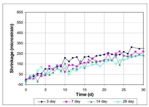
Figure 3.41 - Free Shrinkage, Program IV. Average free shrinkage vs. time for different curing times. Batch 166. Type II coarse ground (CG) cement through 30 days. Drying only.
