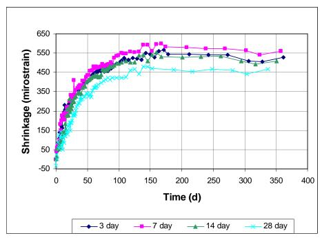
Figure 3.39 - Free Shrinkage, Program IV. Average free shrinkage vs. time for different curing times. Batch 165. Type I/II cement through 365 days. Drying only.
