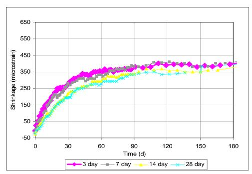
Figure 3.55 - Free Shrinkage, Program IV. Average free shrinkage vs. time for different curing times. Type II coarse ground (CG) cement. Batch 207 through 180 days. Drying only.
