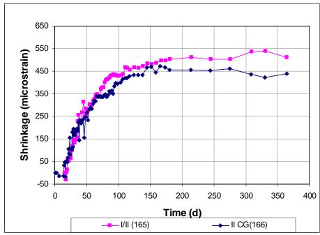
Figure 3.60 - Free Shrinkage, Program IV. Average free shrinkage vs. time for 14-day cure specimens. Comparing cement type through 365 days.
