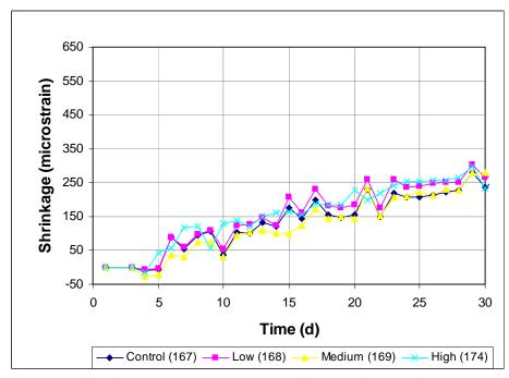
Figure 3.66 Free Shrinkage Test, Program V. Average free shrinkage vs. time. Comparing different dosages of Glenium 3000 NS through 30 days.
