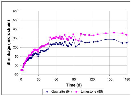
Figure 3.14 Free Shrinkage Test, Program II. Comparison of different aggregate types through 180 days.
