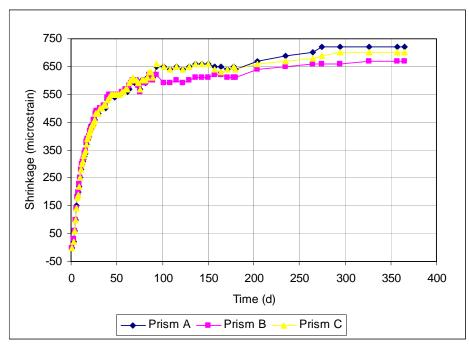
Figure A3.49 Free Shrinkage, Batch 201(3-days-cured), 70% Aggregate, 0.45 w/c ratio, Type I/II Cement. Drying begins at 3 days.
