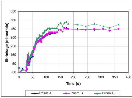
Figure A3.44 - Free Shrinkage, Batch 165, 28-day cure. 70% Aggregate, 0.45 w/c. Type I/II cement. Drying begins at 28 days.
