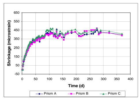
Figure A3.30 - Free Shrinkage, Batch 85. 70% Aggregate, 0.45 w/c. Type I/II cement. Drying begins at 3 days. Control, no mineral admixtures.
