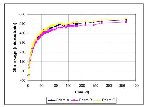
Figure A3.28 - Free Shrinkage, Batch 263. 68.8% Aggregate, 0.45 w/c. Type I/II cement. Air-entrained concrete. Drying begins at 3 days. Limestone.
