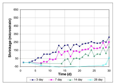
Figure 3.40 - Free Shrinkage, Program IV. Average free shrinkage vs. time for different curing times. Batch 166 through 30 days. Type II coarse ground (CG) cement.
