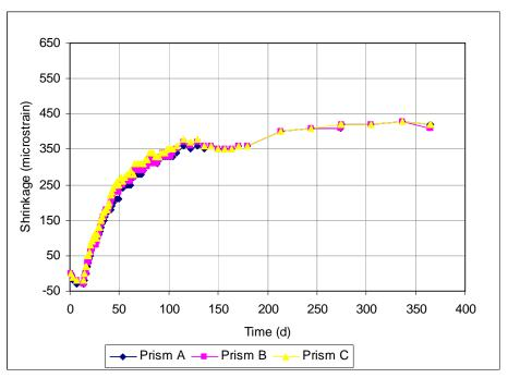
Figure A3.55 Free Shrinkage, Batch 207(14-days-cured), 70% Aggregate, 0.45 w/c ratio, Type II coarse ground (CG) cement. Drying begins at 14 days.
