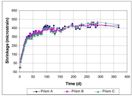
Figure A3.32 - Free Shrinkage, Batch 87. 70% Aggregate, 0.45 w/c. Type I/II cement. Drying begins at 3 days. 30% Class C Fly Ash replacement.
