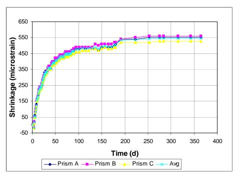
Figure A3.81 - Free Shrinkage, Batch 208. 70% Aggregate, 0.45 w/c. Type I/II cement. Drying begins at 3 days. Control, no chemical admixtures.
