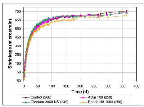
Figure 3.89 Free Shrinkage Test, Program V. Average free shrinkage vs. time. Comparing different Superplasticizers (Dosages for same slump) through 365 days.
