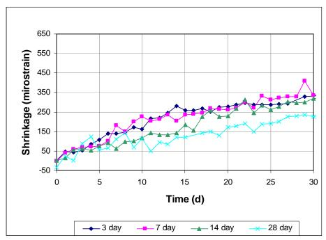
Figure 3.35 - Free Shrinkage, Program IV. Average free shrinkage vs. time for different curing times. Batch 165. Type I/II cement through 30 days. Drying only.
