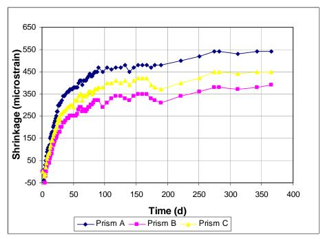
Figure A3.37 - Free Shrinkage, Batch 197. 70% Aggregate, 0.45 w/c. Type I/II cement. Drying begins at 3 days. 10% Replacement by Silica Fume.
