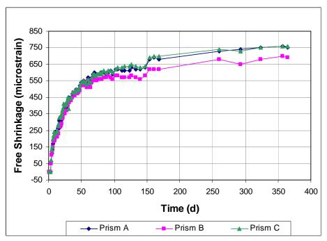
Figure A3.7 - Free Shrinkage, Batch 68. 60% Aggregate, 0.40 w/c. Type I/II cement. Drying begins on day 3.
