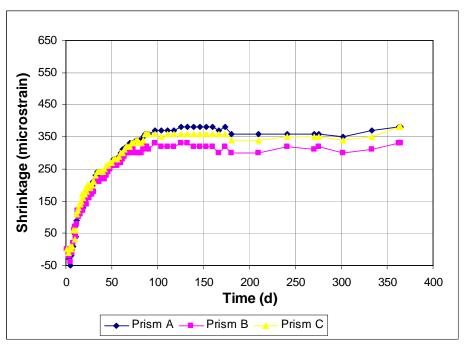
Figure A3.65 - Free Shrinkage, Batch 175. 75% Aggregate, 0.45 w/c. Type I/II cement. Drying begins at 3 days. Control, no chemical admixtures.
