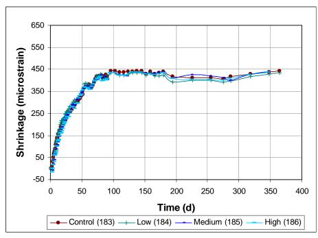
Figure 3.80 Free Shrinkage Test, Program V. Average free shrinkage vs. time. Comparing different dosages of Adva 100 through 365 days.
