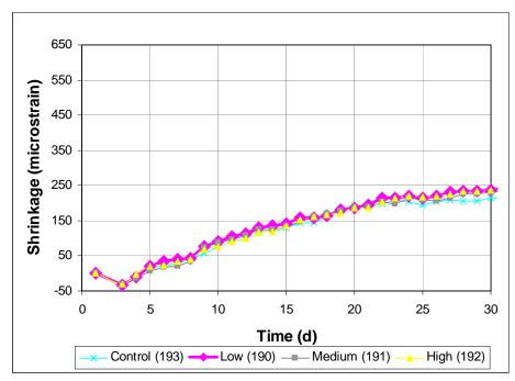
Figure 3.81 Free Shrinkage Test, Program V. Average free shrinkage vs. time. Comparing different dosages of Adva 100 through 30 days.
