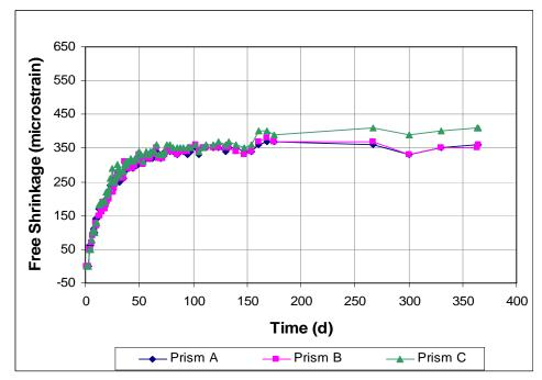
Figure A3.2 - Free Shrinkage, Batch 63. 80% Aggregate, 0.45 w/c. Type I/II cement. Drying begins at 3 days.
