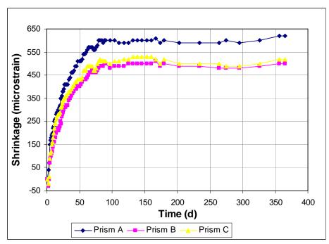
Figure A3.72 - Free Shrinkage, Batch 182. 75% Aggregate, 0.45 w/c. Type I/II cement. Drying begins at 3 days. High dosage of Rheobuild 1000.
