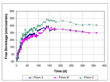
Figure A3.59 - Free Shrinkage, Batch 169. 75% Aggregate, 0.45 w/c. Type I/II cement. Drying begins at 3 days. Medium dosage of Glenium 3000NS.
