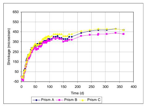
Figure A3.54 Free Shrinkage, Batch 207(7-days-cured), 70% Aggregate, 0.45 w/c ratio, Type II coarse ground (CG) cement. Drying begins at 7 days.
