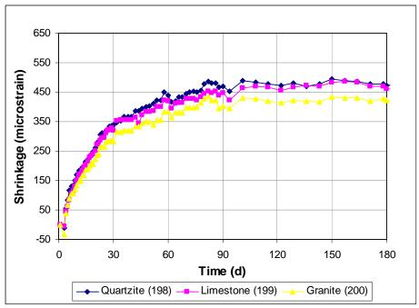
Figure 3.20 Free Shrinkage Test, Program II. Comparison of different aggregate types through 180 days.
