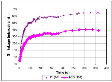
Figure 3.62 - Free Shrinkage, Program IV. Average free shrinkage vs. time for 3-day cure specimens. Comparing cement type through 365 days.
