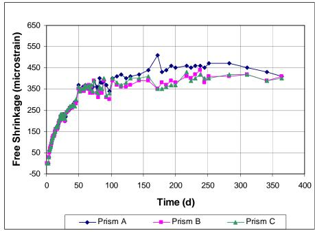
Figure A3.20 - Free Shrinkage, Batch 95. 70% Aggregate, 0.45 w/c. Type I/II cement. Drying begins at 3 days. Limestone.
