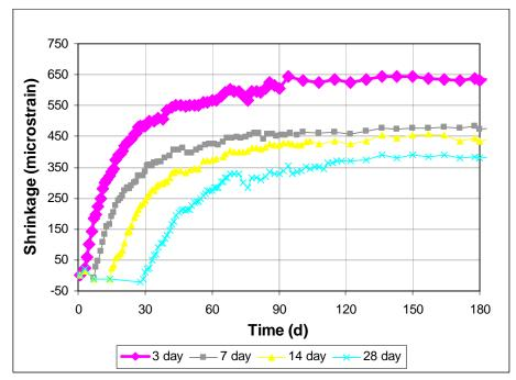
Figure 3.48 - Free Shrinkage, Program IV. Average free shrinkage vs. time for different curing times. Type I/II cement. Batch 201 through 180 days.
