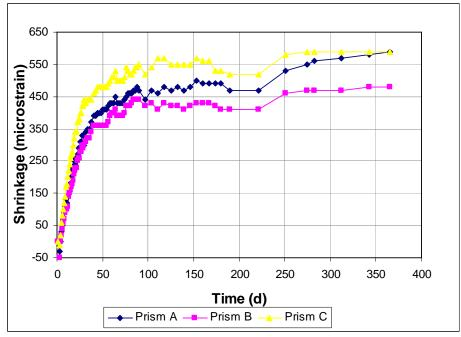
Figure A3.36 - Free Shrinkage, Batch 196. 70% Aggregate, 0.45 w/c. Type I/II cement. Drying begins at 3 days. 30% Replacement by Class C Fly Ash.
