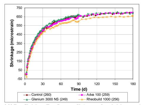
Figure 3.88 Free Shrinkage Test, Program V. Average free shrinkage vs. time. Comparing different Superplasticizers (Dosages for same slump) through 180 days.
