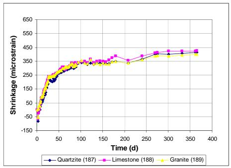
Figure 3.18 Free Shrinkage Test, Program II. Comparison of different aggregate types through 365 days.
