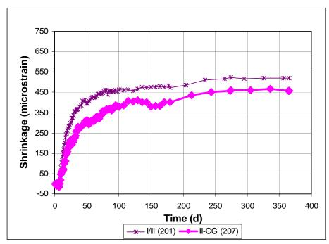
Figure 3.63 - Free Shrinkage, Program IV. Average free shrinkage vs. time for 7-day cure specimens. Comparing cement type through 365 days.
