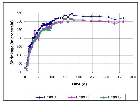
Figure A3.42 - Free Shrinkage, Batch 165, 7-day cure. 70% Aggregate, 0.45 w/c. Type I/II cement. Drying begins at 7 days.
