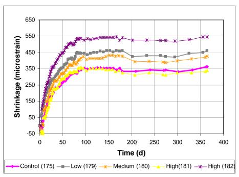
Figure 3.77 Free Shrinkage Test, Program V. Average free shrinkage vs. time. Comparing different dosages of Rheobuild 1000 through 365 days.
