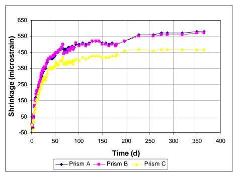
Figure A3.38 - Free Shrinkage, Batch 202. 70% Aggregate, 0.45 w/c. Type I/II cement. Drying begins at 3 days. Control, no mineral admixtures.
