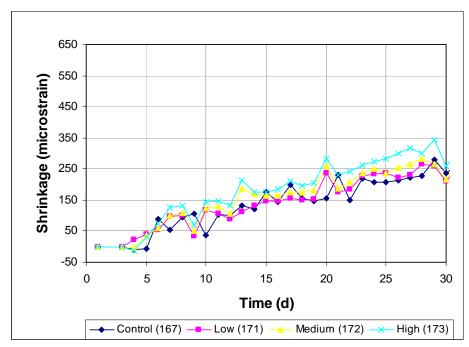
Figure 3.69 Free Shrinkage Test, Program V. Average free shrinkage vs. time. Comparing different dosages of Rheobuild 1000 through 30 days.
