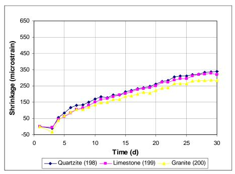
Figure 3.19 Free Shrinkage Test, Program II. Comparison of different aggregate types through 30 days.
