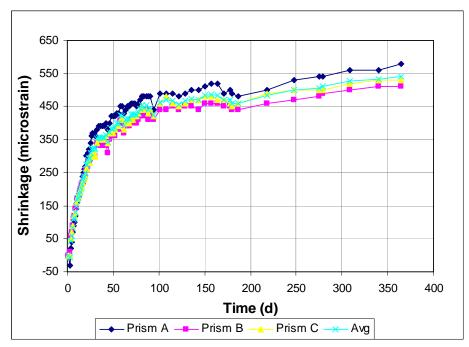
Figure A3.25 - Free Shrinkage, Batch 199. 70% Aggregate, 0.45 w/c. Type I/II cement. Drying begins at 3 days. Limestone.
