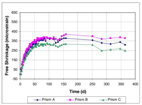
Figure A3.13 - Free Shrinkage, Batch 74. 70% Aggregate, 0.40 w/c. Type II CG cement. Drying begins on day 3.
