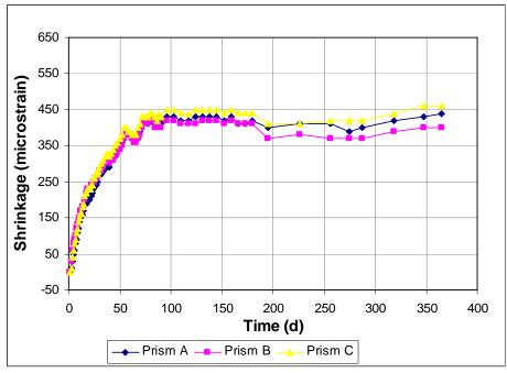
Figure A3.74 - Free Shrinkage, Batch 184. 75% Aggregate, 0.45 w/c. Type I/II cement. Drying begins at 3 days. Low dosage of Adva 100.
