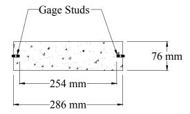
Figure 2.2 – Cross-section of Free Shrinkage Specimen (Tritsch 2005)
