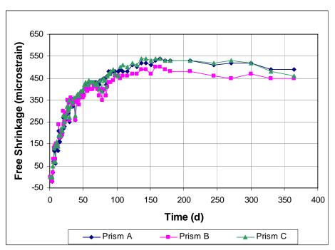
Figure A3.63 - Free Shrinkage, Batch 173. 75% Aggregate, 0.45 w/c. Type I/II cement. Drying begins at 3 days. High dosage of Rheobuild 1000.
