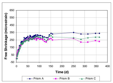
Figure A3.11 - Free Shrinkage, Batch 72. 80% Aggregate, 0.45 w/c. Type II coarse ground (CG) cement. Drying begins on day 3.
