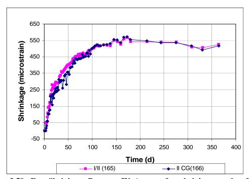
Figure 3.58 - Free Shrinkage, Program IV. Average free shrinkage vs. time for 3-day cure specimens. Comparing cement type through 365 days.
