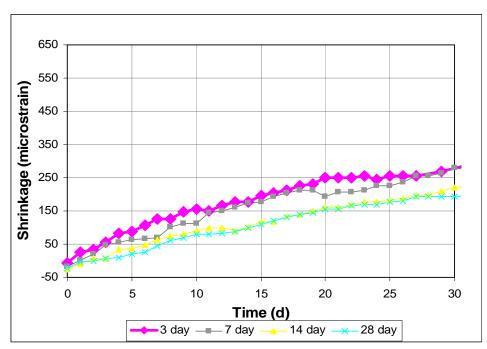
Figure 3.53 - Free Shrinkage, Program IV. Average free shrinkage vs. time for different curing times. Type II coarse ground (CG) cement. Batch 207 through 30 days. Drying only.
