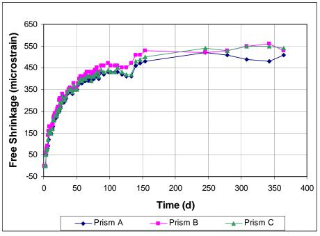
Figure A3.16 - Free Shrinkage, Batch 77. 60% Aggregate, 0.40 w/c. Type II coarse ground (CG) cement. Drying begins on day 3.
