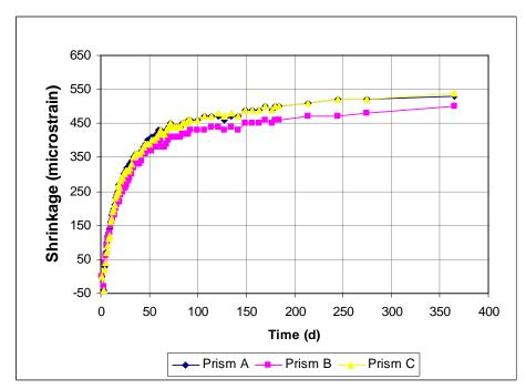
Figure A3.29 - Free Shrinkage, Batch 264. 68.8% Aggregate, 0.45 w/c., Type I/II cement. Air-entrained concrete. Drying begins at 3 days. Granite.
