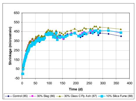
Figure 3.27 Free Shrinkage Test, Program III. Comparing mineral admixtures through 365 days.
