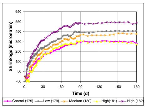
Figure 3.76 Free Shrinkage Test, Program V. Average free shrinkage vs. time. Comparing different dosages of Rheobuild 1000 through 180 days.
