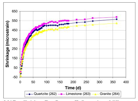
Figure 3.24 Free Shrinkage Test, Program II. Comparison of different aggregate types through 365 days.
