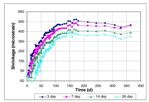
Figure 3.44 - Free Shrinkage, Program IV. Average free shrinkage vs. time for different curing times. Batch 166 through 365 days. Type II coarse ground (CG) cement.
