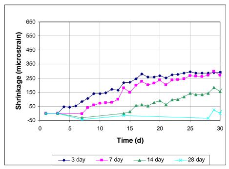
Figure 3.34 - Free Shrinkage, Program IV. Average free shrinkage vs. time for different curing times. Batch 165. Type I/II cement through 30 days.
