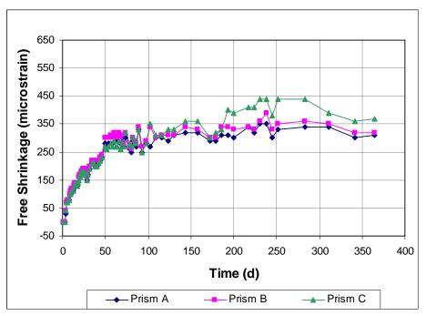
Figure A3.19 - Free Shrinkage, Batch 94. 70% Aggregate, 0.45 w/c. Type I/II cement. Drying begins at 3 days. Quartzite.
