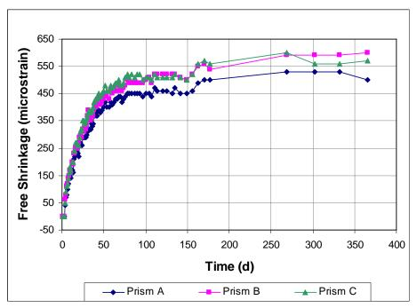
Figure A3.3 - Free Shrinkage, Batch 64. 70% Aggregate, 0.45 w/c. Type I/II cement. Drying begins at 3 days.
