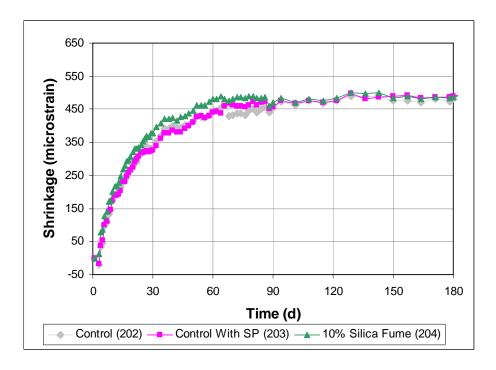
Figure 3.32 Free Shrinkage Test, Program III. Comparing Silica Fume and controls through 180 days.
