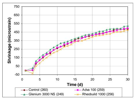
Figure 3.87 Free Shrinkage Test, Program V. Average free shrinkage vs. time. Comparing different Superplasticizers (Dosages for same slump) through 30 days.
