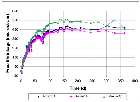
Figure A3.64 - Free Shrinkage, Batch 174. 75% Aggregate, 0.45 w/c. Type I/II cement. Drying begins at 3 days. High dosage of Glenium 3000NS.
