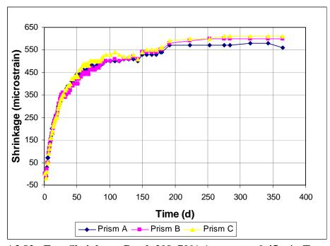
Figure A3.82 - Free Shrinkage, Batch 209. 70% Aggregate, 0.45 w/c. Type I/II cement. Drying begins at 3 days, Adva 100.
