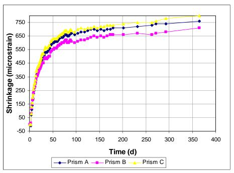
Figure A3.85 - Free Shrinkage, Batch 260. 63.5% Aggregate, 0.45 w/c. Type I/II cement. Air-entrained concrete. Drying begins at 3 days. Control, no superplasticizer, increased paste content for same slump.
