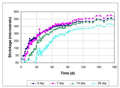
Figure 3.36 - Free Shrinkage, Program IV. Average free shrinkage vs. time for different curing times. Batch 165. Type I/II cement through 180 days.
