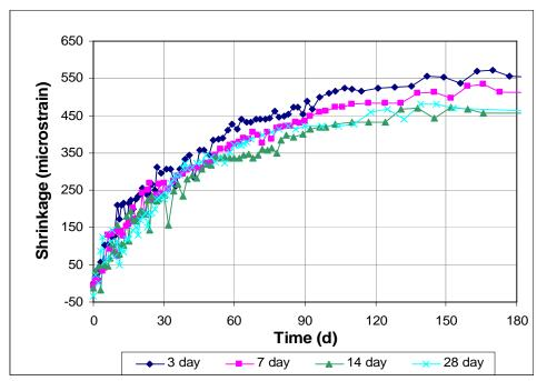
Figure 3.43 - Free Shrinkage, Program IV. Average free shrinkage vs. time for different curing times. Batch 166. Type II coarse ground (CG) cement through 180 days. Drying only.
