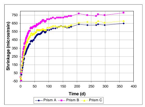
Figure A3.87 - Free Shrinkage, Batch 256. 67.8% Aggregate, 0.45 w/c. Type I/II cement. Air-entrained concrete. Drying begins at 3 days. Rheobuild 1000.
