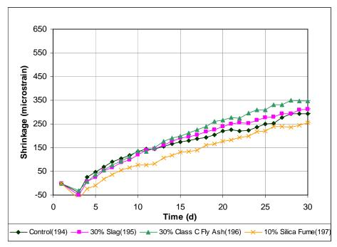
Figure 3.28 Free Shrinkage Test, Program III. Comparing mineral admixtures through 30 days.
