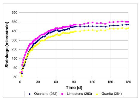
Figure 3.23 Free Shrinkage Test, Program II. Comparison of different aggregate type through 180 days.
