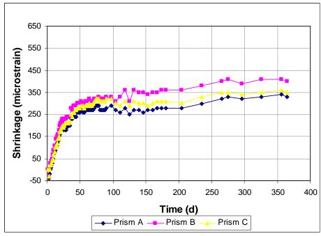
Figure A3.80 - Free Shrinkage, Batch 193. 75% Aggregate, 0.45 w/c. Type I/II cement. Drying begins at 3 days. Control, no chemical admixture.
