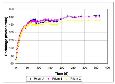
Figure A3.40 - Free Shrinkage, Batch 204. 70% Aggregate, 0.45 w/c. Type I/II cement. Drying begins at 3 days. 10% Replacement by Silica Fume. Adva superplasticizer.
