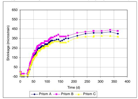
Figure A3.56 Free Shrinkage, Batch 207(28-days-cured), 70% Aggregate, 0.45 w/c ratio, Type II coarse ground (CG) cement. Drying begins at 28 days.
