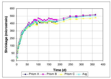
Figure A3.24 - Free Shrinkage, Batch 198. 70% Aggregate, 0.45 w/c. Type I/II cement. Drying begins at 3 days. Quartzite.
