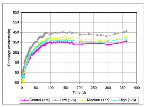
Figure 3.74 Free Shrinkage Test, Program V. Average free shrinkage vs. time. Comparing different dosages of Glenium 3000 NS through 365 days.
