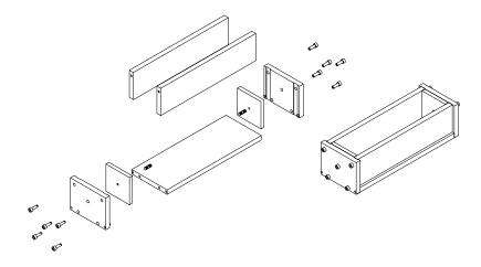
Figure 2.1 – Free Shrinkage Specimen Mold (Tritsch 2005)
