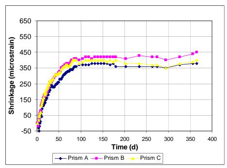
Figure A3.66 - Free Shrinkage, Batch 176. 75% Aggregate, 0.45 w/c. Type I/II cement. Drying begins at 3 days. Low dosage of Glenium 3000NS.
