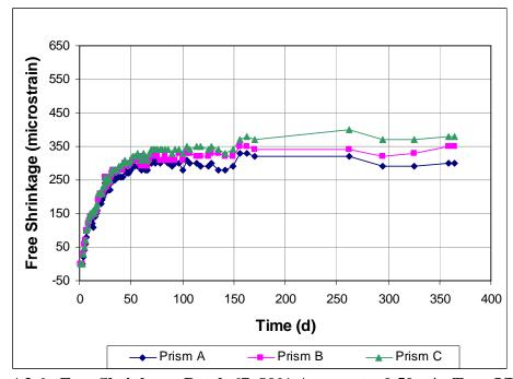
Figure A3.6 - Free Shrinkage, Batch 67. 80% Aggregate, 0.50 w/c. Type I/II cement. Drying begins on day 3.
