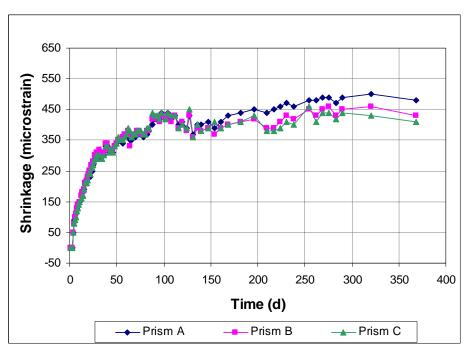
Figure A3.33 - Free Shrinkage, Batch 88. 70% Aggregate, 0.45 w/c. Type I/II cement. Drying begins at 3 days. 10% silica fume replacement.
