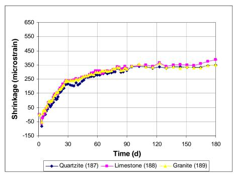
Figure 3.17 Free Shrinkage Test, Program II. Comparison of different aggregate types through 180 days.
