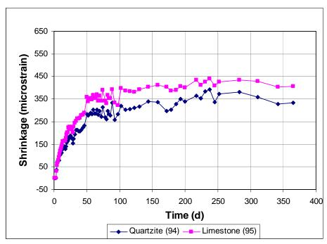
Figure 3.15 Free Shrinkage Test, Program II. Comparison of different aggregate types through 365 days.
