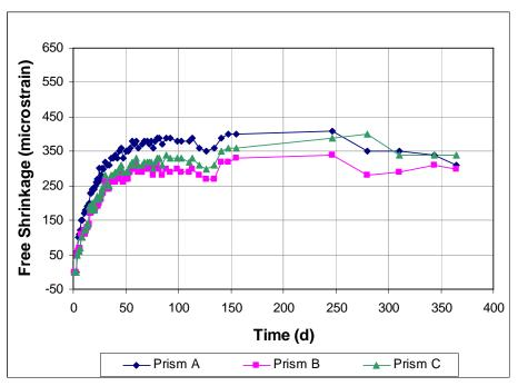
Figure A3.15 - Free Shrinkage, Batch 76. 70% Aggregate, 0.50 w/c. Type II coarse ground (CG) cement. Drying begins on day 3.
