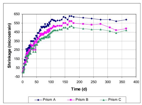
Figure A3.45 - Free Shrinkage, Batch 166, 3-day cure. 70% Aggregate, 0.45 w/c. Type II coarse ground (CG) cement. Drying begins at 3 days.
