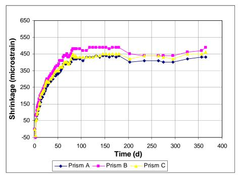
Figure A3.69 - Free Shrinkage, Batch 179. 75% Aggregate, 0.45 w/c. Type I/II cement. Drying begins at 3 days. Low dosage of Rheobuild 1000.
