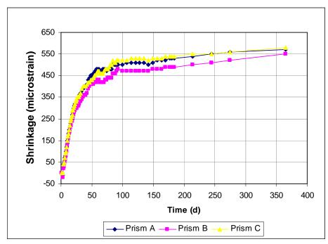
Figure A3.27 - Free Shrinkage, Batch 262. 68.8% Aggregate, 0.45 w/c. Type I/II cement. Air-entrained concrete. Drying begins at 3 days. Quartzite.
