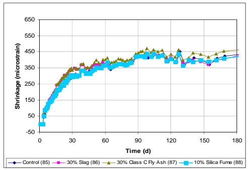
Figure 3.26 Free Shrinkage Test, Program III. Comparing mineral admixtures through 180 days.
