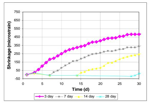
Figure 3.46 - Free Shrinkage, Program IV. Average free shrinkage vs. time for different curing times. Type I/II cement. Batch 201 through 30 days.
