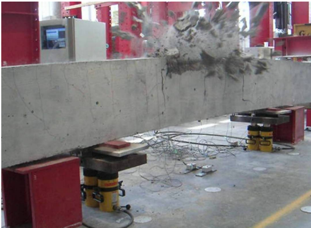
Figure 4: Typical failure of specimens with unconfined spliced bars (NCSU)
