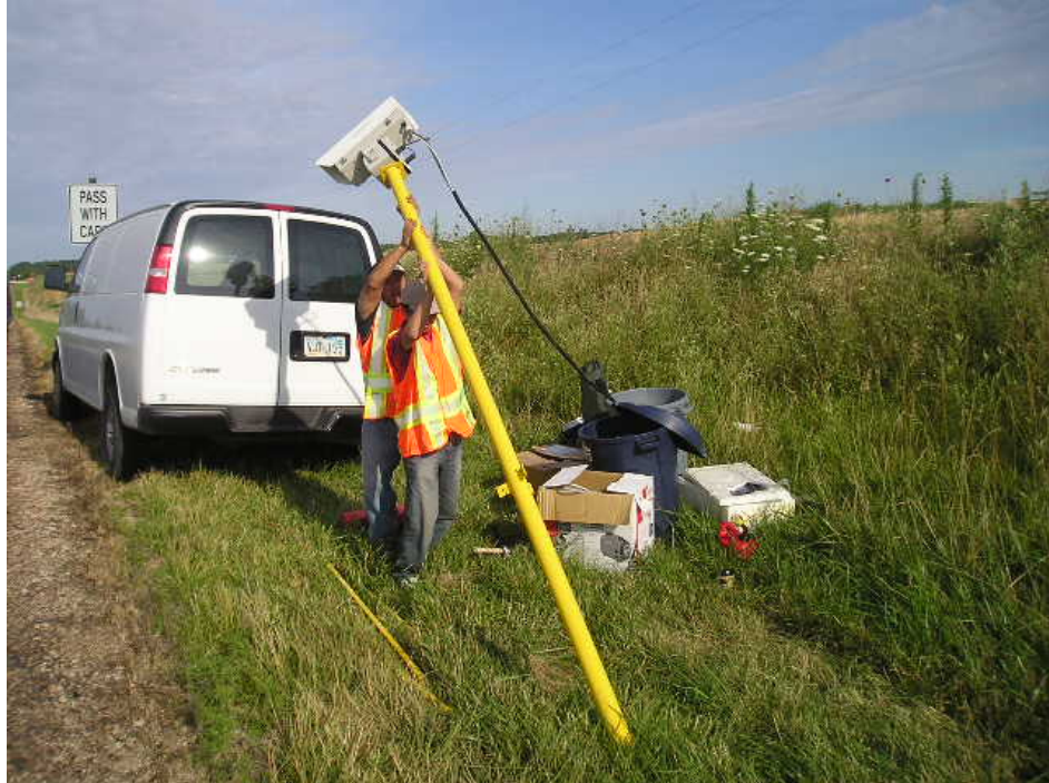
Fig. 14. Erecting the pole perpendicular to the ground
