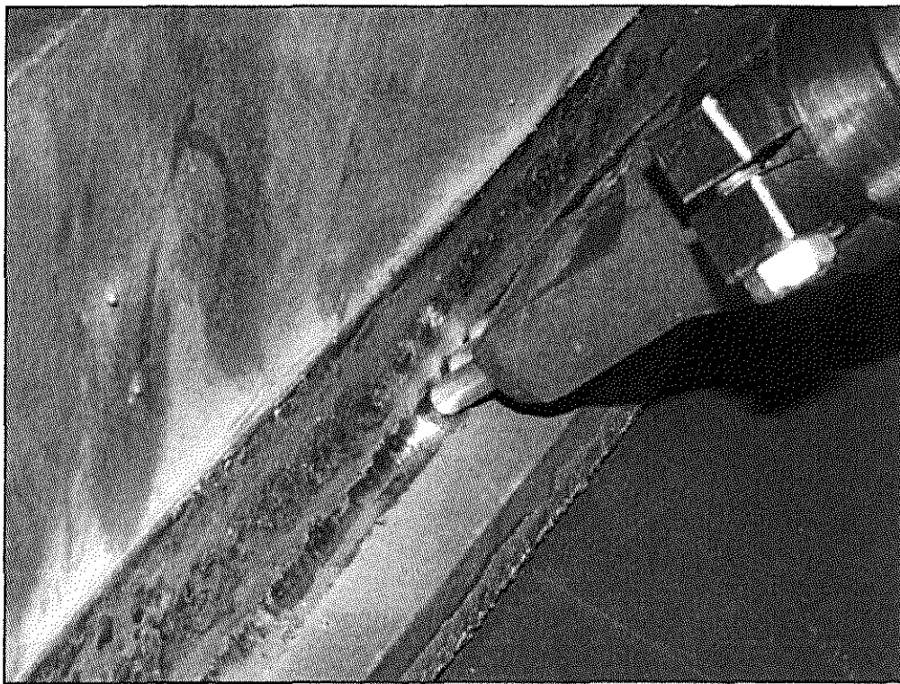
Figure 2.4. UIT needle configuration and the treated surface (Lihavainen et al. 2003).
