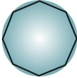
Figure 2.3. Schematic illustrating continuous TIR events within a spherical microcavity. Recirculation of a particular wavelength within the cavity achieves a whispering gallery mode resonance.
