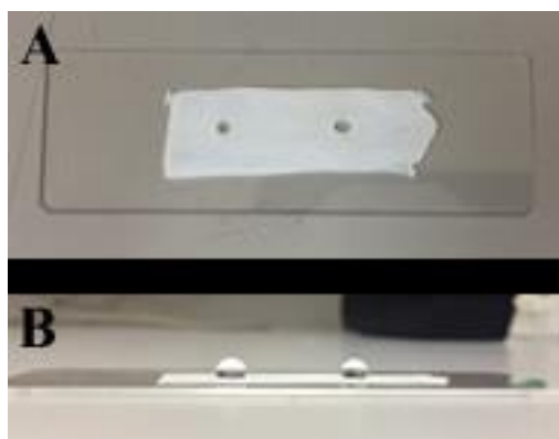
Figure 4.2. Images of Teflon tape on a glass microscope slide to support aqueous droplet formation in air. (A) The Teflon tape was firmly adhered to the microscope slide using heat and pressure. (B) A side view shows the formation of aqueous droplets ( \sim 10\text{ }\mu\text{L} ) on the surface due to the hydrophobic boundary created by the Teflon tape.
