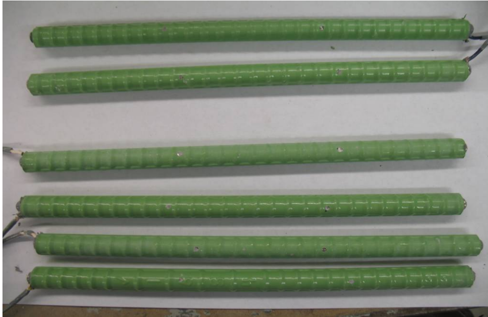
Figure 3.136 – Top and bottom bars of the ECR-4h-45-5 specimen at autopsy (before disbondment test). Top bars are shown at the top of the figure and bottom bars are show at the bottom of the figure.
