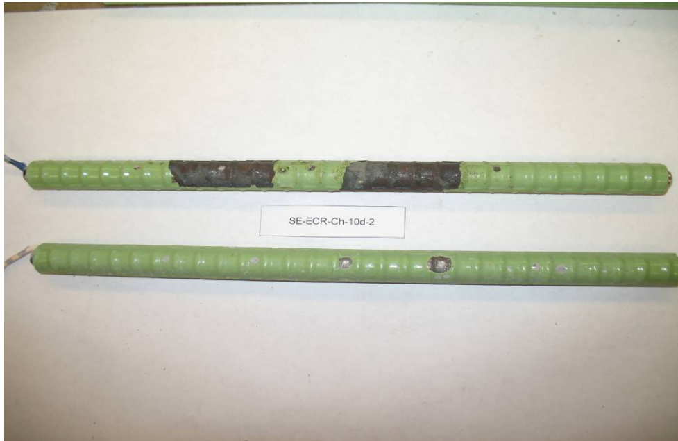
Figure 3.138 – Top bars of the ECR(Chromate)-10h-45-2 specimen at autopsy (after disbondment test).
