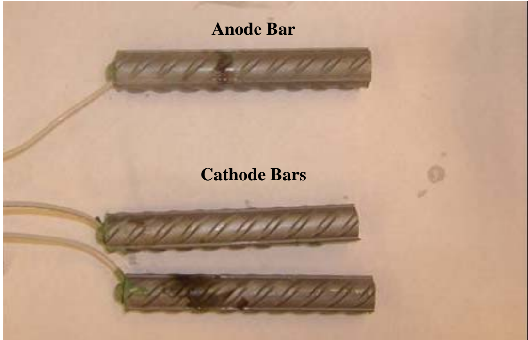
Figure A23: LDX 2101® specimen 1, submerged in simulated pore solution prior to testing. Side A.
