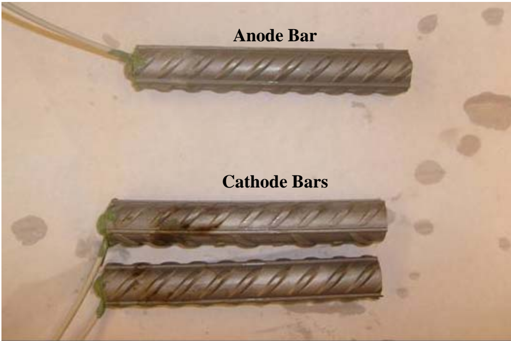
Figure A27: LDX 2101® specimen 3, submerged in simulated pore solution prior to testing. Side A.
