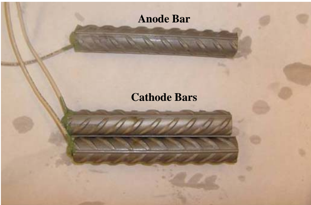
Figure A28: LDX 2101® specimen 3, submerged in simulated pore solution prior to testing. Side B.
