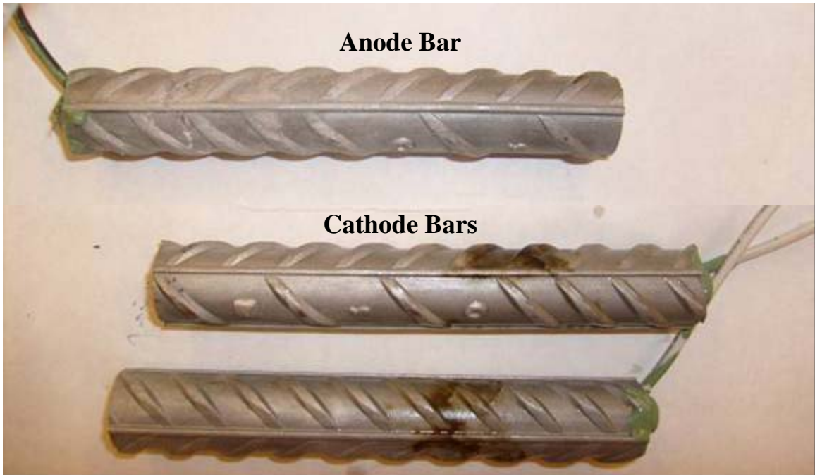
Figure A4: LDX 2101® specimen 2, as received condition. Side B
