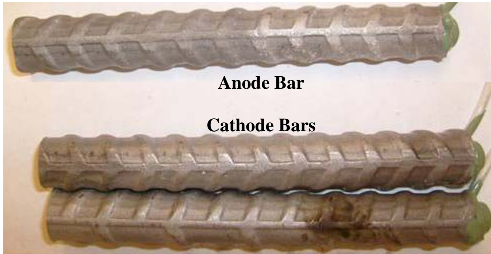
Figure 21: 2205p specimen 3 showing staining at end of test.
