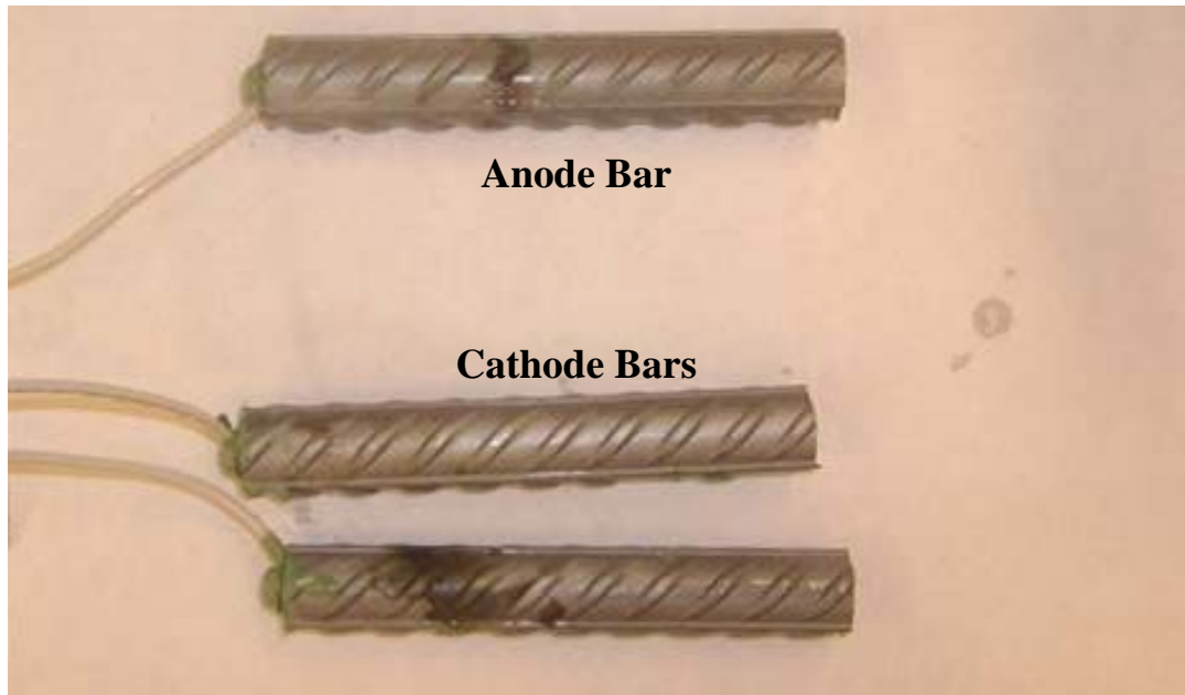
Figure 19: LDX 2101® specimen 1, submerged in simulated pore solution prior to testing. Bars at end of test showing staining.
