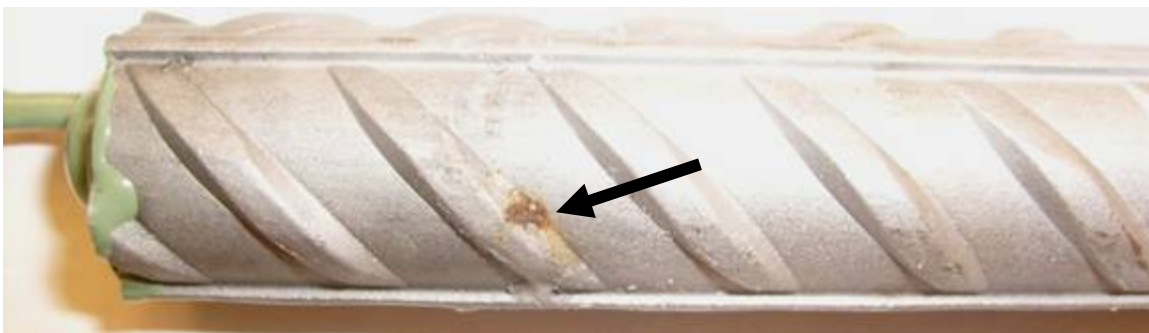
Figure 18: LDX 2101® specimen 6, as received condition. Anode bar at end of test. Limited staining on bar in salt solution.
