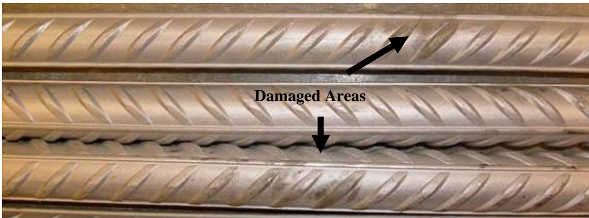
Figure 1: Damage to stainless steel sustained during shipping.
