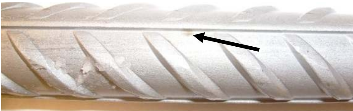
Figure 20: LDX 2101® specimen 2, submerged in simulated pore solution prior to testing. Anode bar at end of test. Limited staining on bar in salt solution.
