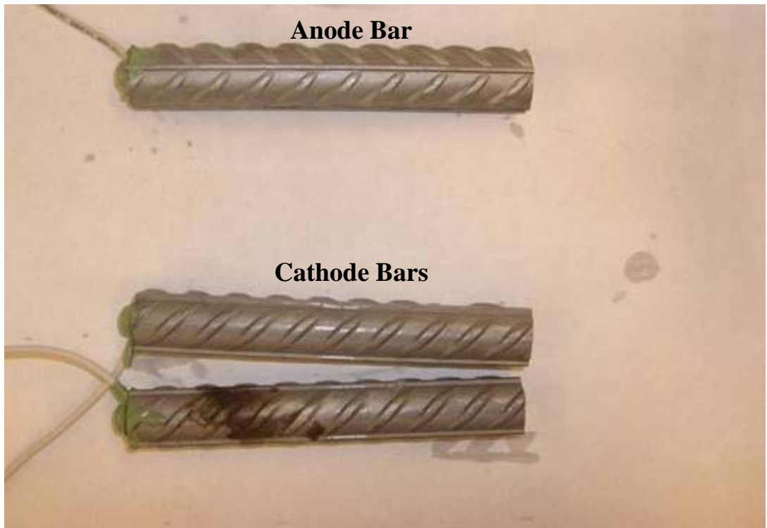
Figure A24: LDX 2101® specimen 1, submerged in simulated pore solution prior to testing. Side B.
