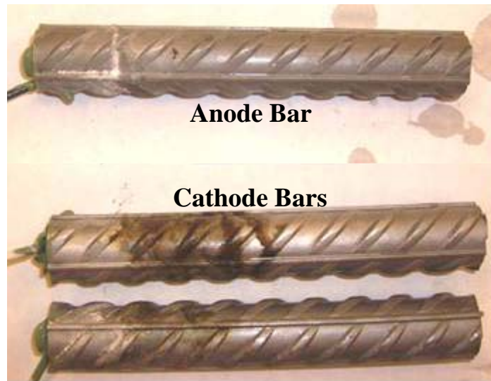
Figure 17: LDX 2101® specimen 3, as received condition. Bars at end of test showing staining.
