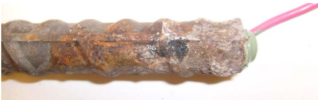
Figure 8: Specimen 4 (opposite site from that shown in Figure 7) one week after removal from solution. Significant corrosion appears on the top third of the anode bar.
