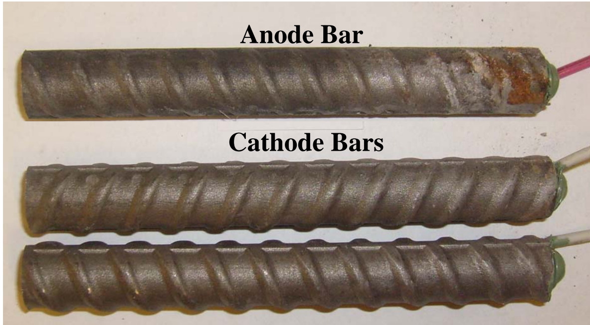
Figure 10: Specimen 3 one week after removal from solution, prior to brushing.
