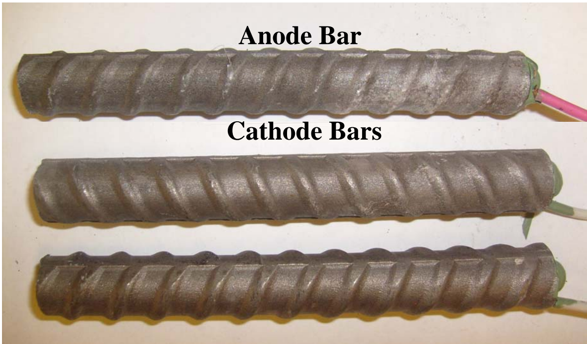
Figure A.6b: Specimen 3, Side B, eight days after removal from solution.
