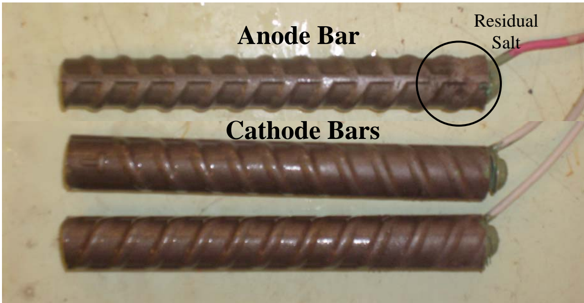
Figure A.11a: Specimen 6, Side A, immediately after removal from solution.
