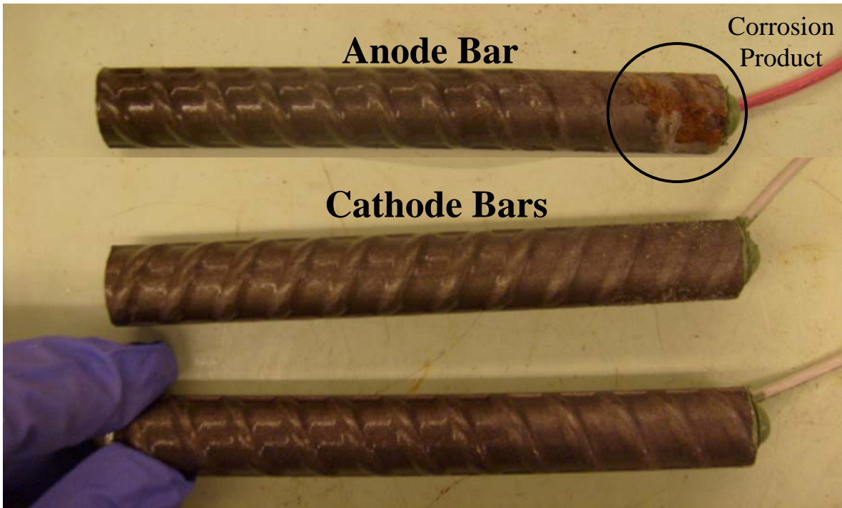
Figure A.5a: Specimen 3, Side A, immediately after removal from solution.
