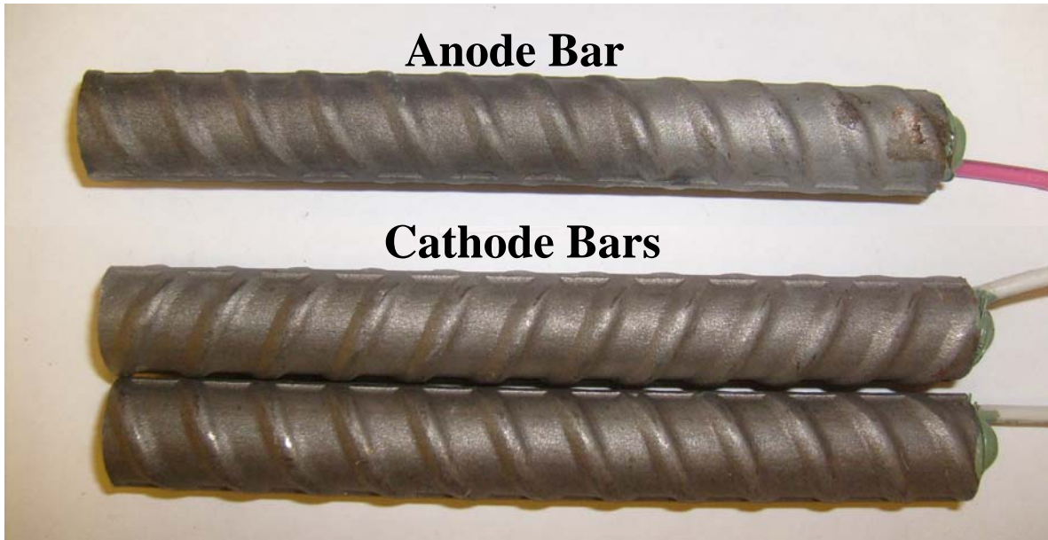
Figure 12: Specimen 3 one week after removal from solution, after brushing. Moderate corrosion occurred at the top of the bar.
