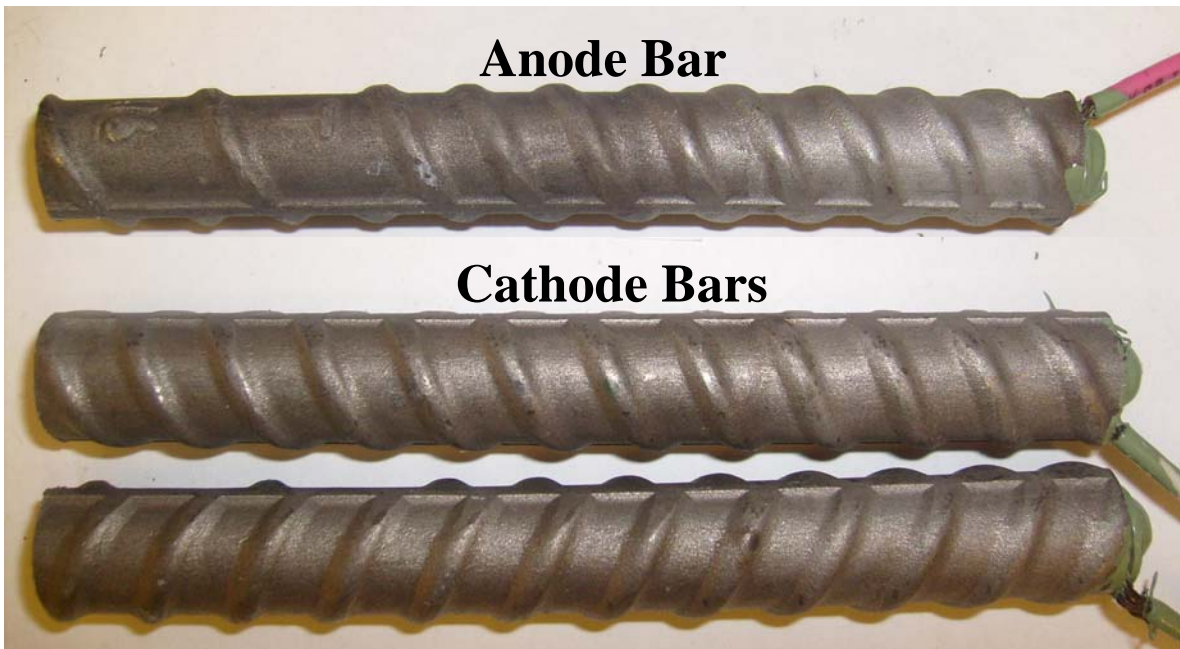
Figure A.9c: Specimen 5, Side A, eight days after removal from solution, after brushing.
