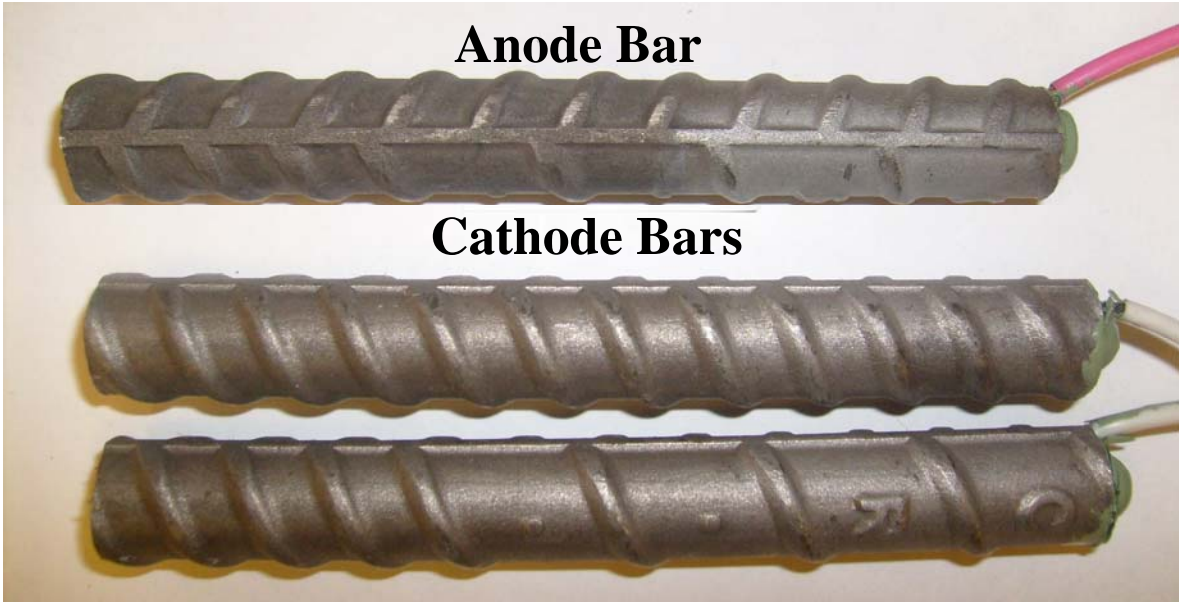
Figure A.3c: Specimen 2, Side A, eight days after removal from solution, after brushing.
