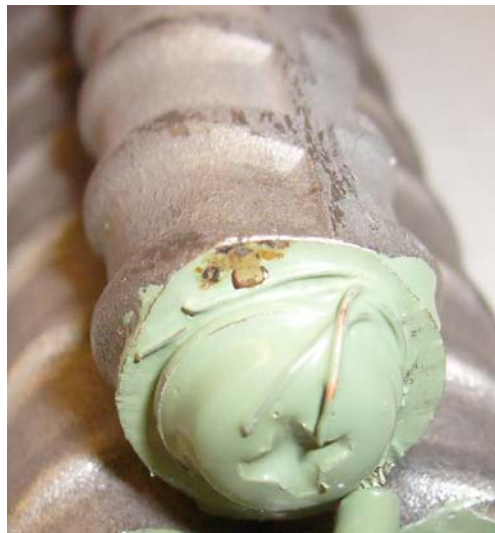
Figure 13: Specimen 5 anode one week after removal from solution, after brushing.
