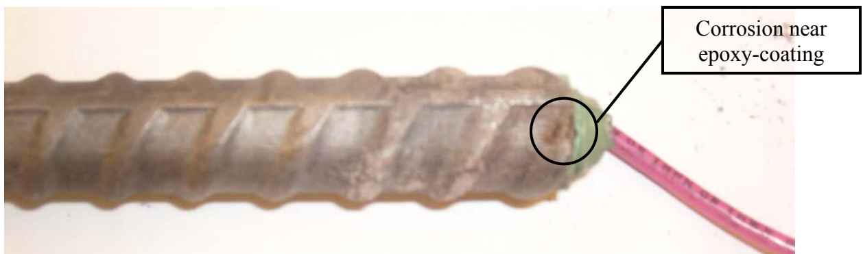
Figure 11: Specimen 5 anode one week after removal from solution, prior to brushing.
