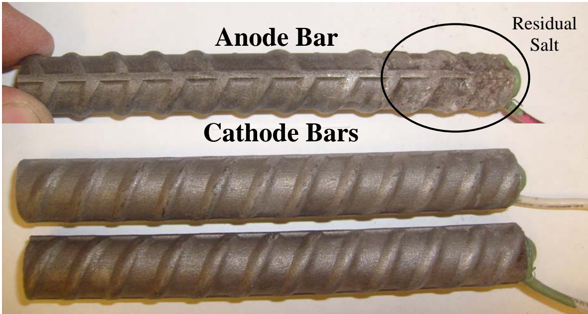
Figure A.4b: Specimen 2, Side B, eight days after removal from solution.
