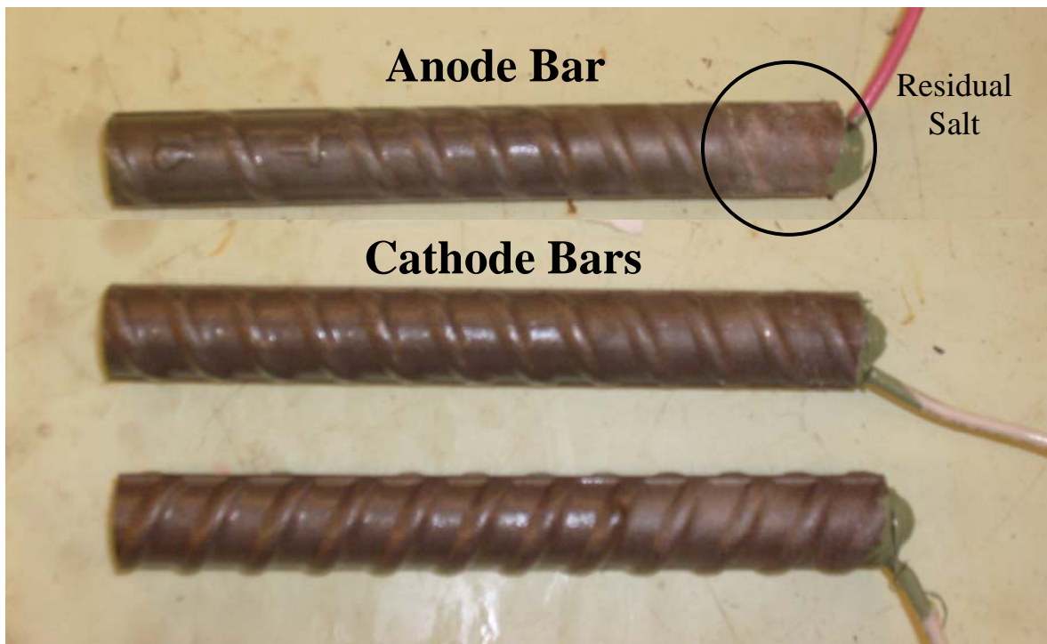
Figure A.9a: Specimen 5, Side A, immediately after removal from solution.
