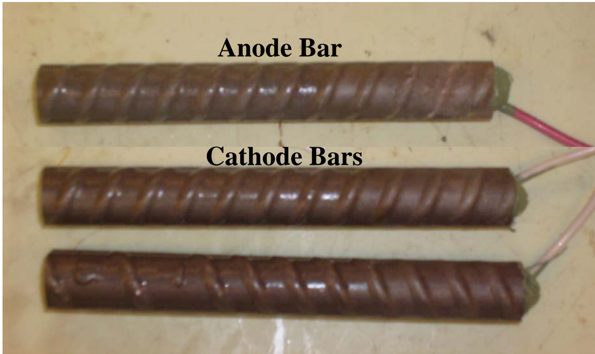
Figure A.10a: Specimen 5, Side B, immediately after removal from solution.
