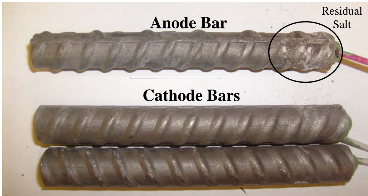
Figure A.7b: Specimen 4, Side A, eight days after removal from solution.
