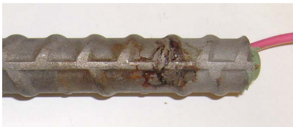
Figure 9: Specimen 4 one week after removal from solution, after brushing. A clear corrosion initiation site is evident, caused by crevice corrosion.
