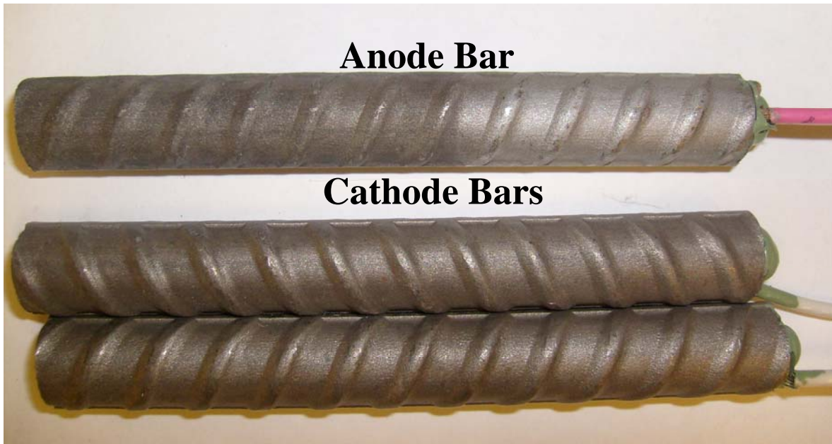
Figure A.6c: Specimen 3, Side B, eight days after removal from solution, after brushing.
