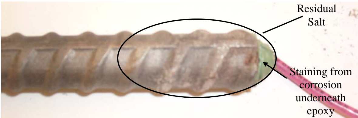
Figure A.10b: Specimen 5 anode, eight days after removal from solution, prior to brushing.
