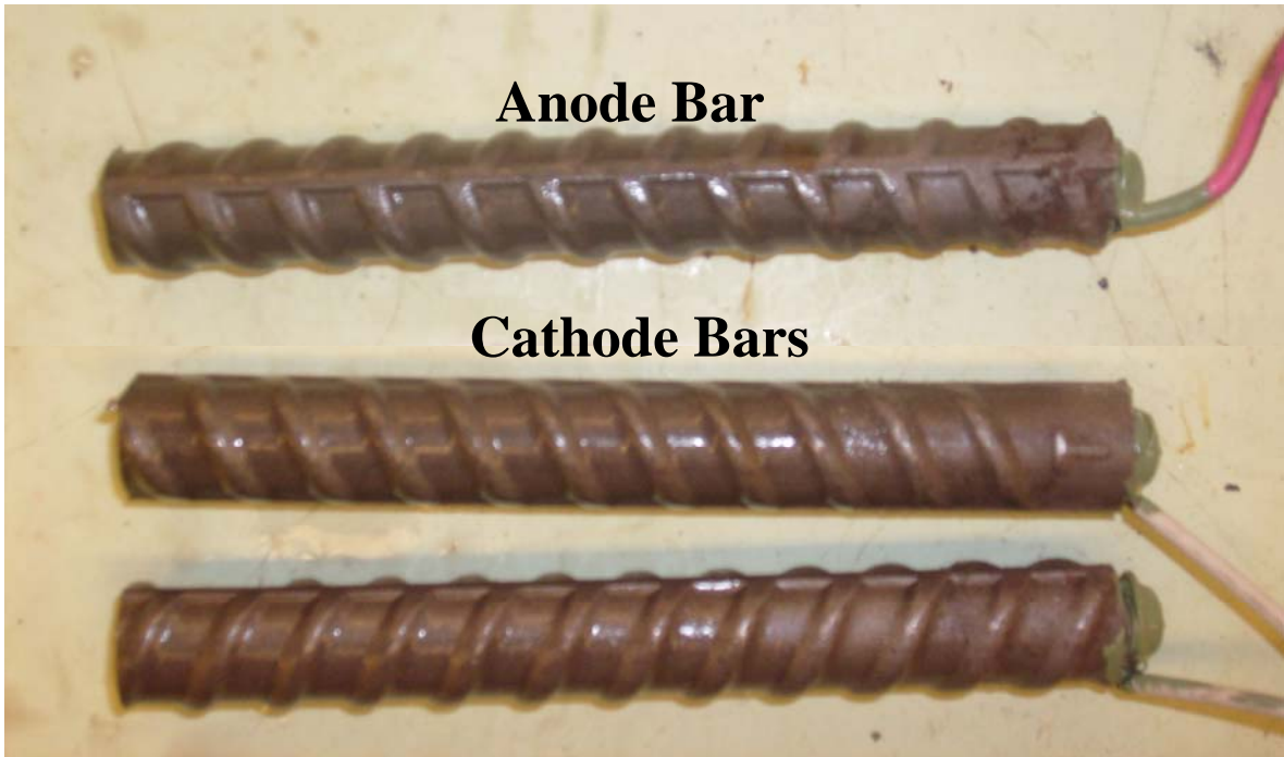
Figure A.12a: Specimen 6, Side B, immediately after removal from solution.
