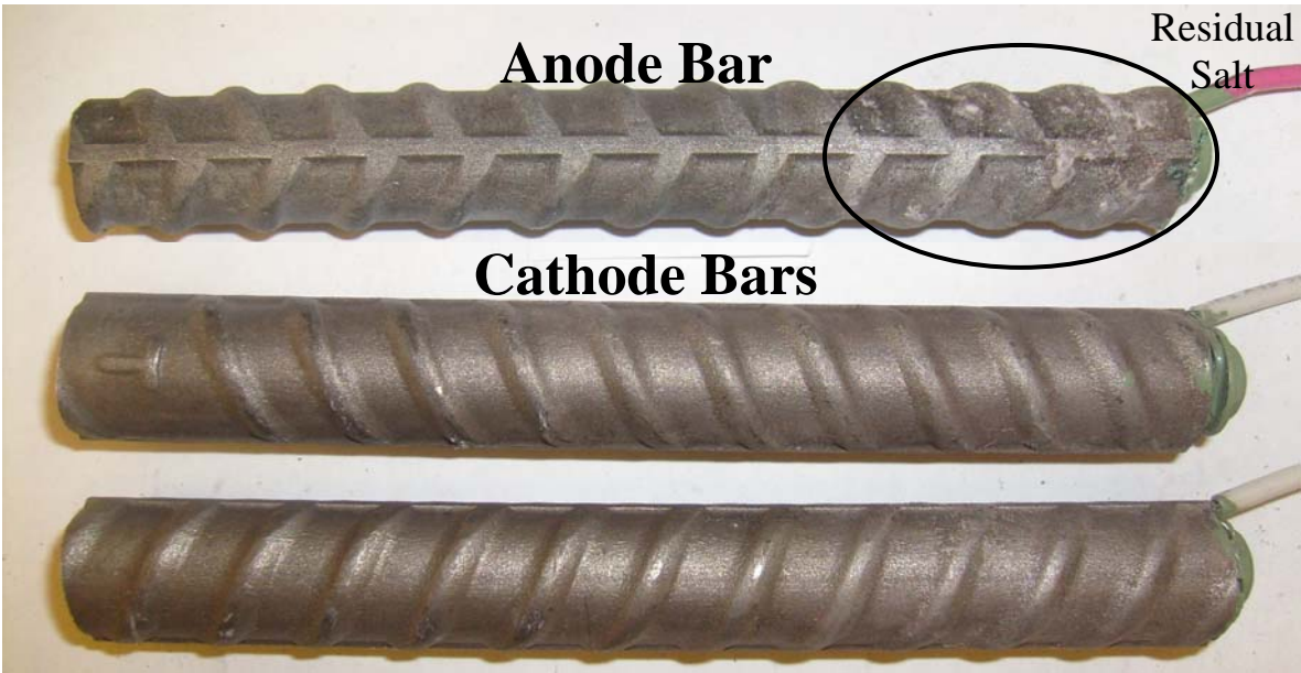
Figure A.11b: Specimen 6, Side A, eight days after removal from solution.
