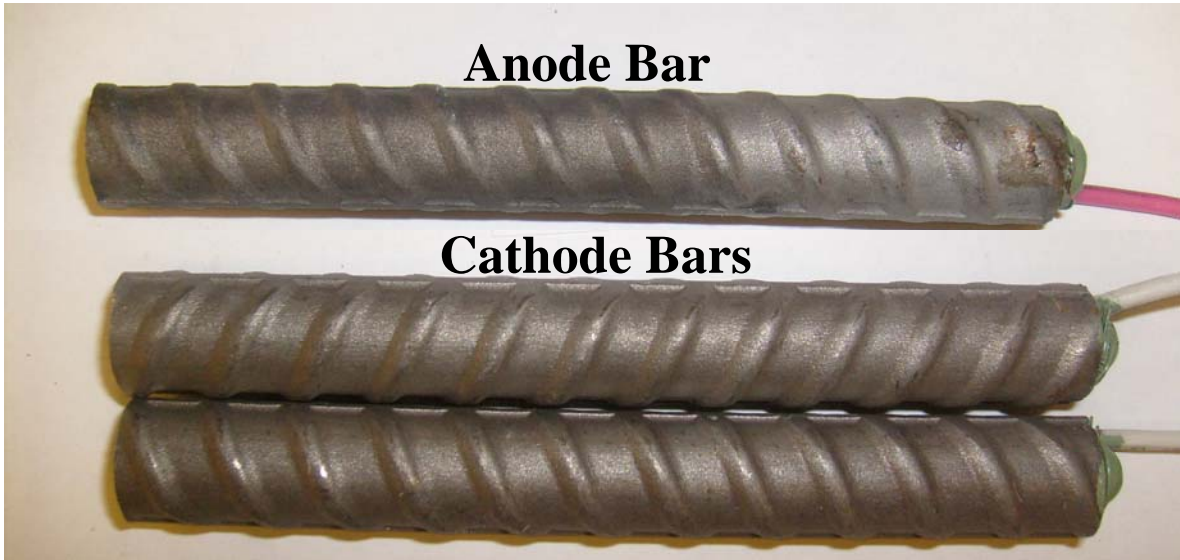
Figure A.5c: Specimen 3, Side A, eight days after removal from solution, after brushing. Much of the corrosion residue is removed with brushing.
