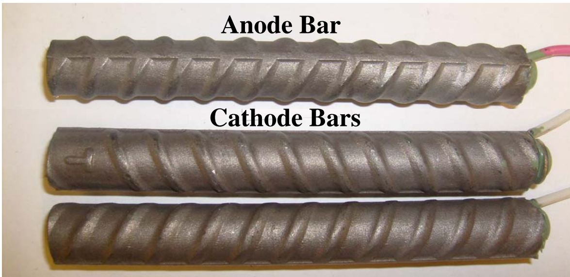
Figure A.11c: Specimen 6, Side A, eight days after removal from solution, after brushing.
