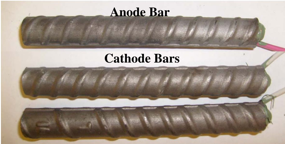
Figure A.10e: Specimen 5, Side B, eight days after removal from solution, after brushing.
