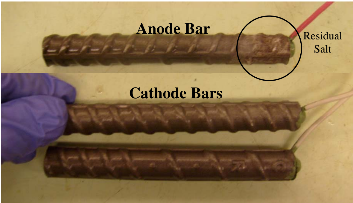
Figure A.3a: Specimen 2, Side A, immediately after removal from solution.
