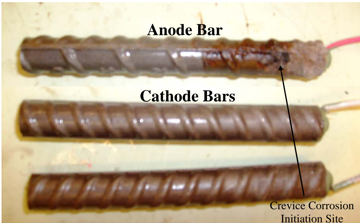
Figure A.8a: Specimen 4, Side B, immediately after removal from solution. Crevice corrosion caused by test configuration; it does not reflect on the corrosion resistance of the steel
