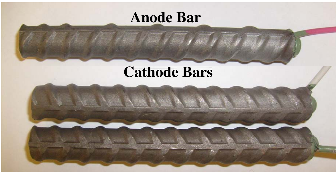
Figure A.2c: Specimen 1, Side B, eight days after removal from solution, after brushing.
