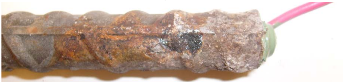
Figure A.8c: Specimen 4 anode bar, eight days after removal from solution.
