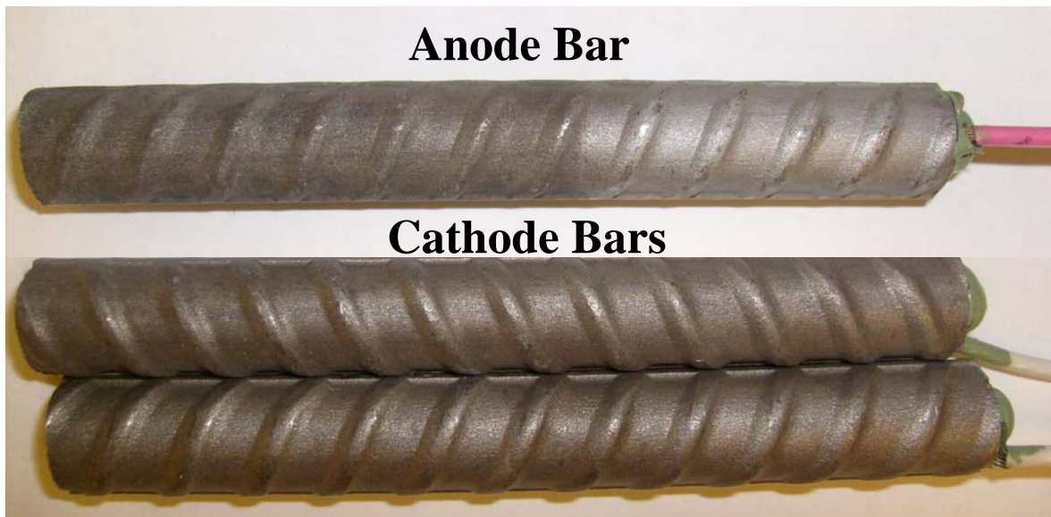
Figure 7: Specimen 3 one week after removal from solution, after brushing. Anode bar exhibits discoloration below the liquid level
