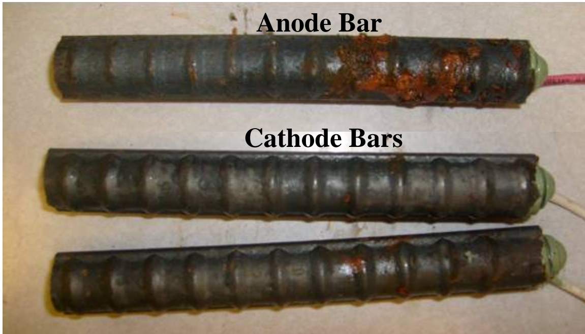
Figure 20: Conventional steel. Specimen 3, side A one week after removal from solution, after rinsing. Specimen exhibits significant corrosion above the liquid level.
