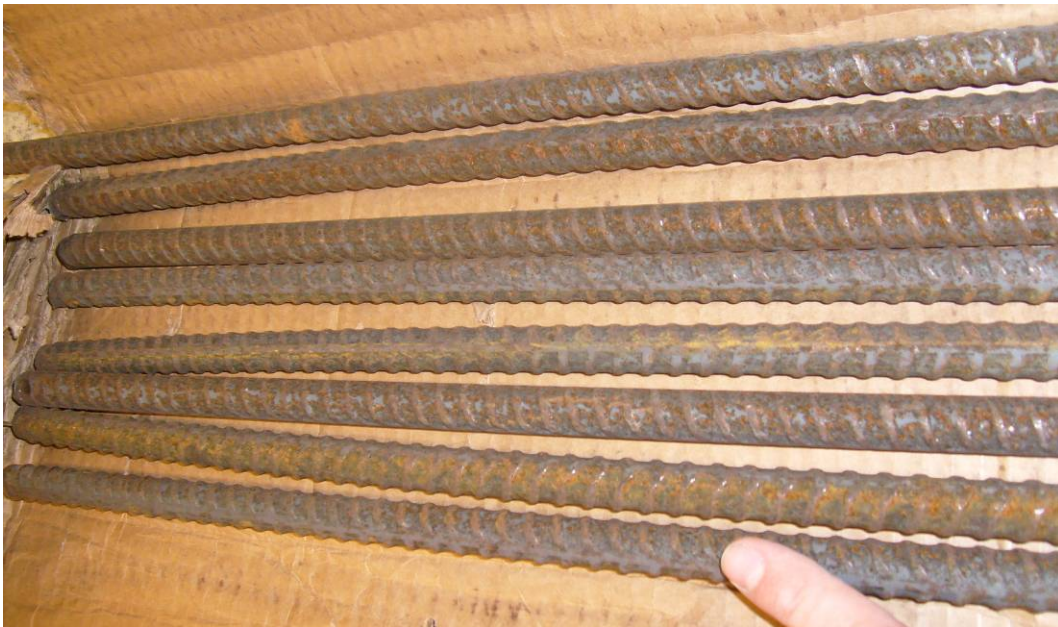
Figure 1: A1035 steel in the as-received condition exhibit corrosion on the surface of the bars.
