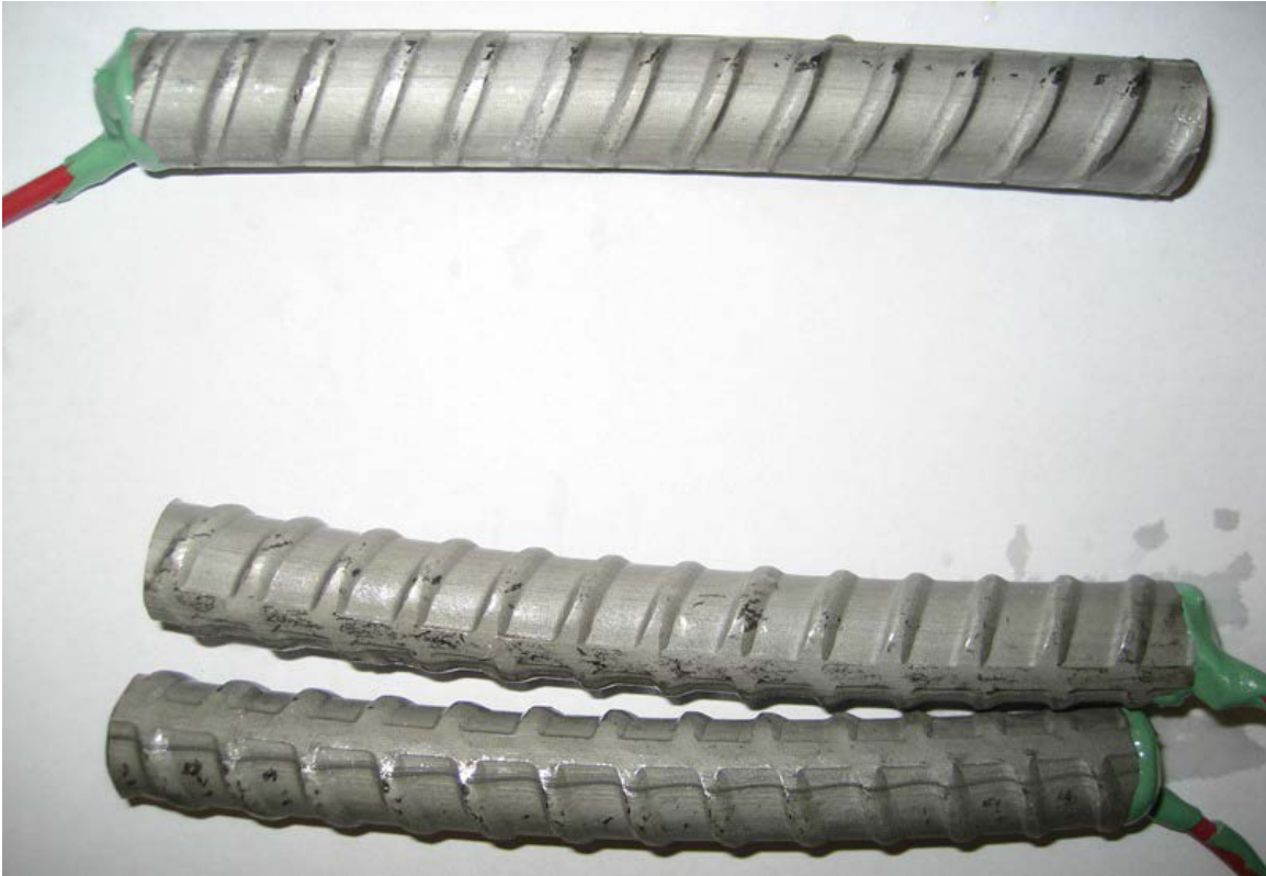
Figure 7: Coiled 2304 stainless steel after testing. Anode (top bar) and cathode (bottom bars).
