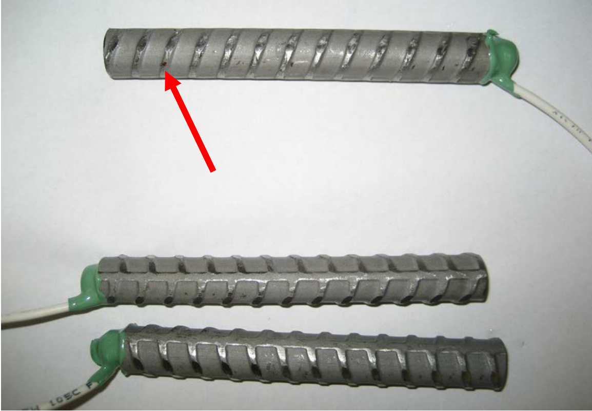
Figure 9a: Straightened 2304 stainless steel after testing. Anode (top bar) and cathode (bottom bars). Corrosion products indicated with arrow.
