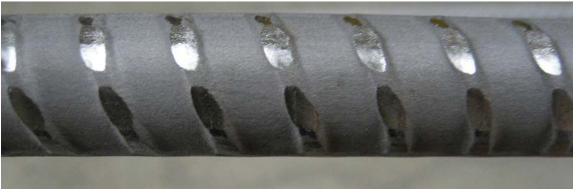
Figure 1: Damage to deformations from straightening process.
