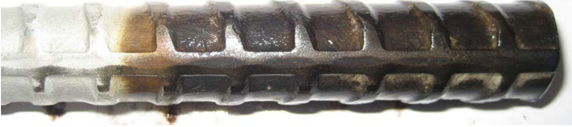
Figure 16b: Straightened XM-28 stainless steel from producer A after testing; specimen XM28s-5. Anode bar with severe discoloration.
