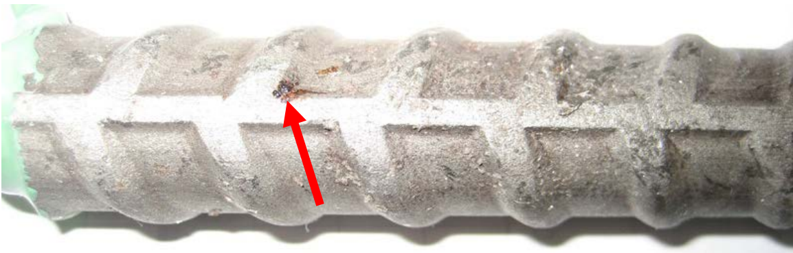
Figure 19b: 2205 stainless steel from producer B showing closeup of corrosion products (arrow) after testing; specimen 2205-1.
