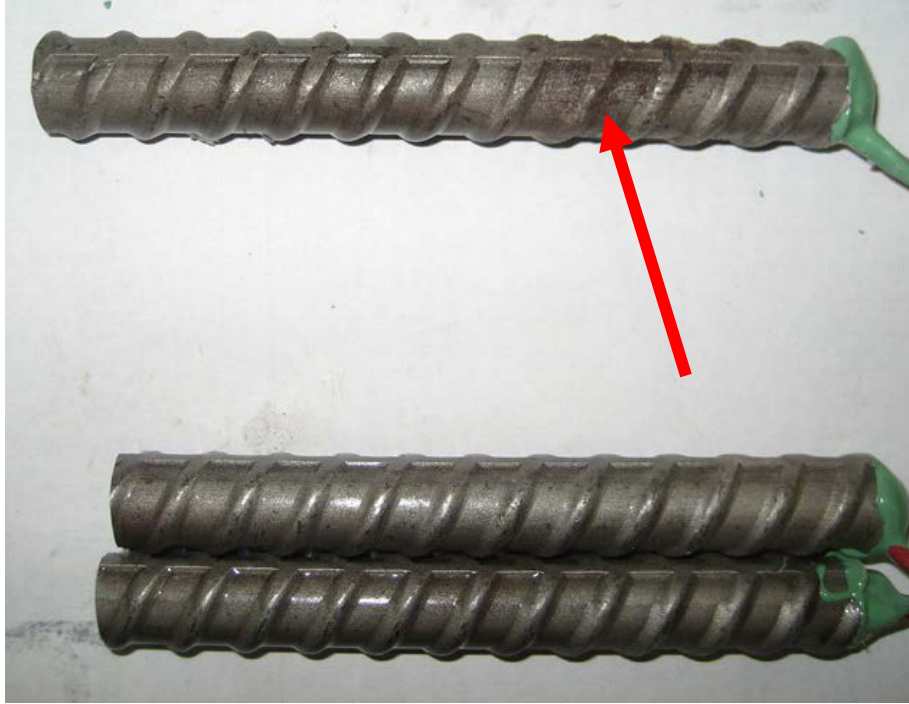
Figure 20a: 2205 stainless steel from producer B showing discoloration and corrosion products (arrow) after testing; specimen 2205-3. Anode (top bar) and cathode (bottom bars).
