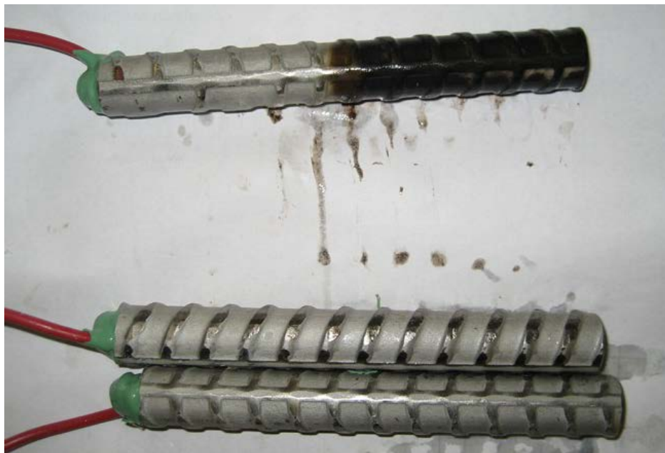
Figure 16a: Straightened XM-28 stainless steel from producer A after testing; specimen XM28s-5. Anode (top bar) and cathode (bottom bars).
