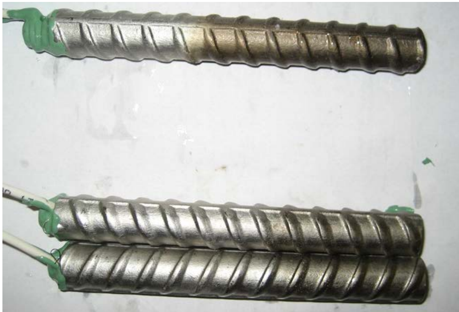
Figure 17: XM-28 stainless steel from producer B showing moderate discoloration after testing; specimen XM28-5. Anode (top bar) and cathode (bottom bars).
