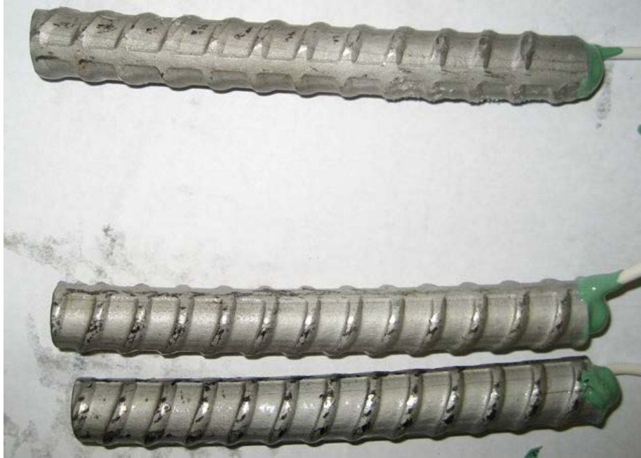
Figure 13: Coiled XM-28 stainless steel from producer A after testing; specimen XM28c-2. Anode (top bar) and cathode (bottom bars).
