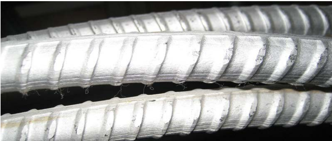
Figure 1b: Damage to deformations on coiled XM-28 bars.
