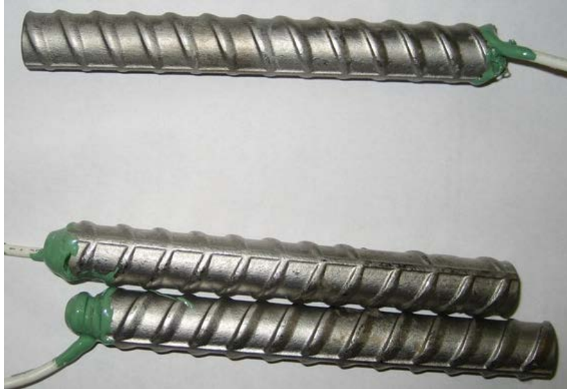
Figure 18: XM-28 stainless steel from producer B showing mild discoloration after testing; specimen XM28-1. Anode (top bar) and cathode (bottom bars).
