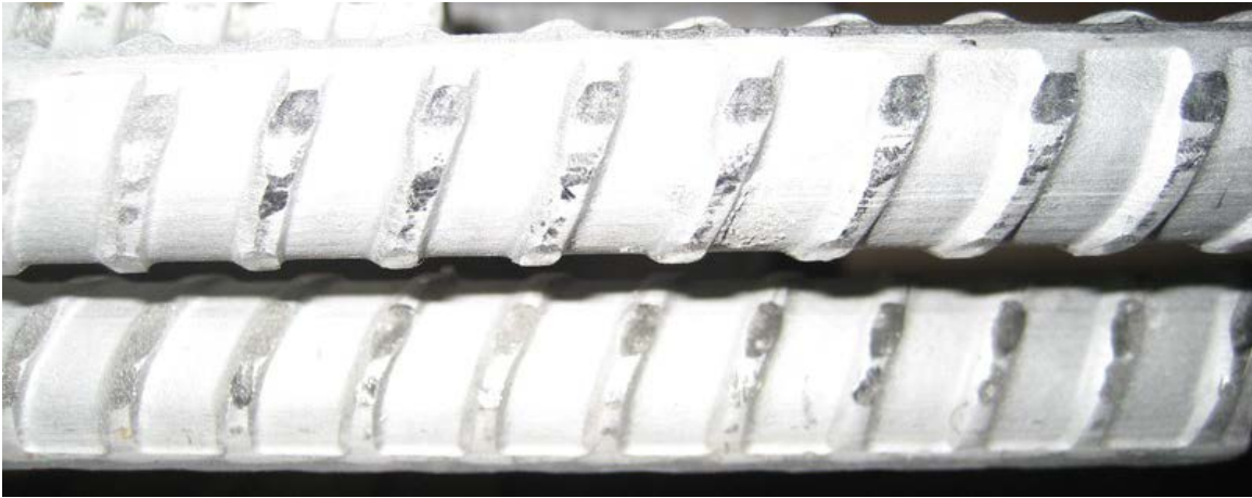
Figure 1a: Damage to deformations on straightened XM-28 bars from the straightening process.
