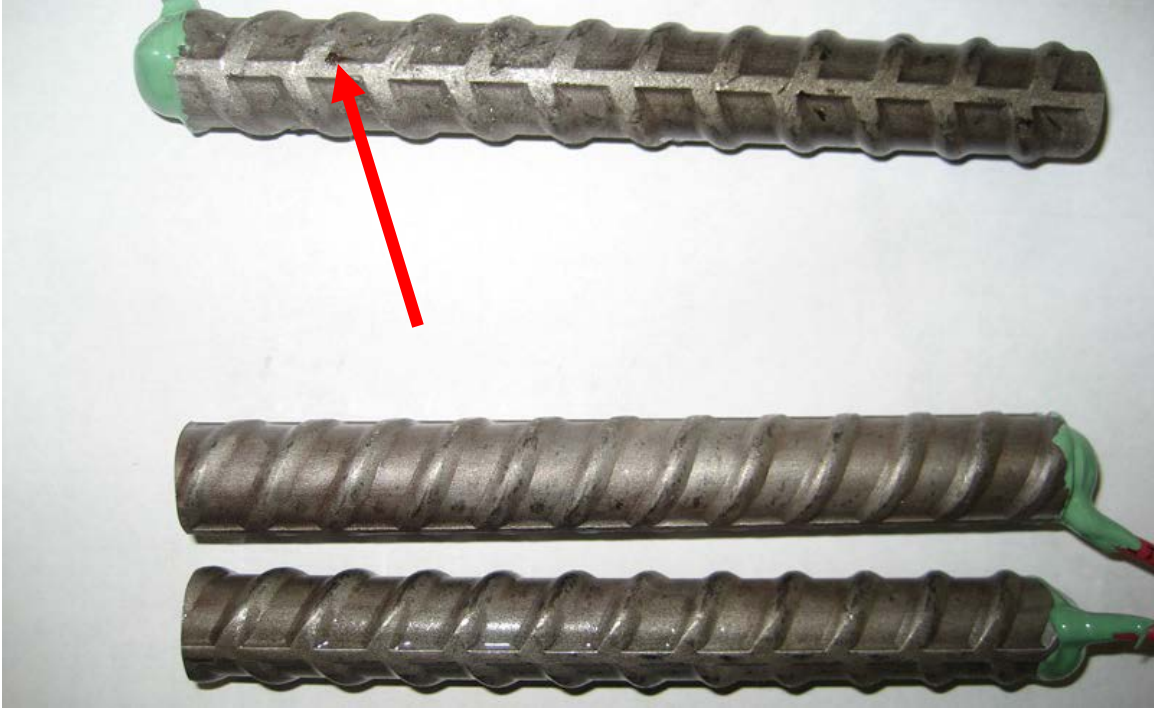
Figure 19a: 2205 stainless steel from producer B showing discoloration and corrosion products (arrow) after testing; specimen 2205-1. Anode (top bar) and cathode (bottom bars).
