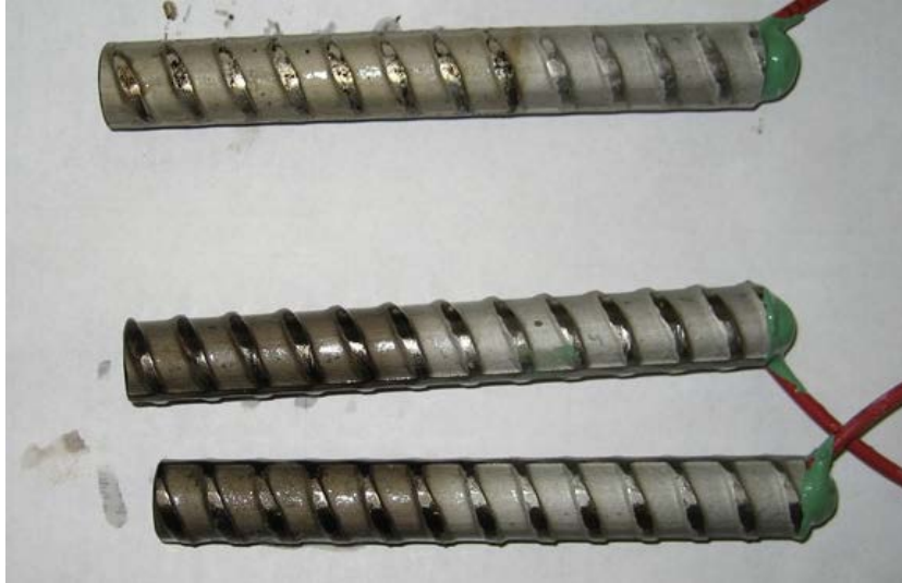
Figure 15: Straightened XM-28 stainless steel from producer A after testing; specimen XM28s-1. Anode (top bar) and cathode (bottom bars).
