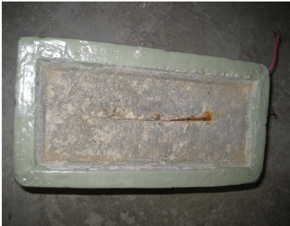
Figure 93a: Staining in the crack of cracked beam specimen 5 containing 2304 stainless steel
