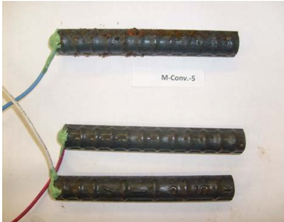
Figure 38: Rapid macrocell specimen upon completion of test, conventional steel (anode on top, cathode on bottom)
