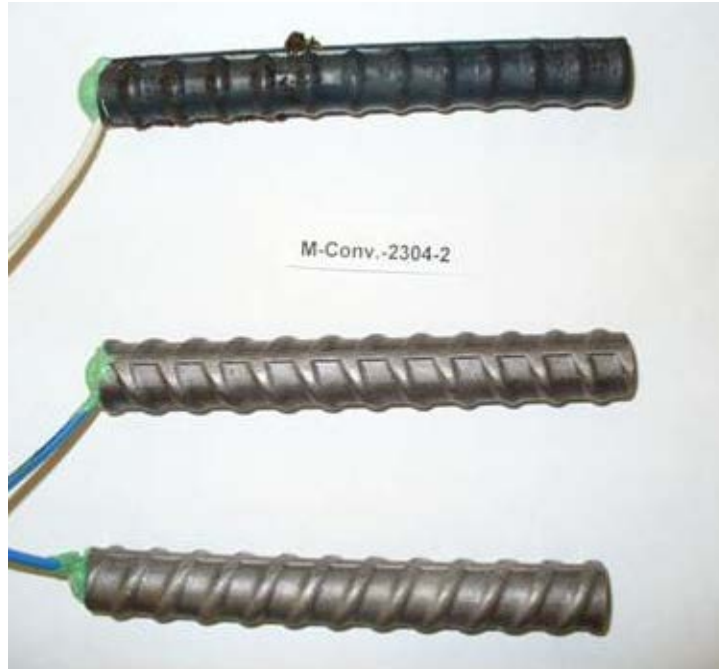
Figure 44: Rapid macrocell specimen upon completion of test, mixed conventional/2304 stainless steel (anode on top, cathode on bottom)
