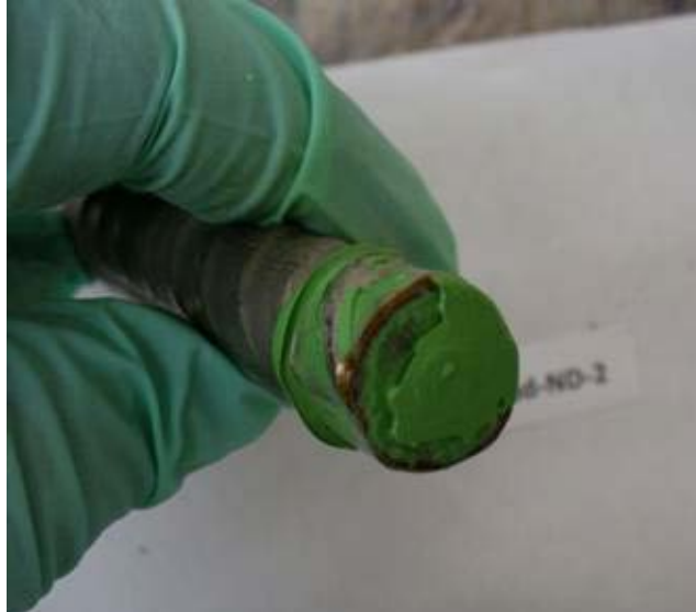
Figure 46: Rapid macrocell specimen upon completion of test, undamaged stainless steel clad reinforcement (close-up of bar end after cap has been removed)
