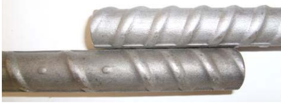
Figure 1: 2304 duplex stainless steel bars in the as-received (left) and repickled (right) conditions
