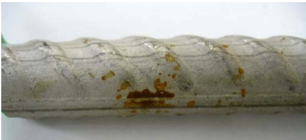
Figure 28b: Photograph of specimen 6 upon completion of the rapid evaluation test, NX-SCR™ stainless steel clad (close-up of cathode)
