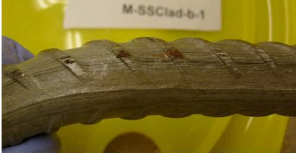
Figure 32: Corrosion staining on bent section upon autopsy, bent NX-SCR™ stainless steel clad bar (close-up)
