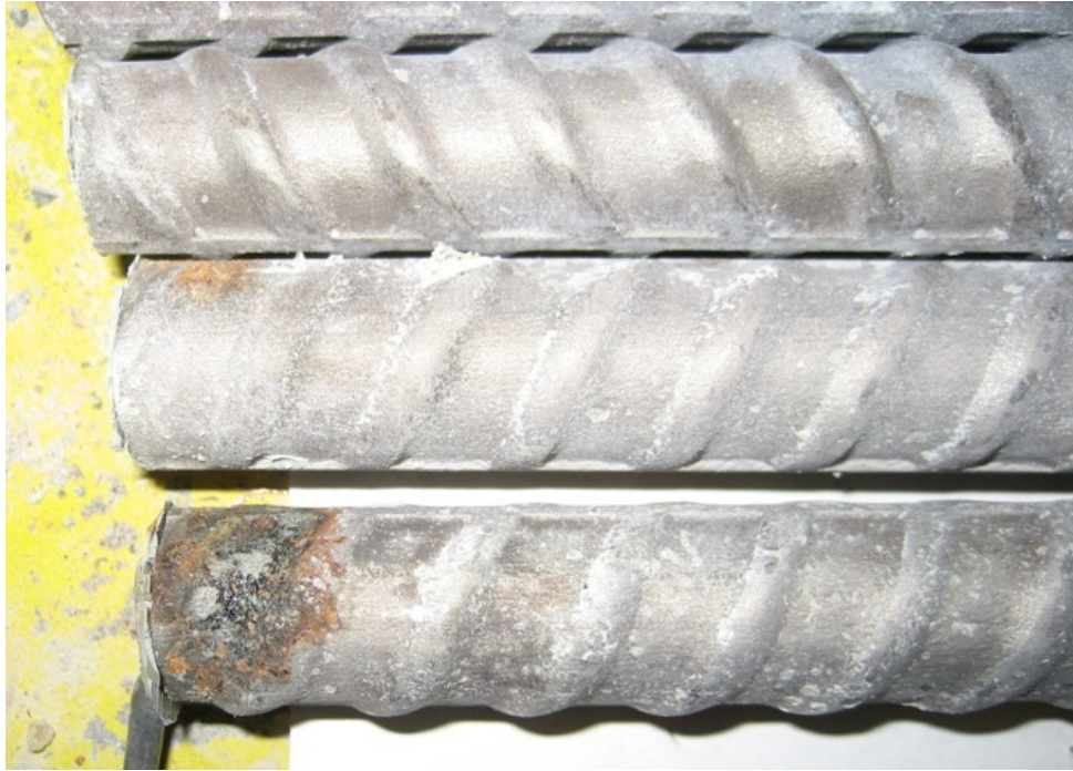
Figure 72: Cathode of 2304 stainless steel, mixed conventional/2304 steel Southern Exposure specimen 1 after autopsy
