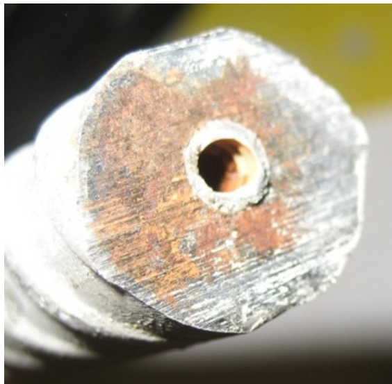
Figure 77b: Corrosion at the end of specimen CB-SSClad-1 upon completion of test
