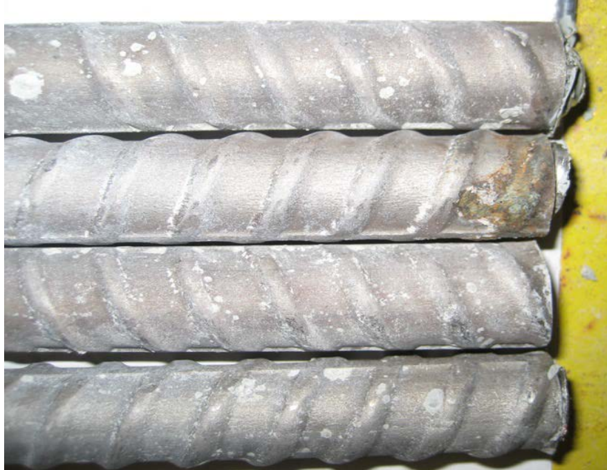
Figure 65b: Bottom bars of specimen SE-2304-2 after autopsy showing signs of corrosion near the end of the bar
