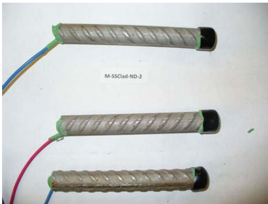
Figure 45: Rapid macrocell specimen upon completion of test, undamaged stainless steel clad reinforcement (anode on top, cathode on bottom)
