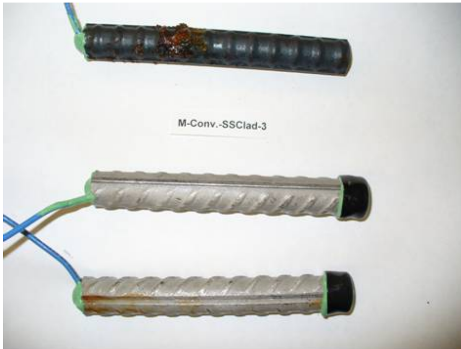
Figure 51: Rapid macrocell specimen upon completion of test, mixed conventional/stainless steel clad reinforcement (anode on top, cathode on bottom)
