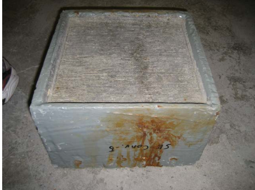
Figure 86a: Staining on outside of Southern Exposure specimen 5 with conventional steel in the top mat
