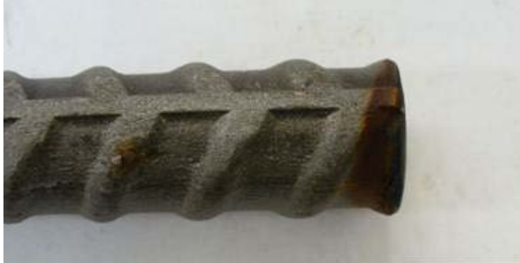
Figure 23: Staining of anode of 2304 stainless steel, mixed 2304/conventional steel macrocell specimen
