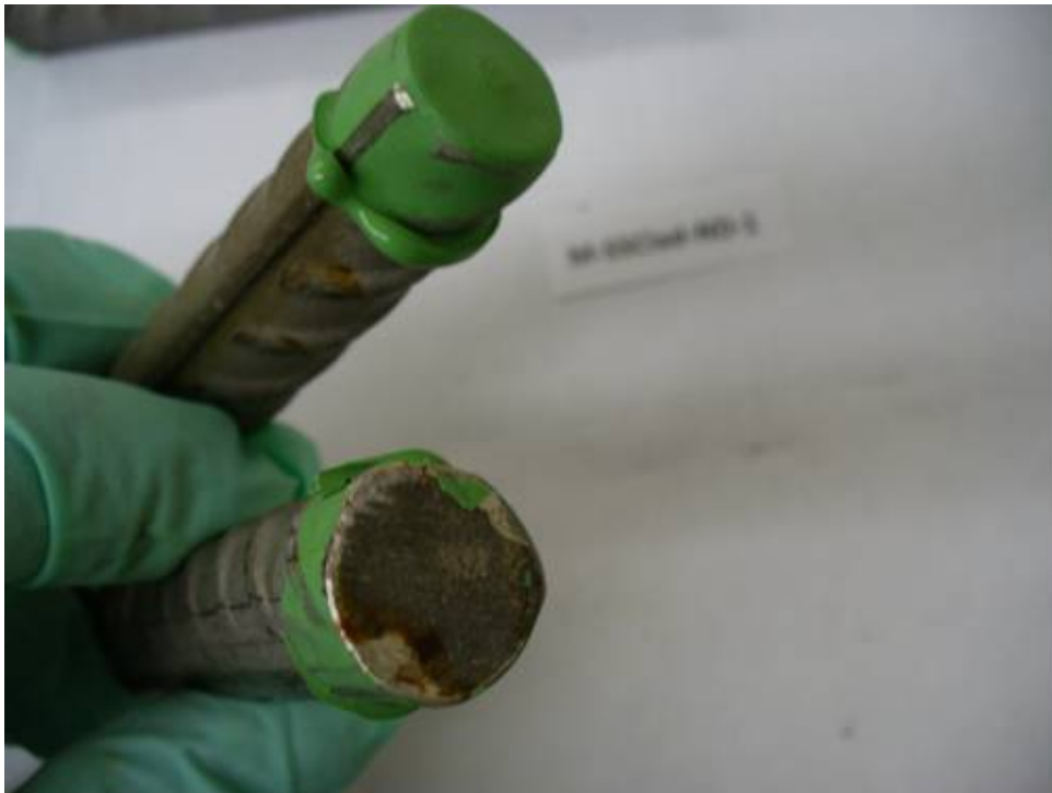
Figure 27: Bar end with protective cap removed at end of rapid macrocell test, NX-SCR™ stainless steel clad (cathodes)
