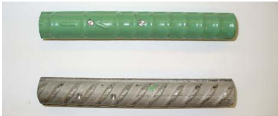
Figure 2: Rapid macrocell specimens, ECR and NX-SCR™ stainless steel clad bars with holes in the coating (0.83% exposed area)
