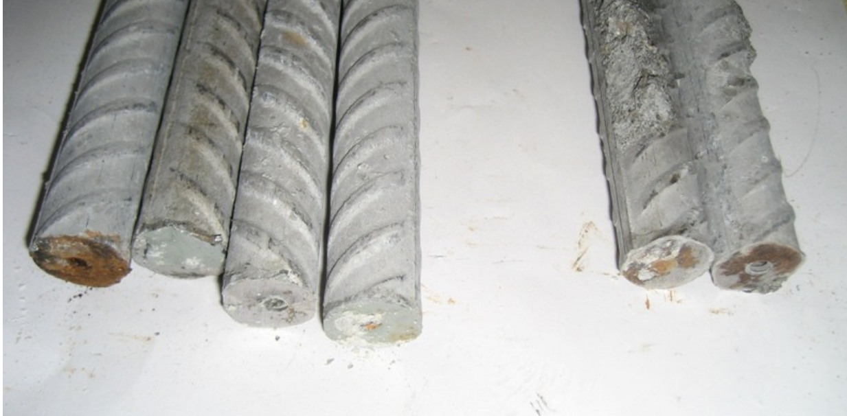
Figure 98b: Bars from Southern Exposure specimen 4 containing undamaged stainless steel clad reinforcement after autopsy, showing corrosion at ends of top and bottom bars (close up)
