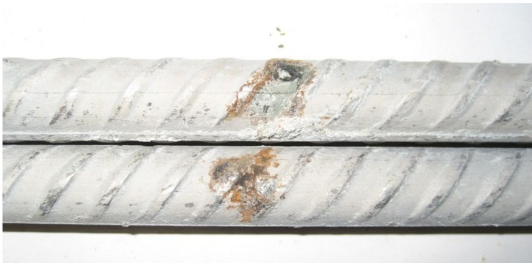
Figure 97b: Top Bars from Southern Exposure specimen 5 containing stainless steel clad reinforcement with holes through the cladding after autopsy, showing corrosion at damage site on top bars (close up)
