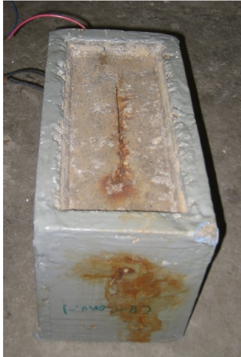
Figure 87a: Staining of cracked beam specimen 1 containing conventional reinforcement
