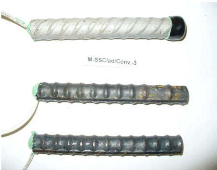
Figure 52: Rapid macrocell specimen upon completion of test, mixed stainless steel clad/conventional steel (anode on top, cathode on bottom)
