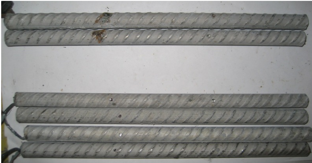
Figure 97a: Bars from Southern Exposure specimen 5 containing stainless steel clad reinforcement with four holes through the cladding after autopsy
