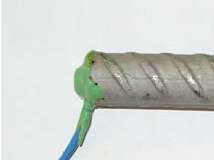
Figure 28c: Photograph of specimen 6 upon completion of the rapid evaluation test, NX-SCR™ stainless steel clad showing corrosion at electrical connection
