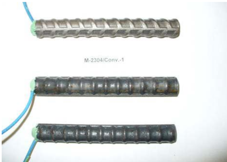
Figure 43: Rapid macrocell specimen upon completion of test, mixed 2304/conventional steel (anode on top, cathode on bottom)
