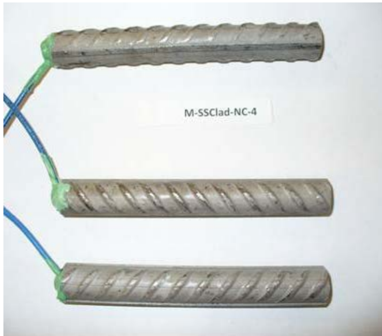
Figure 48: Rapid macrocell specimen upon completion of test, uncapped stainless steel clad reinforcement (anode on top, cathode on bottom)
