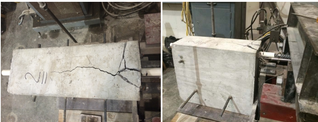
Figure 6 – Specimen No. 2 after failure.
