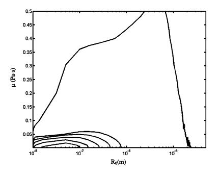
FIG. 4. Contour plot of bubble growth rates at 3 MPa, 1 MHz, and dissolved gas concentration 100%. Solid lines correspond to growth rates of, from top to bottom, 0, 1, 10, 100, 1000, and 10 000 m/s.
