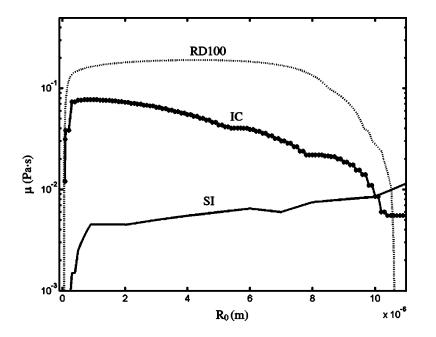
FIG. 1.  $P_a = 1.0$  MPa, f = 1 MHz, and 100% gas saturation. Rectified diffusion (RD100, dashed line), shape instability (SI, thin solid line), and inertial cavitation (IC, thick solid line with stars) thresholds. Below RD bubbles grow. Below IC bubbles collapse inertially. Below SI bubbles break up from shape instabilities.
