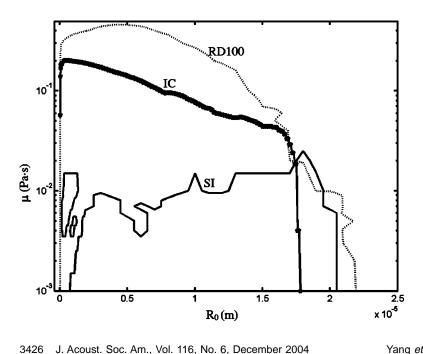
FIG. 2.  $P_a = 2.5$  MPa, f = 1 MHz, and 100% gas saturation. Rectified diffusion (RD100, dashed line), shape instability (SI, thin solid line), and inertial cavitation (IC, thick solid line with stars) thresholds at  $P_a = 1$  MPa, f = 1 MHz. Below RD bubbles grow. Below IC bubbles collapse inertially. Below and enclosed by SI bubbles break up from shape instabilities.
