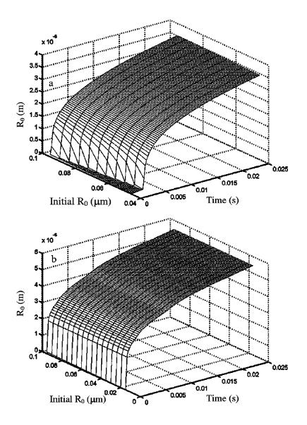
FIG. 5. Bubble equilibrium radius vs time for bubbles with initial radii ranging from 15 nm to 95 nm at 2 MPa for different viscosities: (a) 0.05 Pa s and (b) 0.005 Pa s. Dissolved gas concentration 20%.
