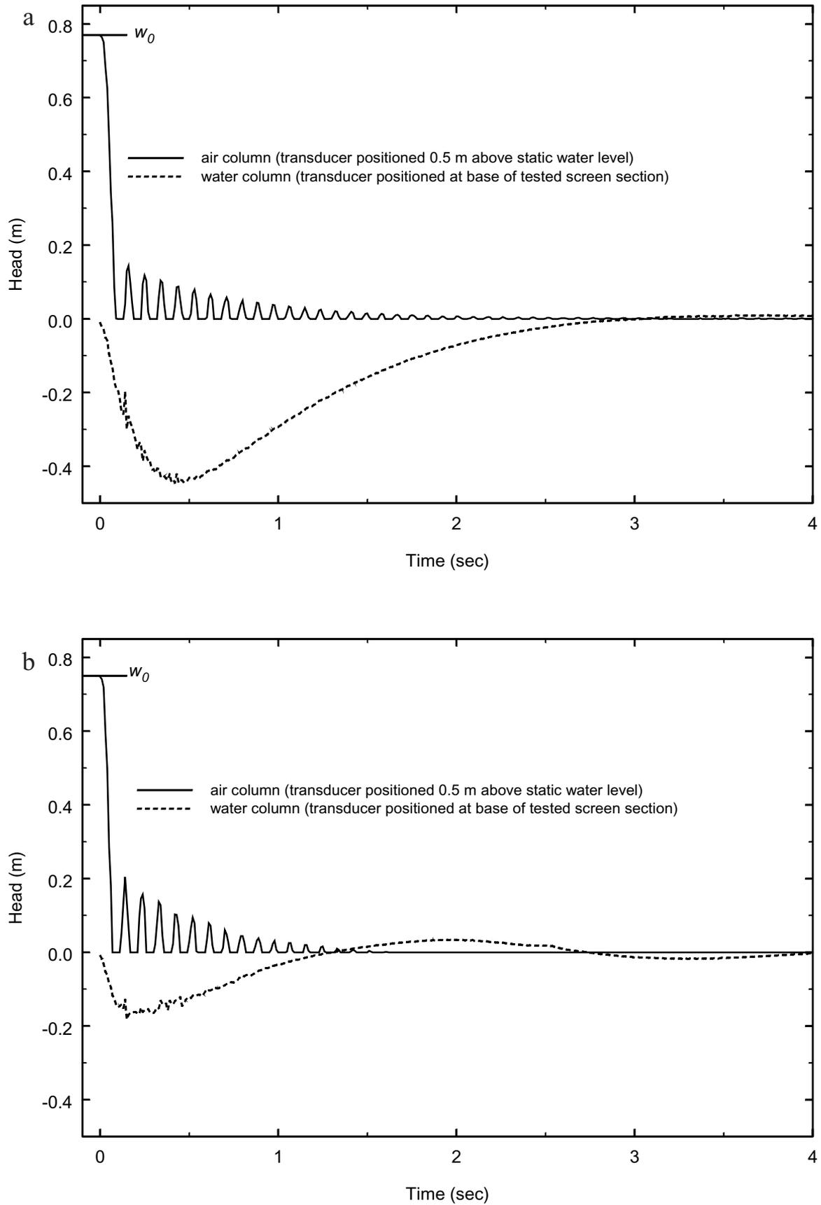
**Figure A1.** Pressure head responses in the water column and in the air column during an MLST ( $w_0 = 0.7$  m) performed in well 15 at the Horkheimer Insel, Germany, field site. (a) Monotonic response from depth of 8.3 m. (b) Oscillatory response from depth of 7.7 m. MLST geometry is  $l_s = 0.65$  m,  $l_p = 0.63$  m, and  $l_r \approx 1.3$  and 1.9 m for Figures A1a and A1b, respectively, with  $r_s = 7.6$  cm,  $r_p = 1.9$  cm, and  $r_r = 2.5$  cm.
