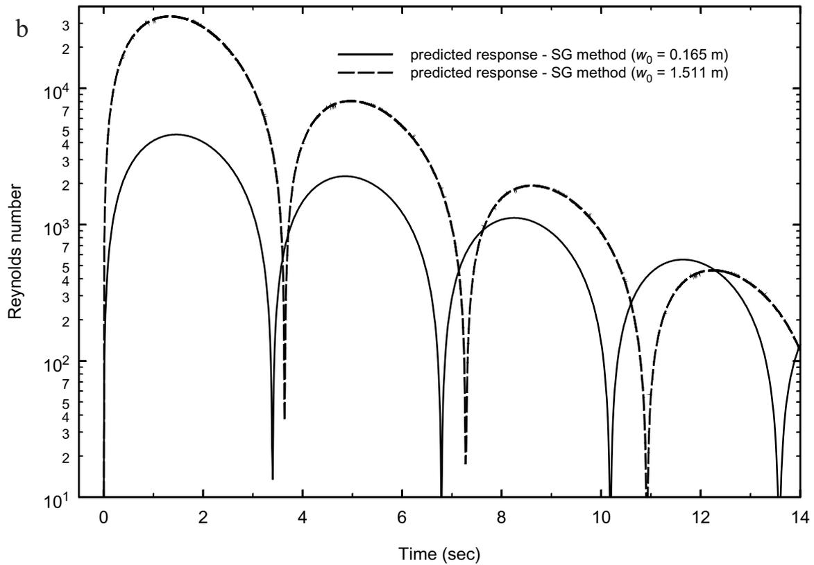
**Figure 5.** (a) Example results of individual optimization for subset of tests of Figure 3 using the dynamic interpretation of transducer-measured head. (b) Reynolds number for predicted responses from the Springer-Gelhar (SG) method.
