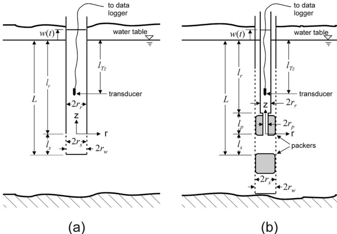
**Figure 1.** Schematic of (a) slug test performed in partially penetrating well and (b) multilevel slug test. Although not shown, depth to transducer positioned within the screened interval between packers is designated as  $l_{Tz}$ .
