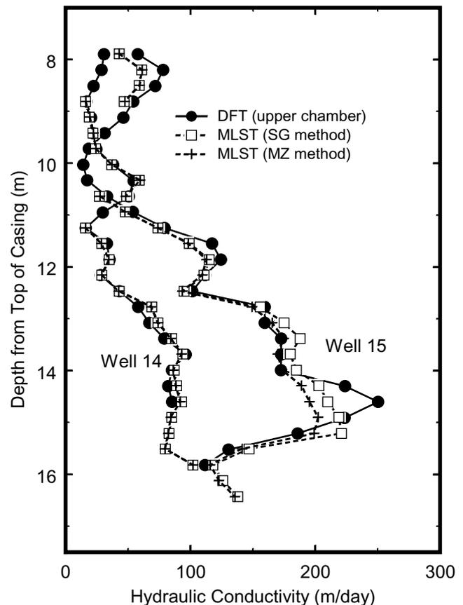
**Figure 9.**  $K_r$  profiles from the dipole-flow test and MLST for wells 14 and 15.
