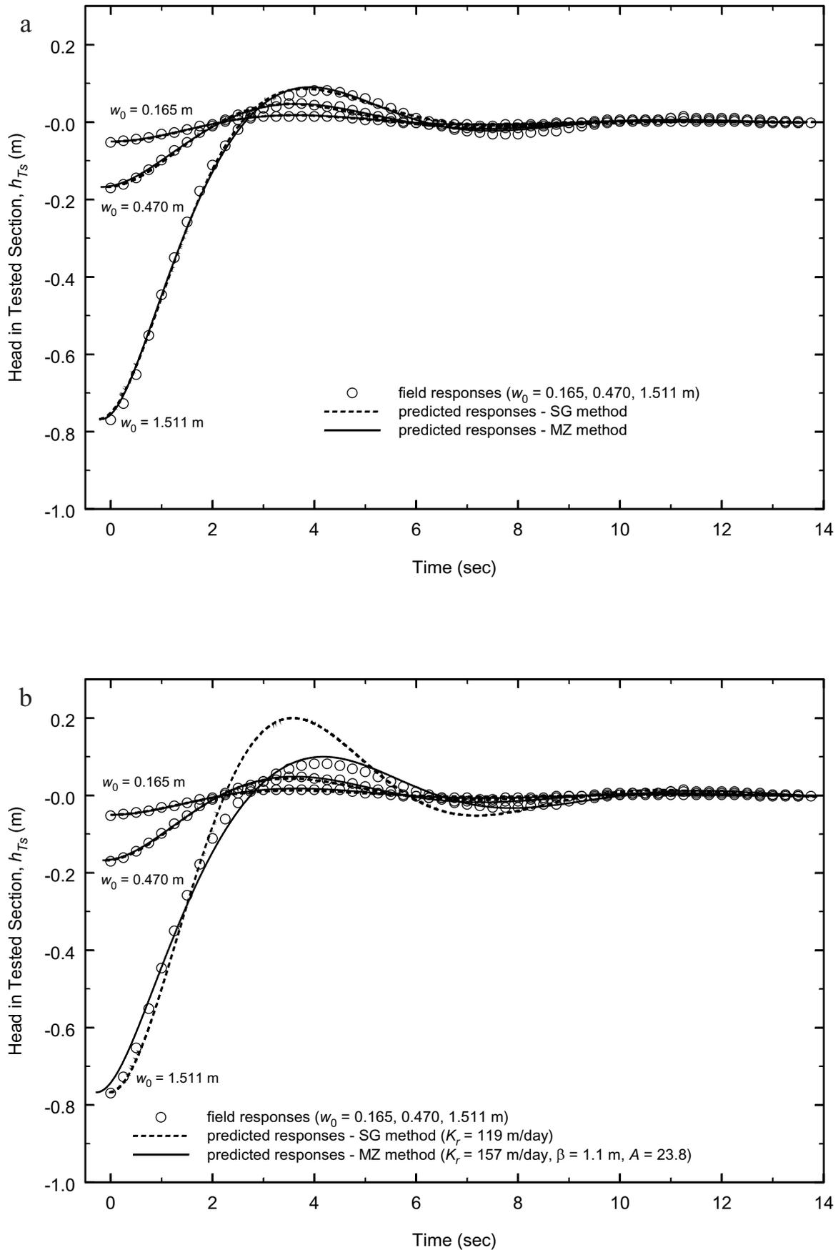
**Figure 8.** Example optimization results for subset of tests of Figure 3 using “translated” head response and the hydrostatic interpretation of transducer-measured head with (a) individual optimization and (b) group optimization.
