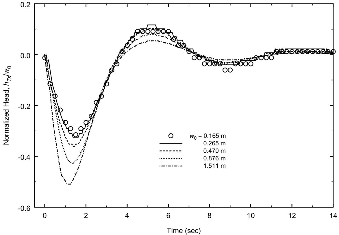
**Figure 3.** Normalized head responses obtained in well 15 (depth of tested interval 14.3 m) using various initial displacements. Pressure response for small  $w_0$  (0.165 and 0.265 m) illustrate approximately linear behavior. MLST specifications are the same as in Figure 2b with the exceptions  $l_{T_s} = 10.9$  m,  $l_s = 0.62$  m, and  $l_r = 9.65$  m. Note that symbols are displayed at 1/4 of the field-recorded frequency.
