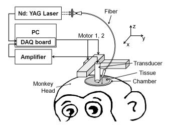
Fig. 1 Schematic of the PA system.
