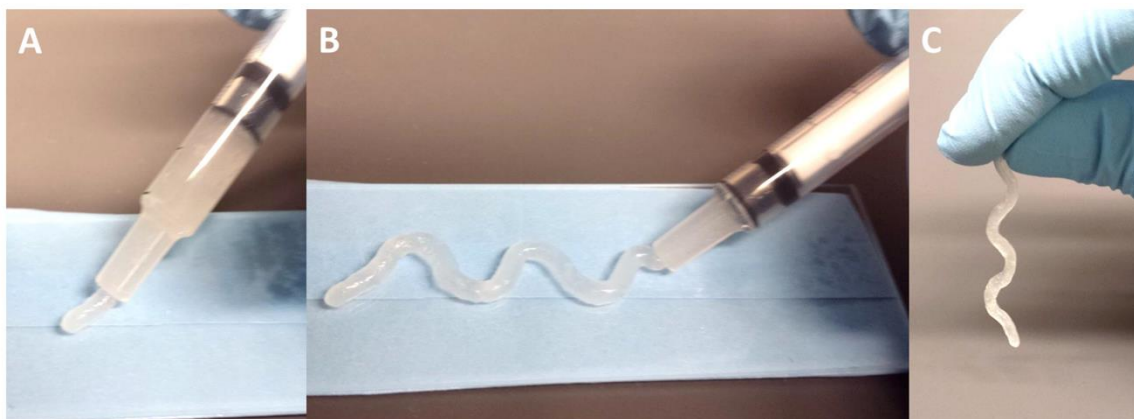
Figure 3.4: Hyaluronic Acid Nanoparticle (HANp)-Incorporated Solutions Maintain Shaping Before and After Crosslinking
