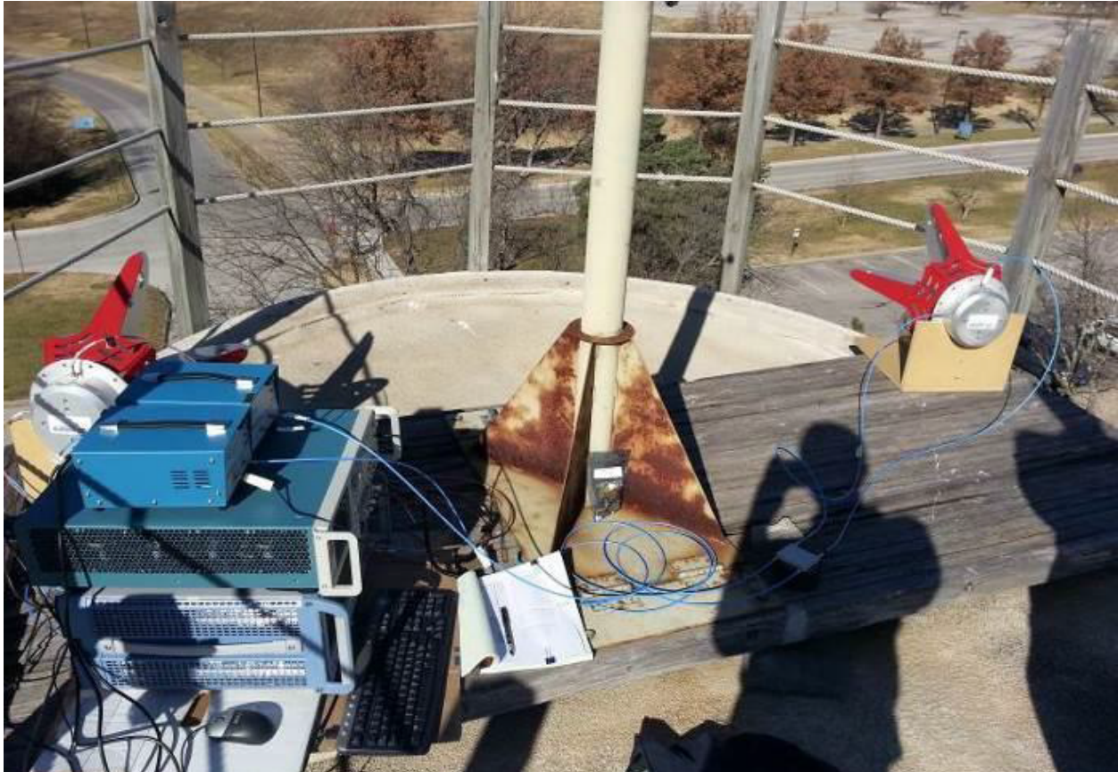
Figure 4.1: Equipment used to record measurements. The radar is quasi-monostatic, with the right antenna used to transmit and the left to receive. The antennas are roughly 15 meters from the ground and are directed at two large buildings on the University of Kansas campus.
