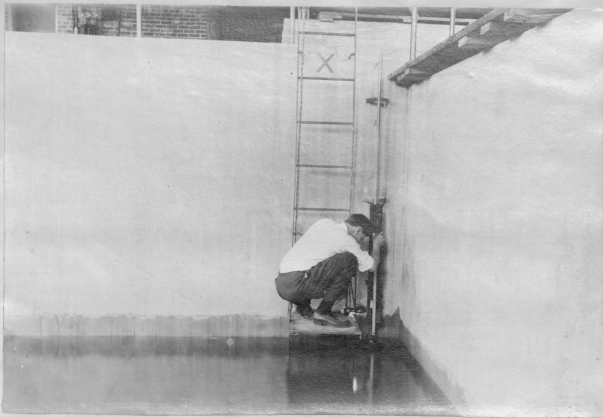
Figure 2 Observing water-level in calibrated tank.
