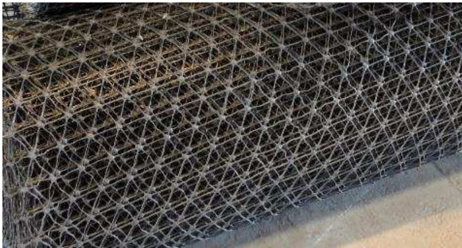
Figure 3.14 The geogrid used in this study
