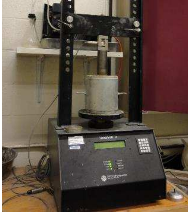
Figure 3.3 CBR test setup
