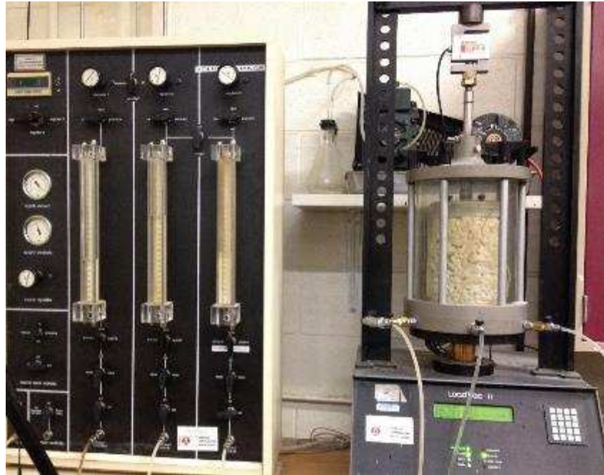
Figure 3.5 The triaxial test setup
