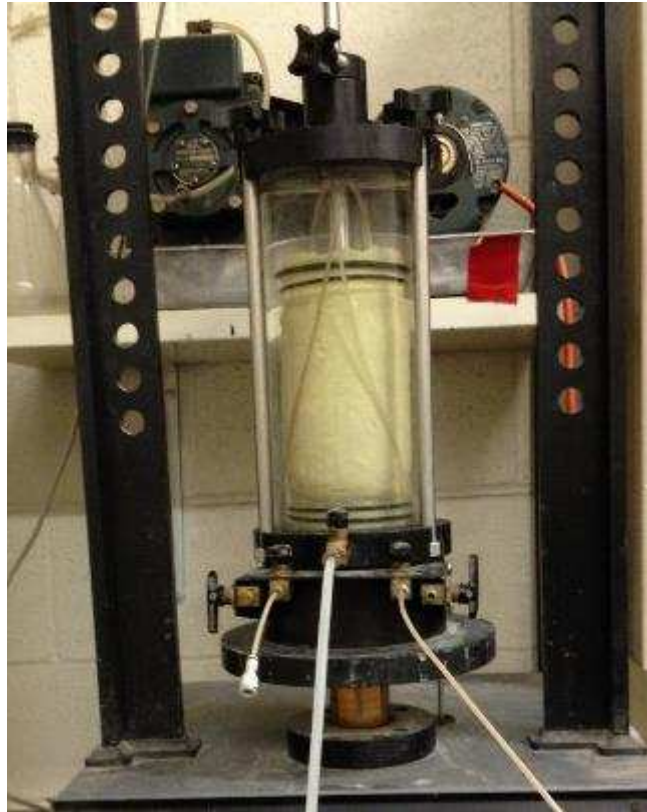
Figure 3.11 Triaxial test of the subgrade
