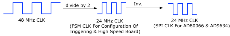
Fig. 4.17 Synthesis of registry configuration and data transfer clocks from the 48 MHz clock.
