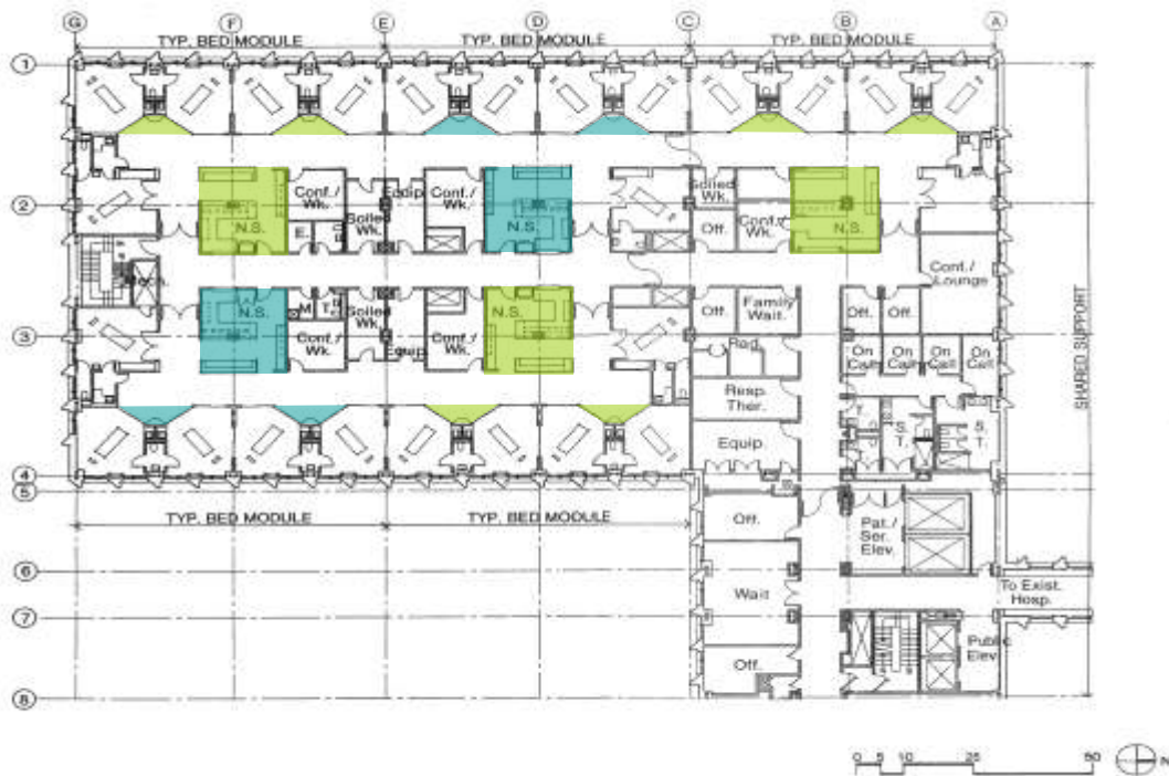
Figure 13: Nursing substations with observation units.
