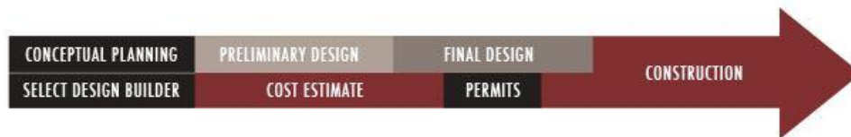
Figure 2.4: DB Project Delivery Framework (Makatura Inc., 2013)
