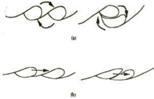
Figure 13: Vortex merging processes: (a) rotational pairing, and (b) slapping 54
