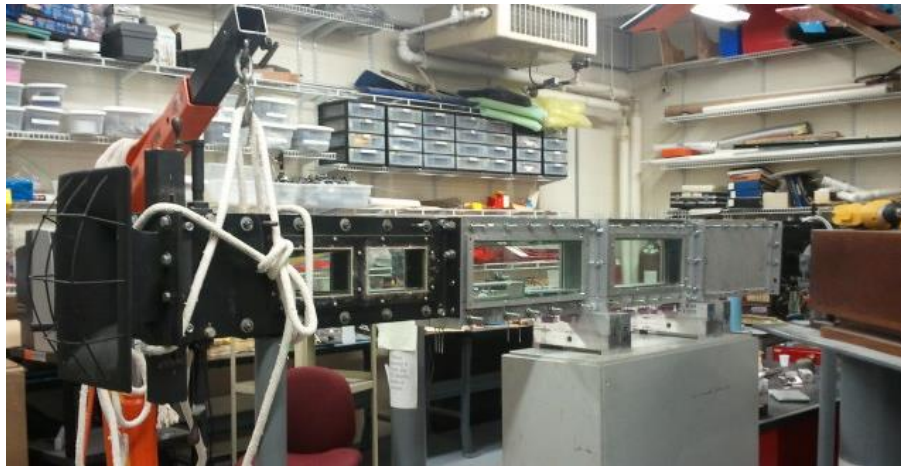
Figure 77: Completed Wind Tunnel with New Test Section
