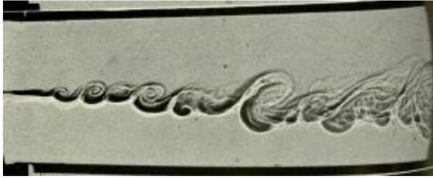
Figure 6: Brown and Roshko Shear Layer Shadowgraph Image 9
