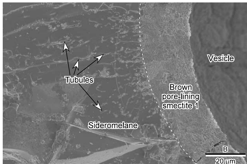
Figure 7. (a) Backscattered-electron image of reddened smectitic grain replacement (RSGR) and pore-lining smectite from 1426 mbsl. Within the zone of smectite alteration, a sideromelane shard has been coated with smectite and partially replaced by reddened smectitic grain replacement. An early fracture running from the upper lower left to the lower right of the BSE micrograph has been filled with smectite containing abundant apatite inclusions. The smectitic grain replacements contains abundant inclusions of spherulitic, titaniferous nodules (<10 μm in diameter). A mist zone (containing tubules that appear as black and gray dots) separates the smectitic grain replacement from sideromelane (containing plagioclase microlites). (b) Secondary electron micrograph of vesicle wall and tubules from 1478.5 mbsl. Vesicle contains pore-lining smectite.
